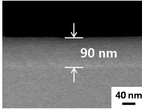
**Fig. S2** Cross-sectional SEM image of the  $\text{N}_2\text{O}$ -gas-based  $\text{SiO}_2$  film prepared by PECVD.
