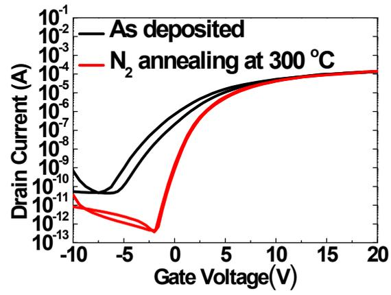
**Fig. S5** Hysteresis characteristics of IGZO TFTs with NO-based SiO<sub>2</sub> films as deposited and N<sub>2</sub> annealing.
