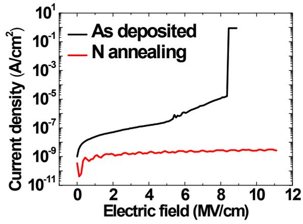
**Fig. S3** Dielectric breakdown of NO-based SiO<sub>2</sub> films before and after annealing.
