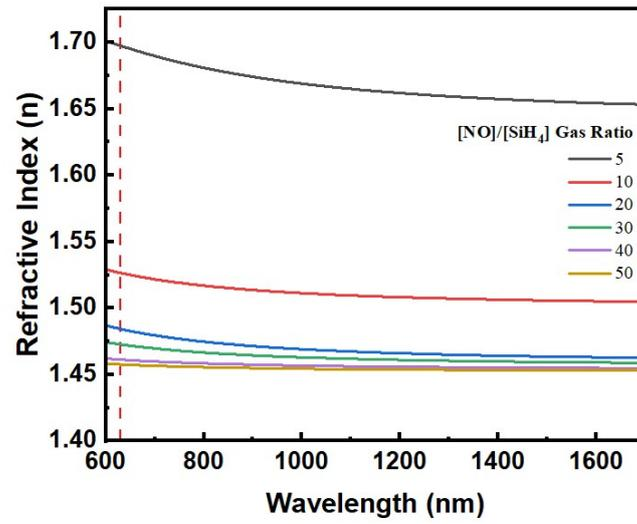
**Fig. S1** Refractive index of NO-based SiO<sub>2</sub> films for different [NO]/[SiH<sub>4</sub>] gas ratios in the wavelength range of 600 to 1700 nm.
