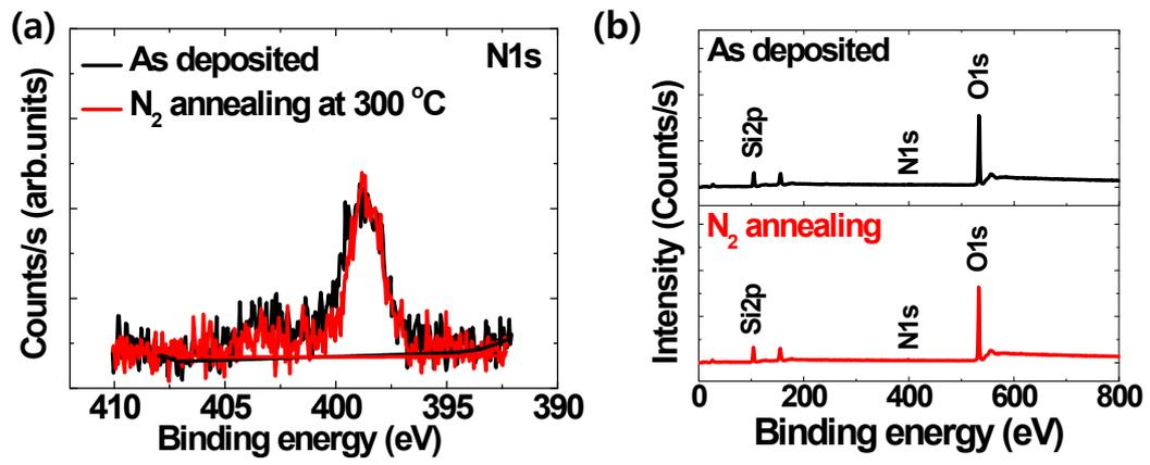
**Fig. S4** (a) N1s and (b) wide XPS spectra of NO-based SiO<sub>2</sub> films as deposited and N<sub>2</sub> annealing.
