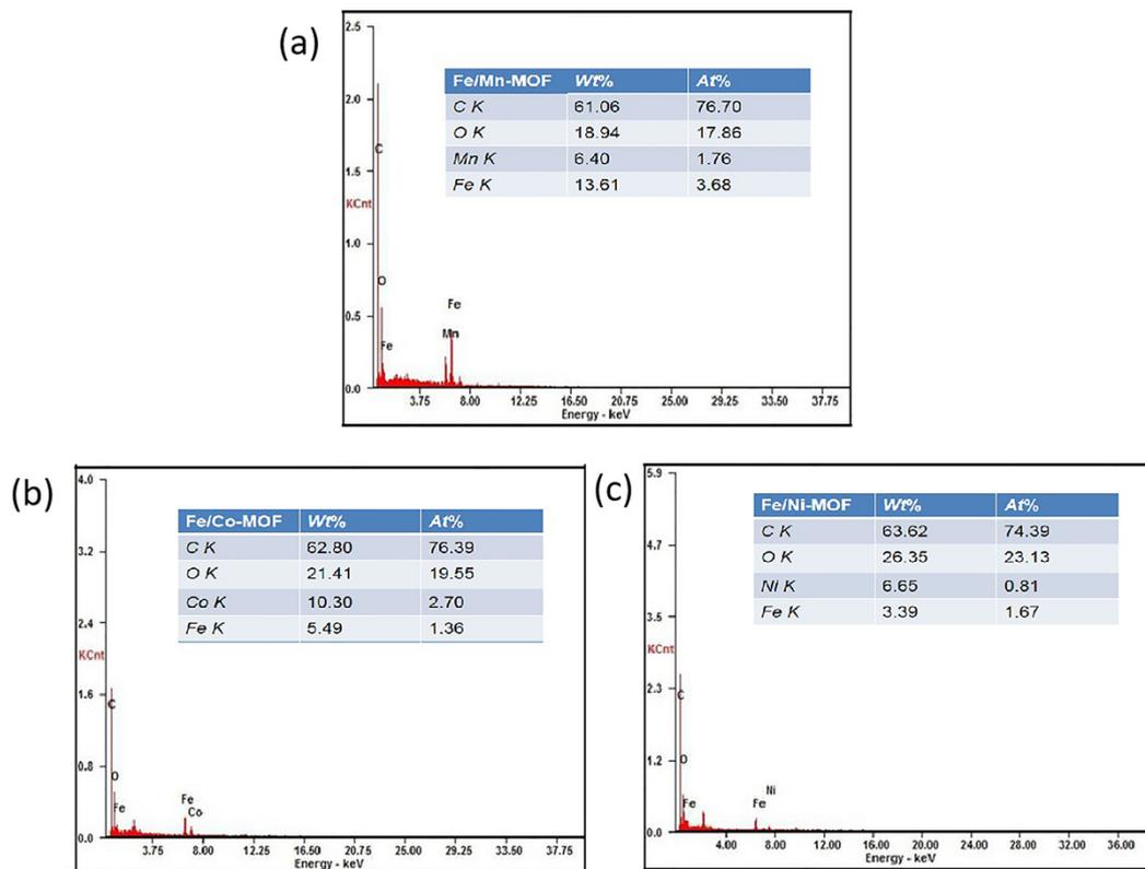
**Figure S2.** EDS spectra of (a) Fe/Mn-MOF; (b) Fe/Co-MOF; (c) Fe/Ni-MOF;
