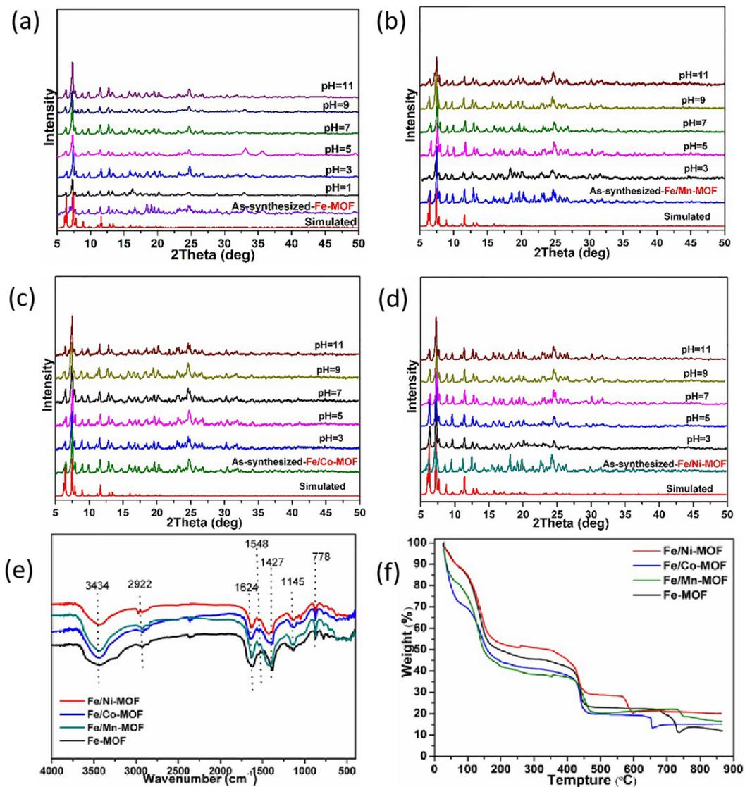
**Figure S1.** (a - d)The PXRD patterns of Fe<sub>2</sub>M-MOF ( M =Mn, Co, Ni) samples treated in water at different pH values for 12 h; (e) IR spectra of Fe/M-MOF (M =Mn, Co, Ni) materials and (f) TG curves.
