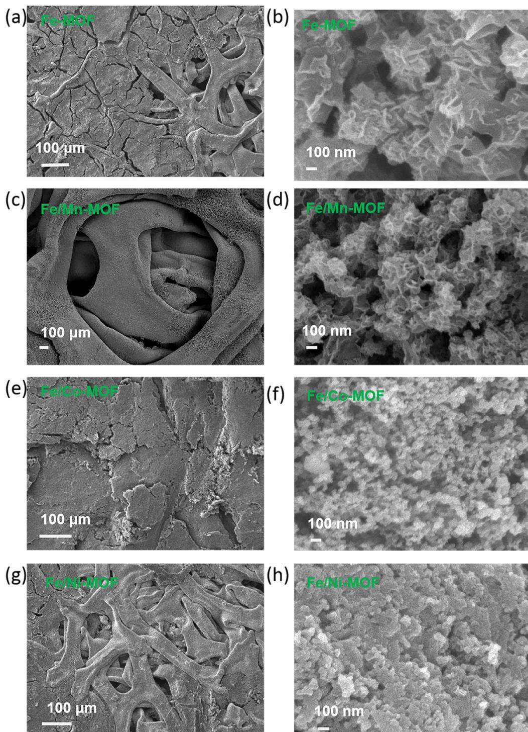
**Figure S4.** (a), (c), (e), and (g) samples loaded on foam nickel SEM images after 1000 Cycling and (b), (d), (f), and (h) samples of Fe-MOF, Fe/Mn-MOF, Fe/Co-MOF and Fe/Ni-MOF respectively.
