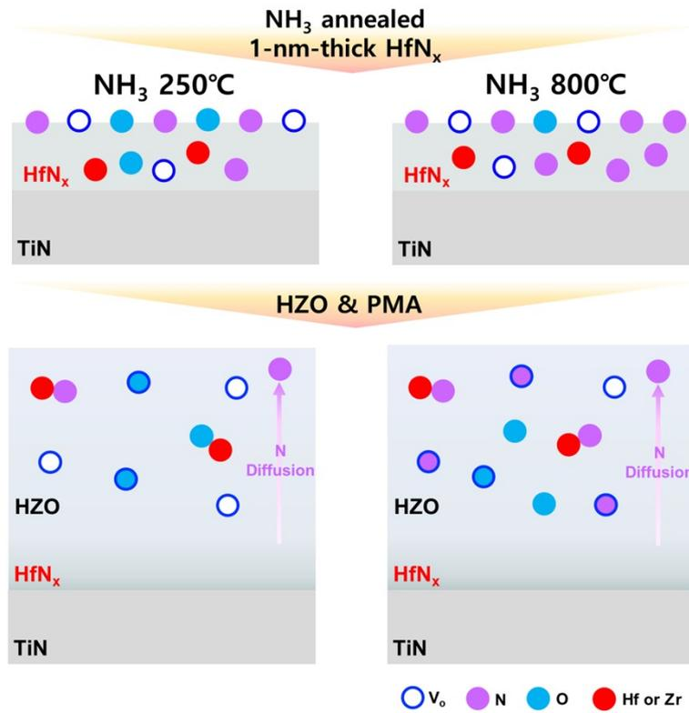
**Figure S4.** Schematic diagram depicting a proposed model for the role of nitrogen (N) and oxygen (O) in influencing the ferroelectric properties of 1-nm-thick HfN<sub>x</sub> films subjected to NH<sub>3</sub> annealing at 250 °C and 800 °C.
