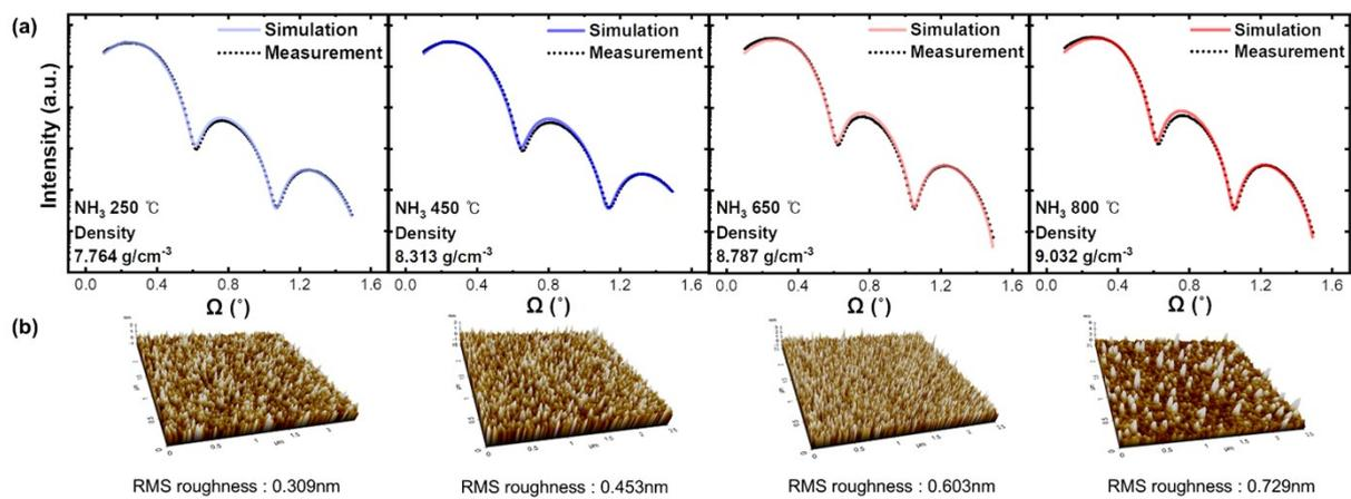
**Figure S3.** (a) XRR results and (b) AFM results of 10-nm-thick  $\text{HfN}_x$  films annealed in  $\text{NH}_3$  at 250 °C, 450 °C, 650 °C, and 800 °C, showing the measured film density and surface roughness.
