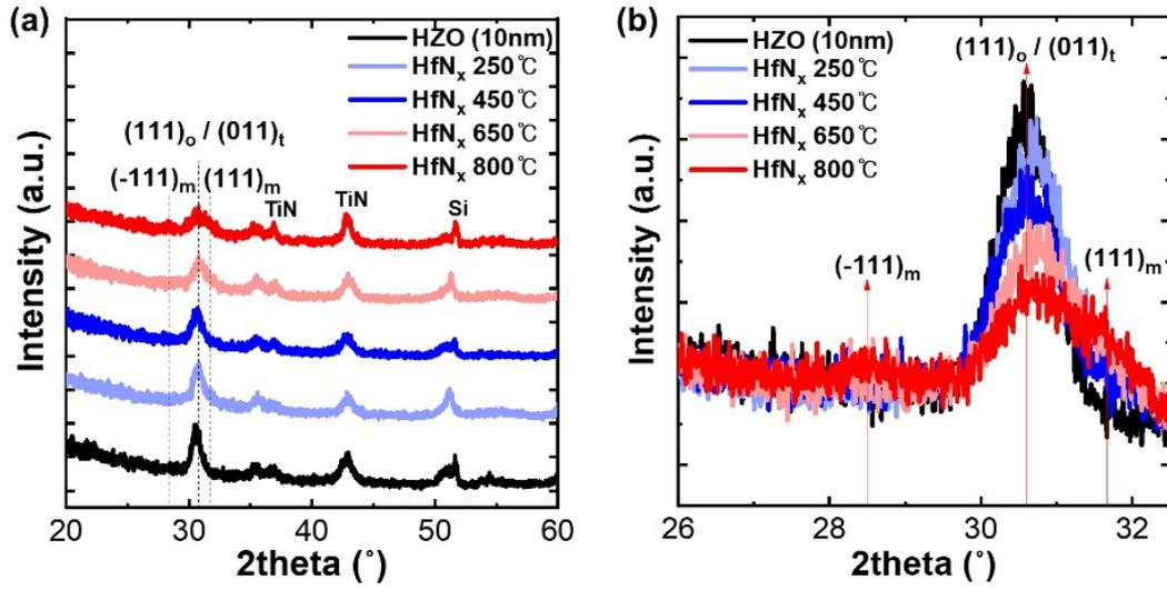
**Figure S2.** GIXRD patterns of 10-nm-thick HZO and HfN<sub>x</sub> IL samples annealed in NH<sub>3</sub> at various temperatures: (a) GIXRD patterns of the 10-nm-thick HZO and 1-nm-thick HfN<sub>x</sub> IL annealed at 250 °C to 800 °C, and (b) enlarged GIXRD patterns in the 26°-32.5° range.
