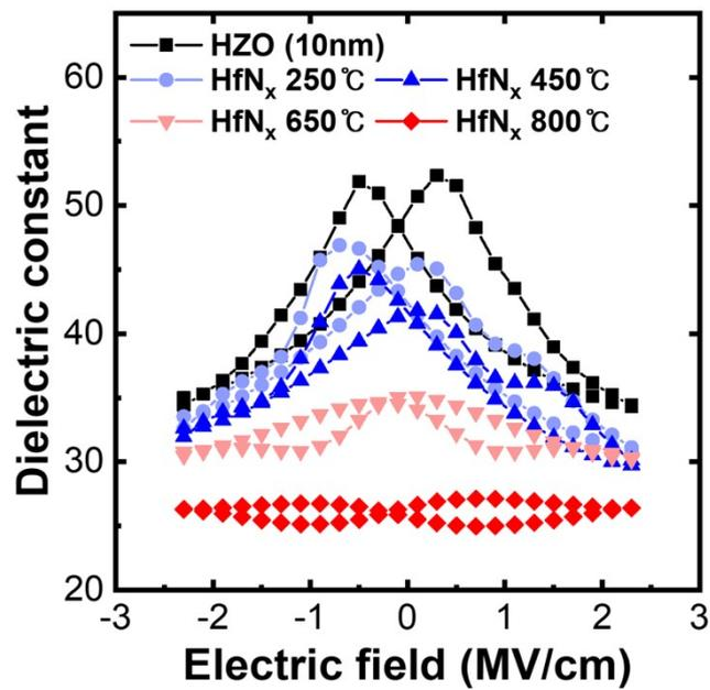
**Figure S5.**  $\epsilon_r$ -E curves of TiN/10-nm-thick HZO/TiN and TiN/HZO/HfN<sub>x</sub>/TiN capacitors annealed in NH<sub>3</sub> from 250 °C to 800 °C.
