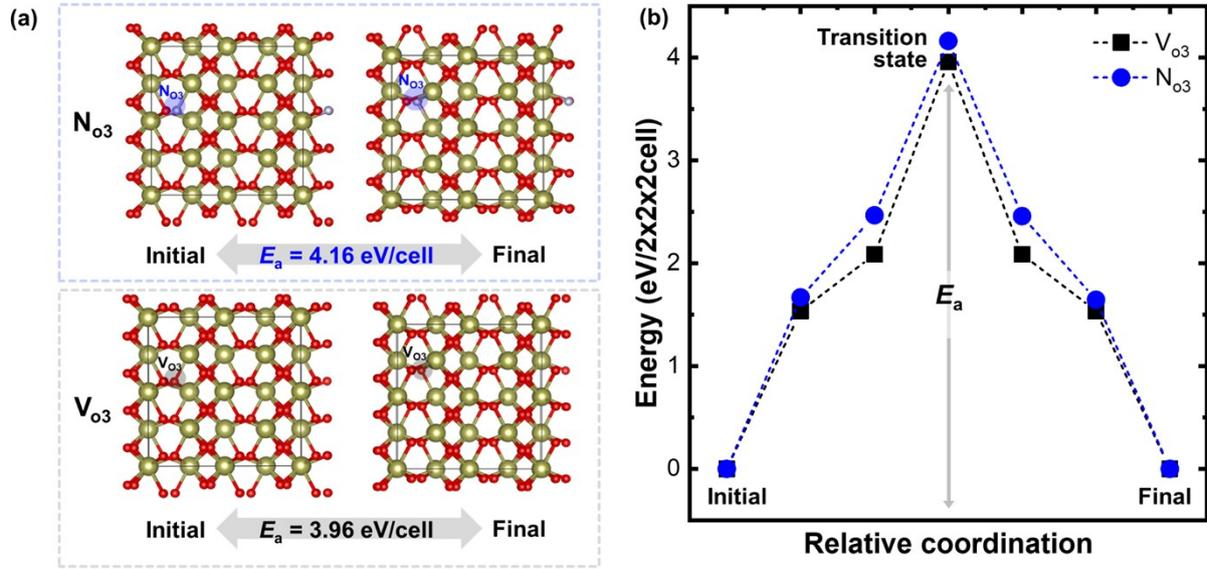
**Figure S6.** Calculated switching barrier for  $2 \times 2 \times 2$   $Pca2_1$   $HfO_2$  cells, including (a)  $N_{o3}$  and  $V_{o3}$ . Transition state calculations show (b) diffusion barriers of  $N_{o3}$  and  $V_{o3}$ .
