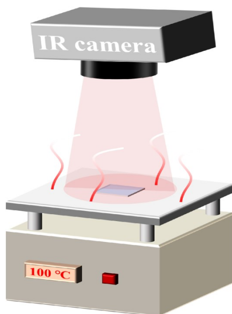
Figure S13. A Schematic representation of the IR thermal images test.
