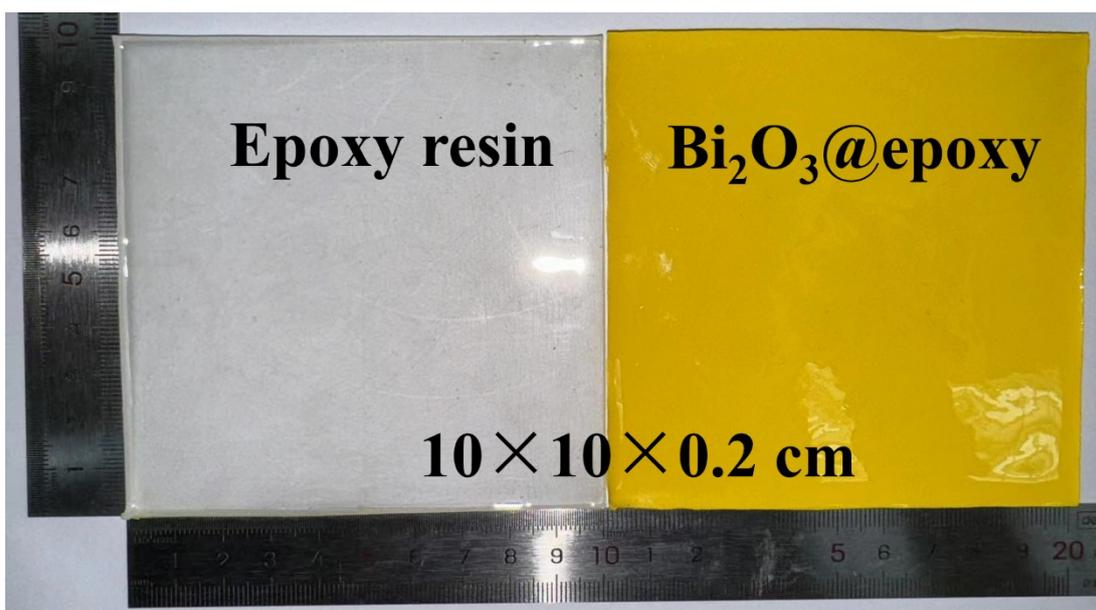
Fig. S1. Photographs of epoxy resin and Bi<sub>2</sub>O<sub>3</sub>@ epoxy composites prepared by mechanical co-mingling vacuum defoaming process
