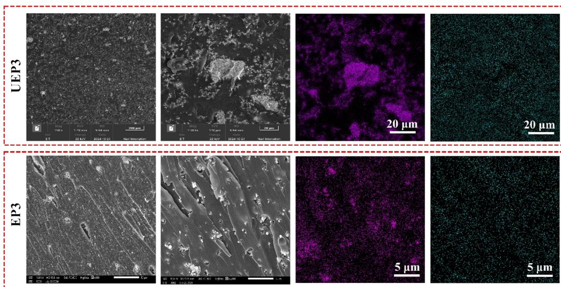
**Fig. S5** SEM of tensile sections of EP3 and UEP3
