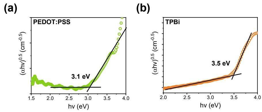
**Figure S4.** Tauc plot of PeLEDs: (a) PEDOT:PSS, and (b) TPBi.
