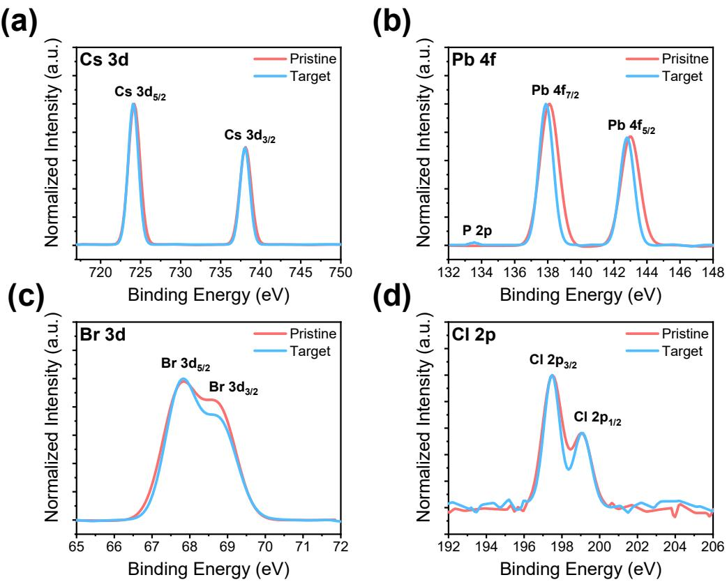
**Figure S2.** Binding energy spectra of pristine and doped (target) films: Normalized spectra of (a) Cs 3d, (b) Pb 4f and P 2p, and (c) Br 3d and Cl 2p.
