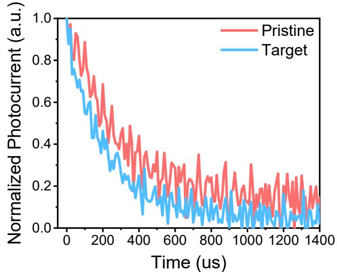
**Figure S8.** Normalized transient photocurrent (TPC) spectra of pristine and doped (target) devices.
