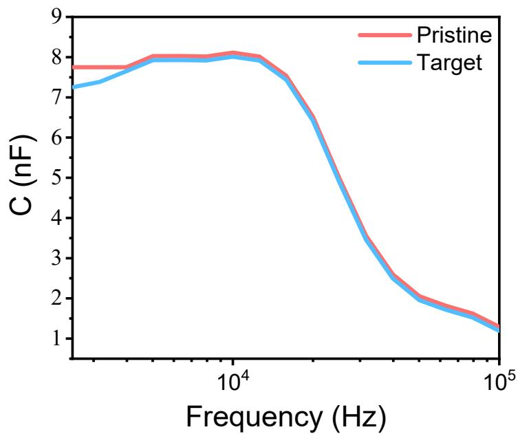
**Figure S9.** Extraction of the relative dielectric constant ( $\epsilon_r$ ) from capacitance-frequency measurements, using the device structure of ITO/PEDOT/perovskite/Al.
