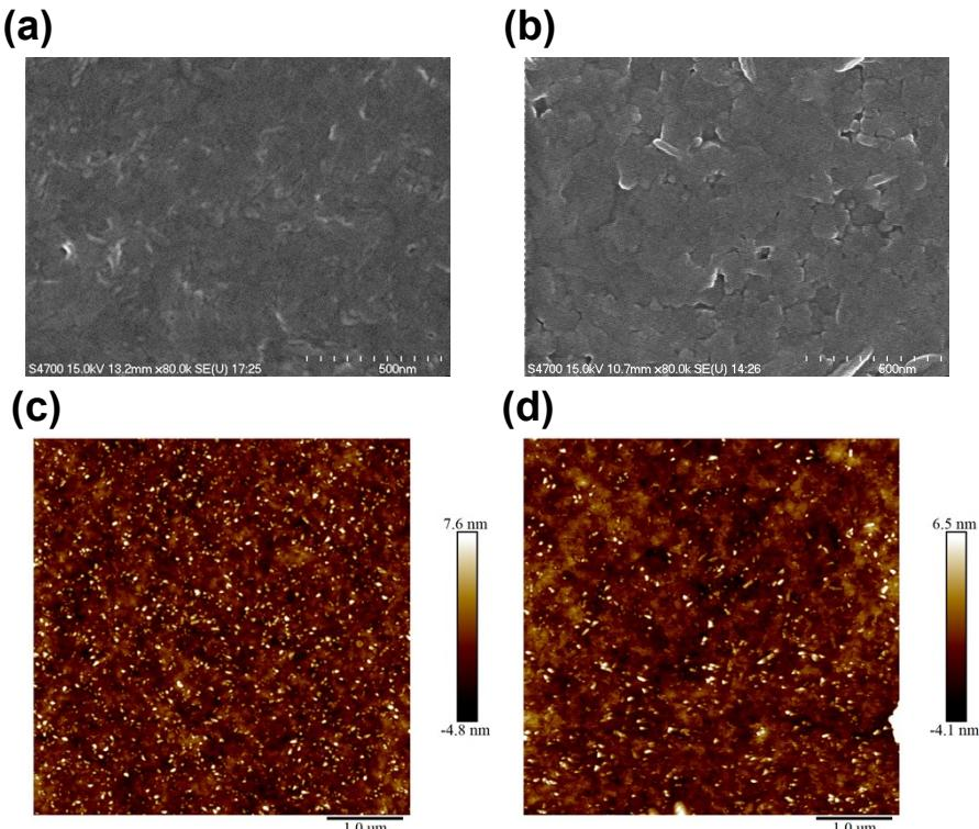
**Figure S11.** Sample surface images: (a), (b) Top-view scanning electron microscope (SEM) images of the pristine and doped (target) films. (c), (d) Atomic force microscope (AFM) images of the pristine and doped (target) films (scale bar: 1 μm).
