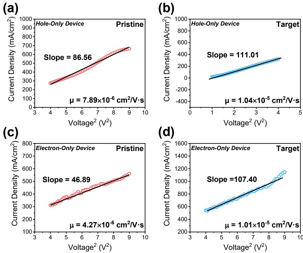
**Figure S10.** (a), (b) Hole mobility measurement using the SCLC method, with the hole-only devices structure ITO/PEDOT/perovskite/MoO<sub>3</sub>/Ag. (c), (d) Electron mobility measurement using the SCLC method, with the electron-only devices structure ITO/TPBi/perovskite/TPBi/LiF/Al.
