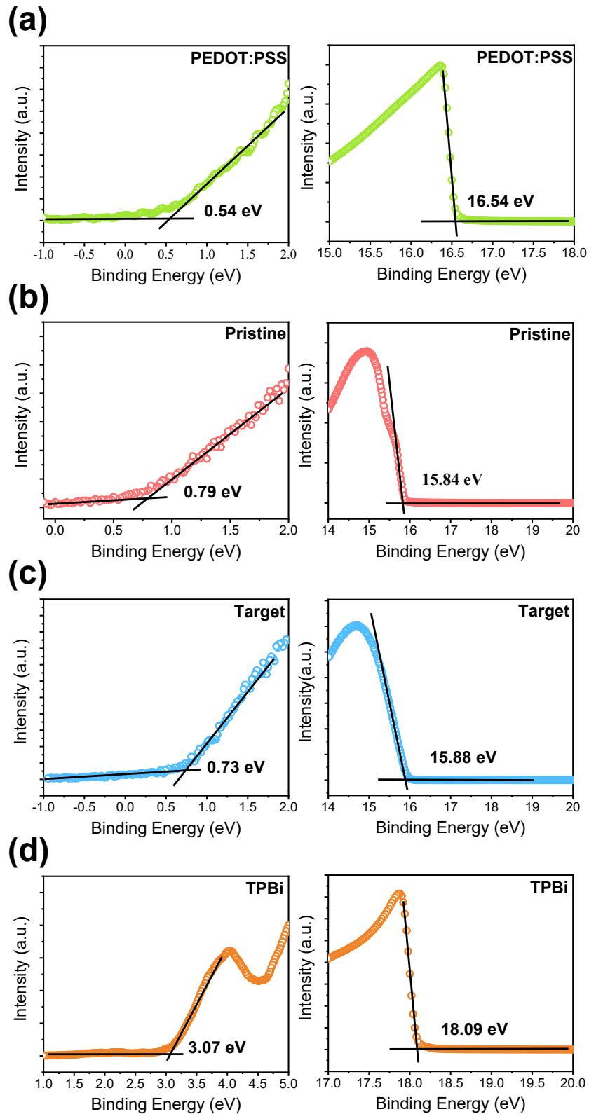
**Figure S5.** UPS spectra of PeLEDs: (a) PEDOT:PSS, (b) Pristine, (c) Doped (target), and (d) TPBi. A He I source with a photon energy of 21.22 eV was used for excitation in the UPS measurements. The calculated valence band energies were 5.22 eV for PEDOT:PSS, 6.17 eV for pristine, 6.07 eV for doped (target), and 6.20 eV for TPBi.
