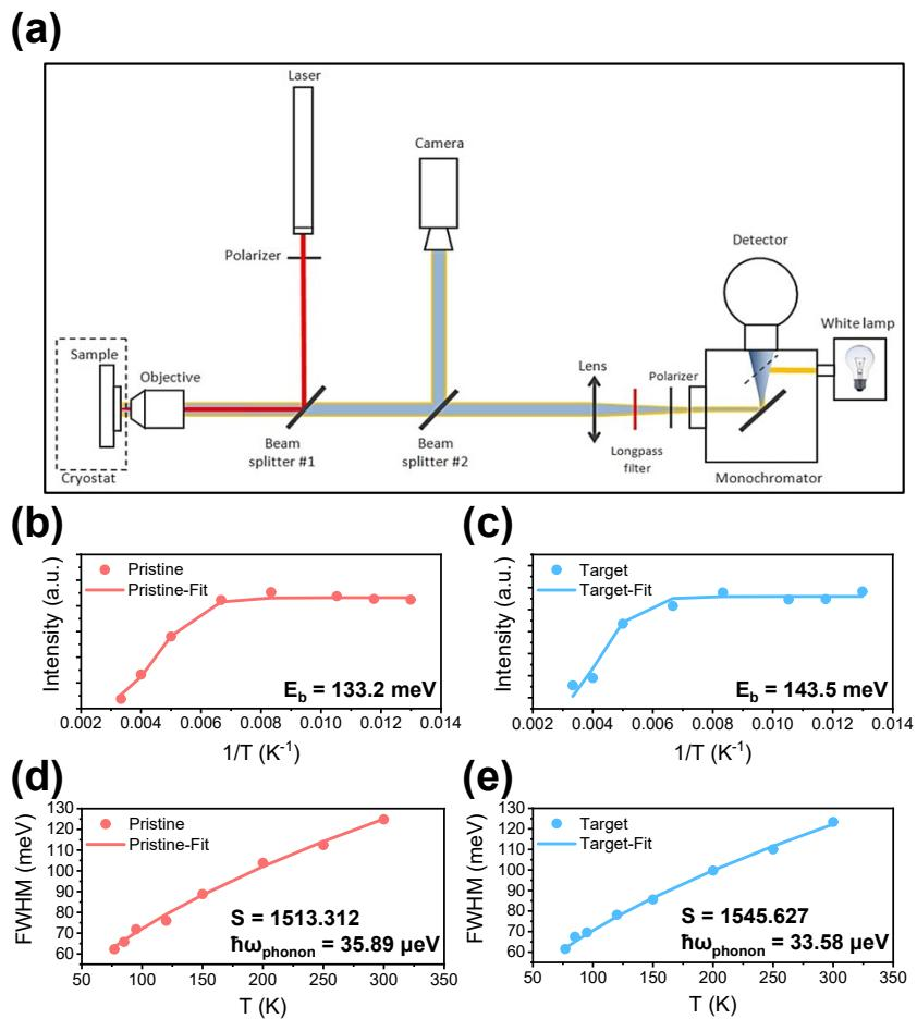
**Figure S7.** Temperature-dependent PL measurements and optical characteristics: (a) A schematic diagram of the optical setup for temperature-dependent PL measurements. (b) and (c) Exciton binding energy ( $E_b$ ) for pristine and doped (target) films obtained from the relationship between PL intensity and  $1/T$ . (d) and (e) Huang-Rhys factor ( $S$ ) for pristine and doped (target) films obtained by fitting the profile of FWHM vs.  $T$ .
