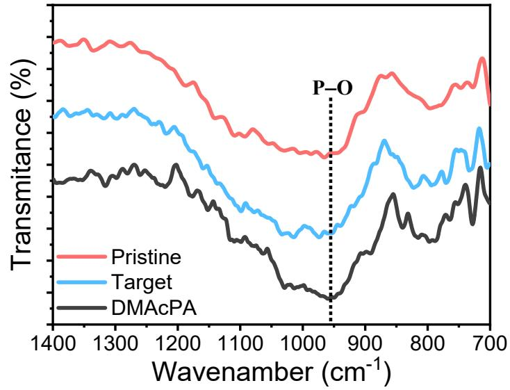
**Figure S3.** FTIR spectra of pristine and doped (target) films, compared with bare DMAcPA on glass.
