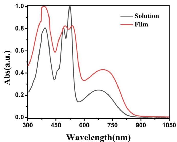
Figure S1 UV-Vis-NIR absorption spectra of S-PDI-IDT-1
