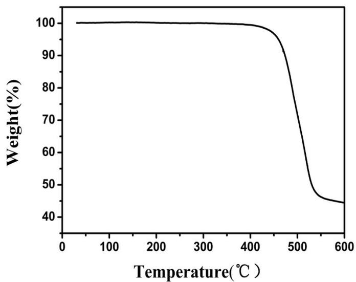
Figure S2 Thermogravimetric (TGA) analysis of S-PDI-IDT-1 measured at a heating rate of 10°C/ min in nitrogen
