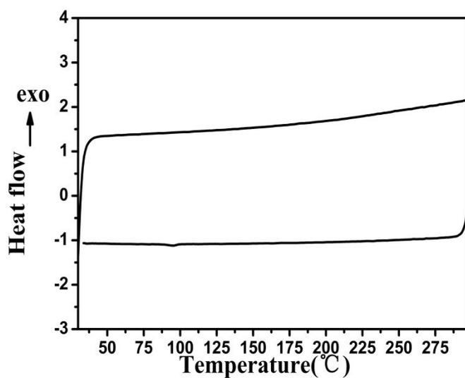
Figure S3 Differential scanning calorimetry (DSC) analysis of S-PDI-IDT-1 measured at a heating rate of 10°C/ min in nitrogen
