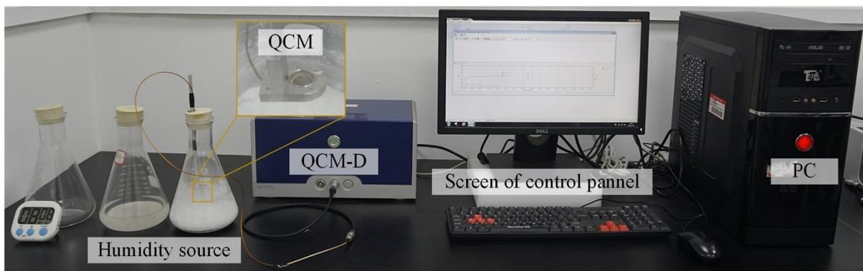
**Fig. S3.** Schematic diagram of the experimental setup for humidity detection by QCM-D.
