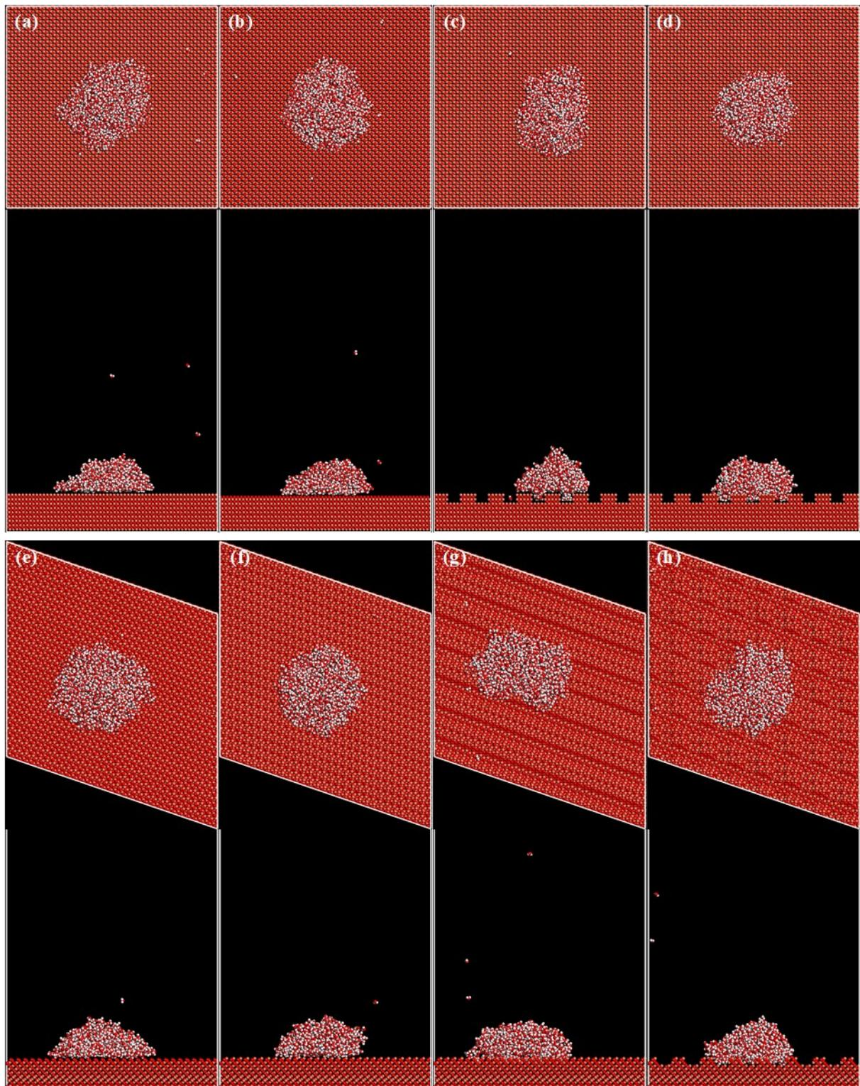
**Fig. S18.** Water droplet on the (002) CuO surface with (a) flat Cu; (b) flat O; (c) groove array; (d) micro-pit array after simulation. Water droplet on the (111) CuO surface with (e) flat Cu; (f) flat O; (g) groove array; (h) micro-pit array after simulation.
