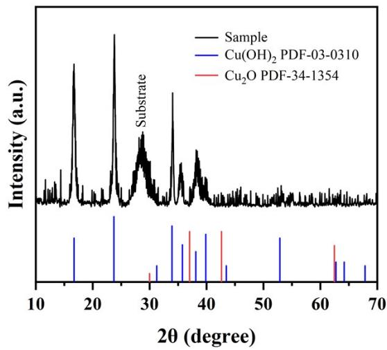
**Fig. S11.** XRD pattern of the Cu(OH)<sub>2</sub> nanowires before annealing.
