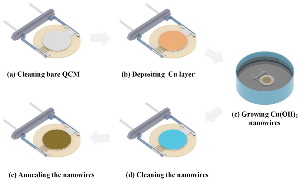
**Fig. S2.** Flow protocols of the fabrication for CuO nanowires based QCMs. **(a)** Cleaning bare QCMs, **(b)** depositing Cu layer, **(c)** in-situ growing the Cu(OH)<sub>2</sub> nanowires in solution, **(d)** Cu(OH)<sub>2</sub> nanowires QCM humidity sensor, **(e)** in-situ annealing Cu(OH)<sub>2</sub> nanowires in air.
