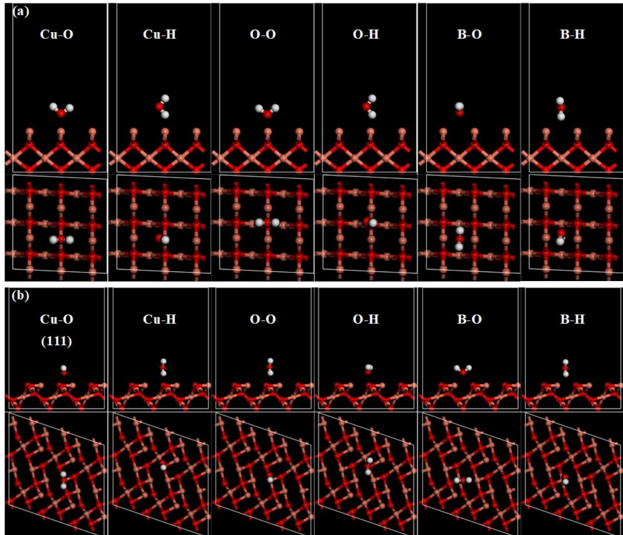
**Fig. S5.** Adsorption geometries of  $\text{H}_2\text{O}$  on the CuO surfaces. (a) (002); (b) (111). The salmon pink, red and gray balls represent Cu, O, and H atoms, respectively.
