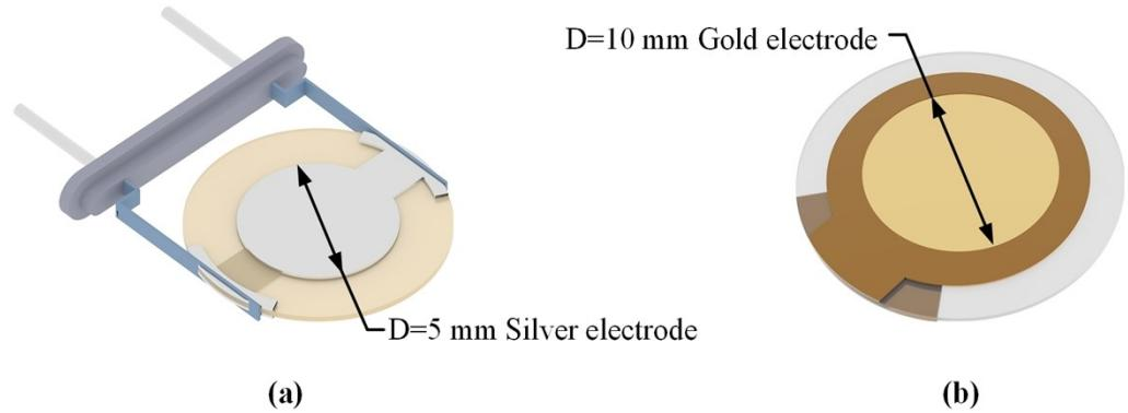
**Fig. S1.** (a) Structure of bare QCMs with an AT crystal (8 mm in diameter) and two silver electrodes (5 mm in diameter); (b) Structure of bare QCMs with an AT crystal (15 mm in diameter) and two gold electrodes (10 mm in diameter).
