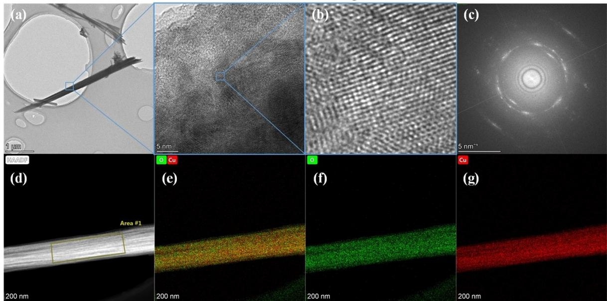
**Fig. S9.** TEM images, HRTEM images, SEAD images and Element mapping of the nanowires before and after annealing.
