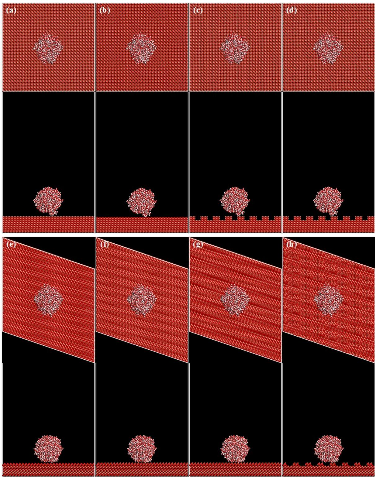
**Fig. S4.** Water droplet on CuO (111) surface (a) Cu; (b) O; (c) stripe groove; (d) vertical and horizontal groove; Water droplet on CuO (002) surface (e) Cu; (f) O; (g) stripe groove; (h) vertical and horizontal groove.
