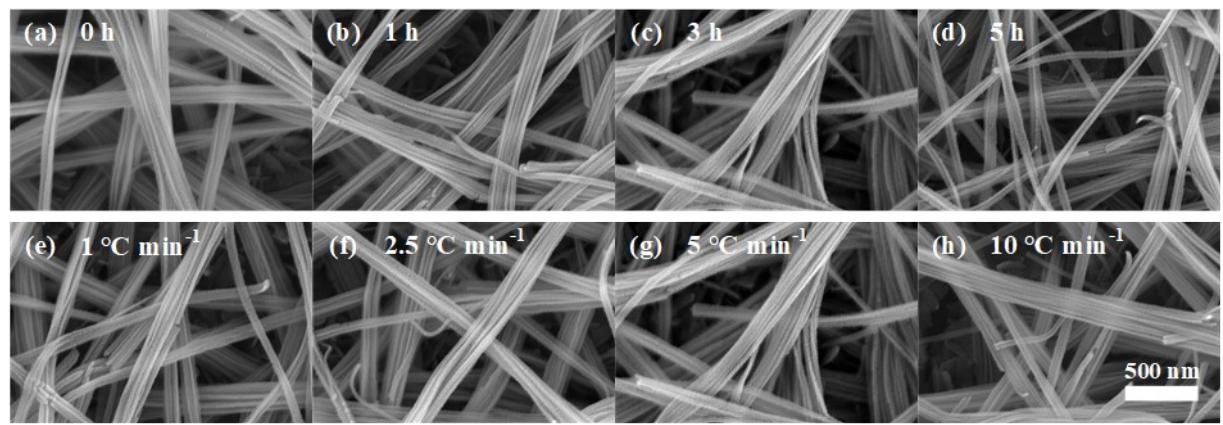
**Fig. S8.** SEM images of the CuO nanowires after annealing at 300 °C for (a) 0 h, (b) 1 h, (c) 3 h and (d) 5 h; at 300 °C for 3 h with a heating rate of (e) 1 °C min<sup>-1</sup>, (f) 2.5 °C min<sup>-1</sup>, (g) 5 °C min<sup>-1</sup> and (h) 10 °C min<sup>-1</sup>.
