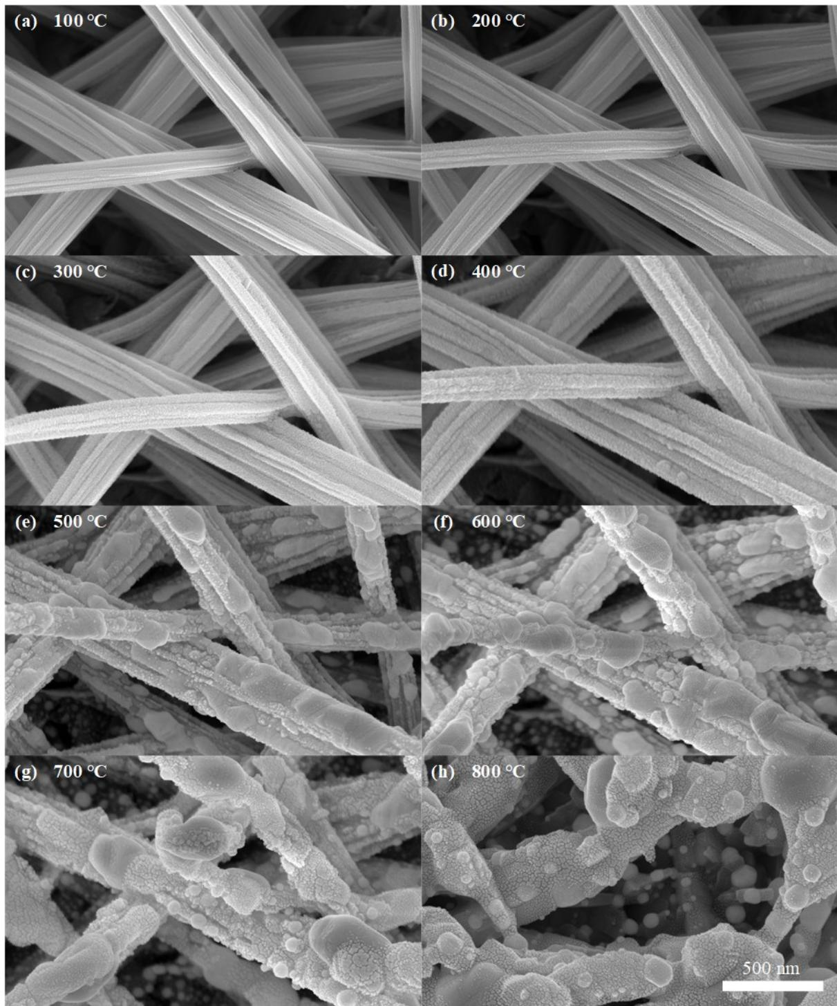
**Fig. S6.** The SEM images of the nanowires annealed at (a) 25°C, (b) 200°C, (c) 300°C, (d) 400°C, (e) 500°C, (f) 600°C, (g) 700°C, (h) 800°C last for 1 hour with a heating rate of 5 °C/min.
