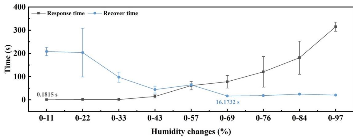
**Fig. S16.** The response/recovery time of the sensor under different humidity levels.
