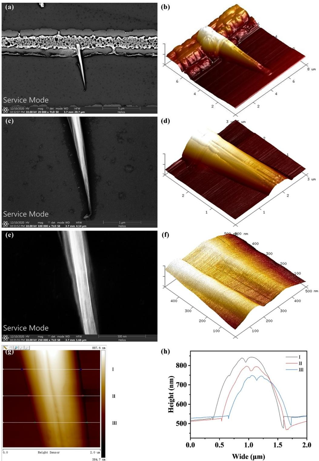
**Fig. S19.** (a, c, e) AFM images and (b, d, f) sectional views of the single CuO nanowire at different magnifications; (g) Height distribution image of the single CuO nanowire and (h) its corresponding sectional height curves.
