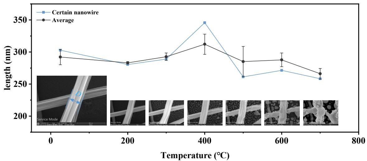
**Fig. S7.** The width of the nanowires vs. annealing temperature.
