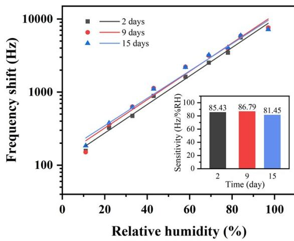
**Fig. S17.** The response curves of the sensor after long-term storage.
