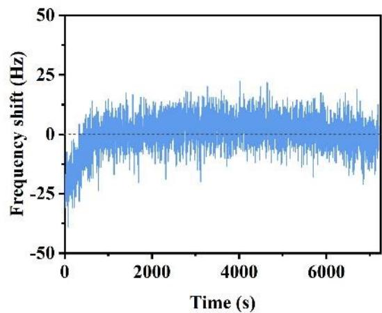
**Fig. S23.** The robust humidity sensing capability of the CuO nanowires based QCMs.
