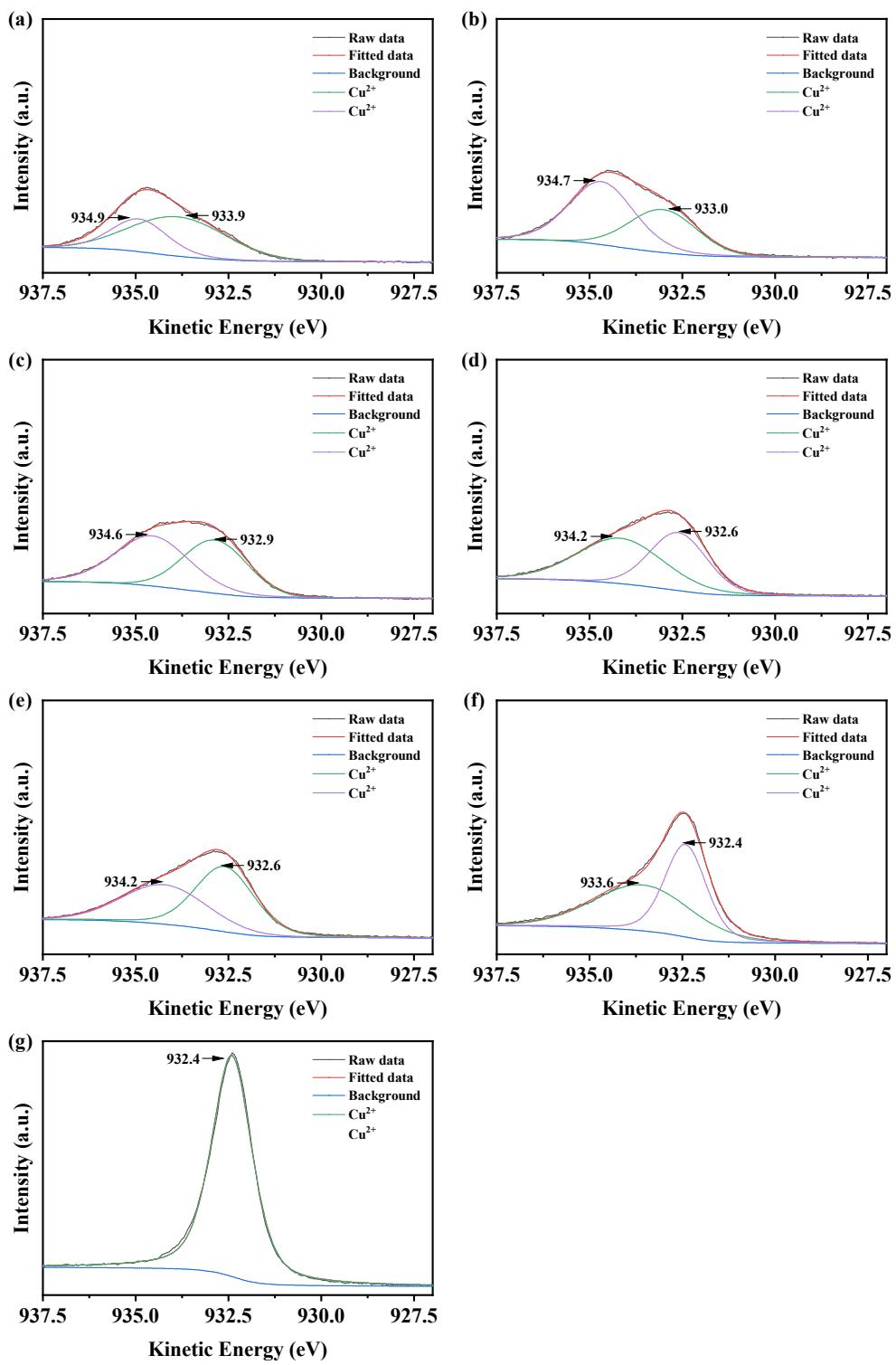
**Fig. S12.** XPS curves of Cu element of sensing materials at **(a)** 30°C; **(b)** 100°C; **(c)** 140°C; **(d)** 160°C; **(e)** 200°C; **(f)** 300°C; **(g)** 400°C.
