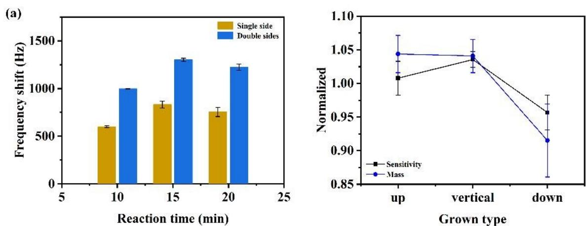
**Fig. S15.** The performance of the sensor with different (a) reaction times and (b) growing types.
