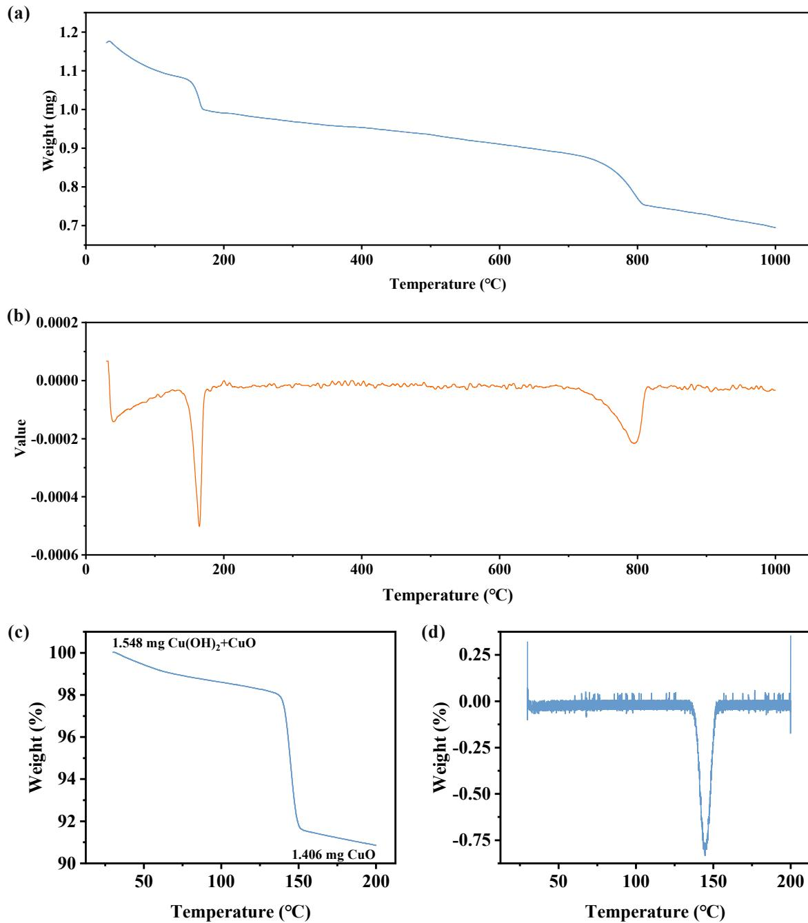
**Fig. S14.** **(a)** The weight of the sensing materials *vs.* temperature; **(b)** differential coefficient of the weight of the sensing materials *vs.* temperature (25°C~1000°C). **(c)** The weight of the sensing materials *vs* temperature; **(d)** differential coefficient of the weight of the sensing materials *vs* temperature (25°C~200°C).
