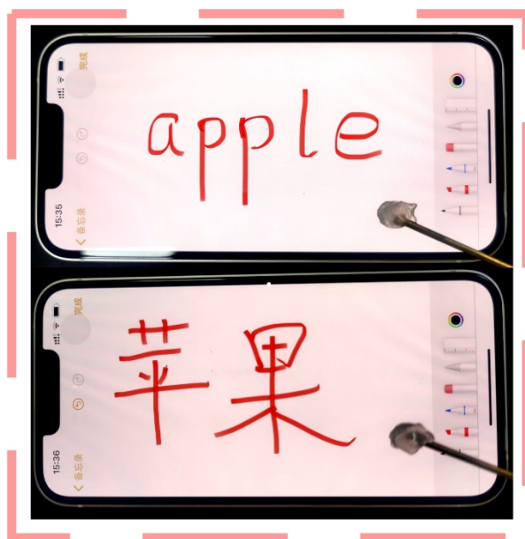
Fig. S9. Potential application of MFI hydrogel as a dielectric assembled in a capacitive pen writing “Apple” in English and in Chinese on the mobile phone screen.
