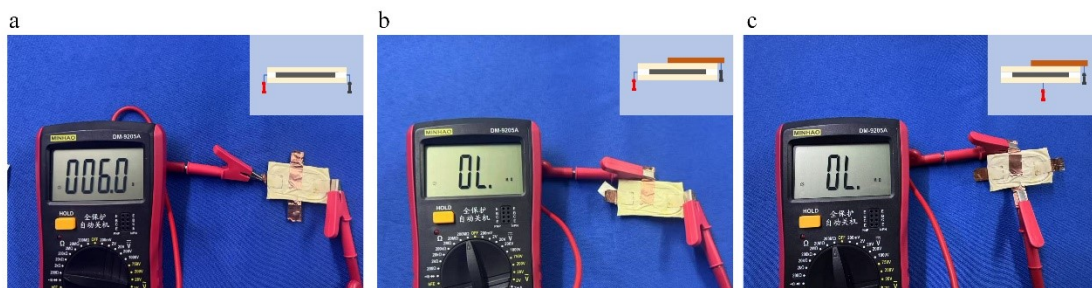
Figure S18 Electrical insulation properties of the samples with protection layer
