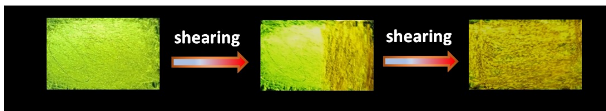
Figure S24. Illustration of the mechanochromic behavior induced by shearing a DTBTE film on a glass slide with a spatula, visualized under a UV lamp (356 nm).
