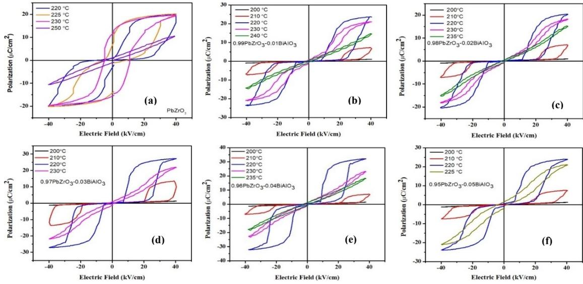
Figure S3. (a-f) Polarization-electric field (P-E) relations measured under electric fields of  $\pm 40$  kV/cm at 10 Hz frequency at various temperatures between 200 and 250 °C.
