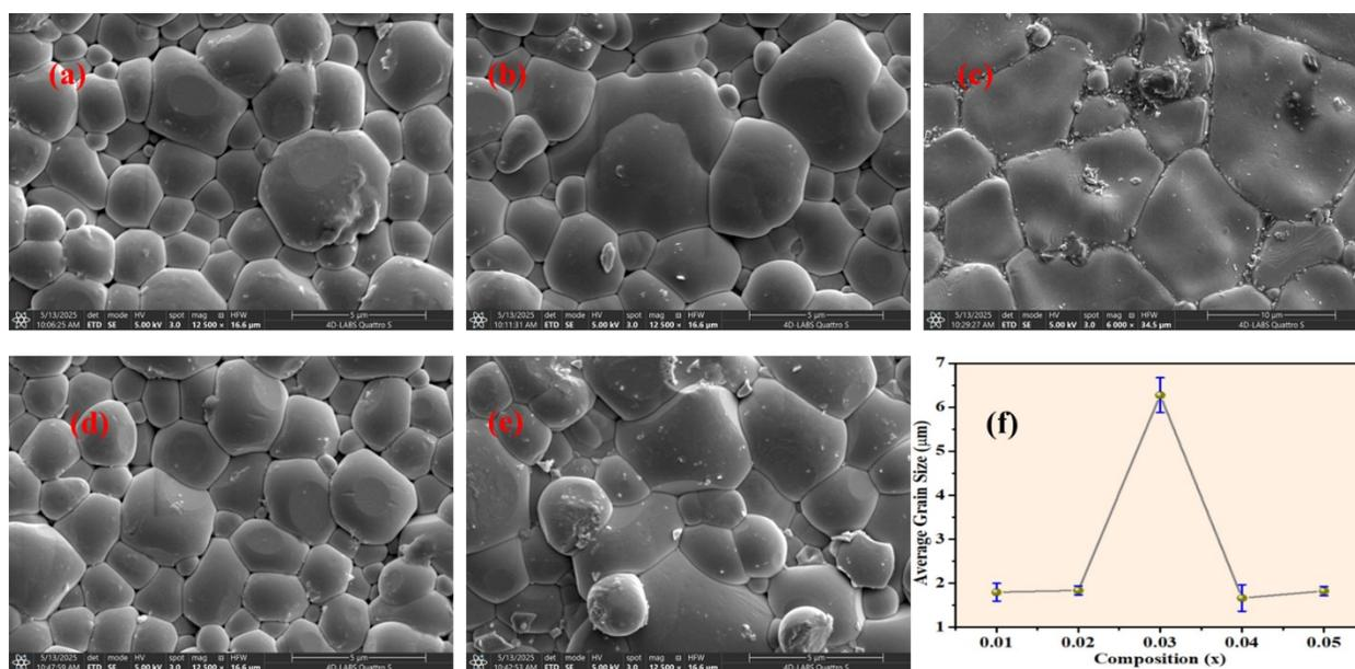
Figure S1. (a-f) SEM images of the surfaces of as sintered (1-x) $\text{PbZrO}_3$ -x $\text{BiAlO}_3$  ceramics: (a) x = 0.01, (b) x = 0.02, (c) x = 0.03, (d) x = 0.04 and (e) x = 0.05. (f) Variation of the average grain size as a function of  $\text{BiAlO}_3$  concentration, with error bars presented by blue colour.
