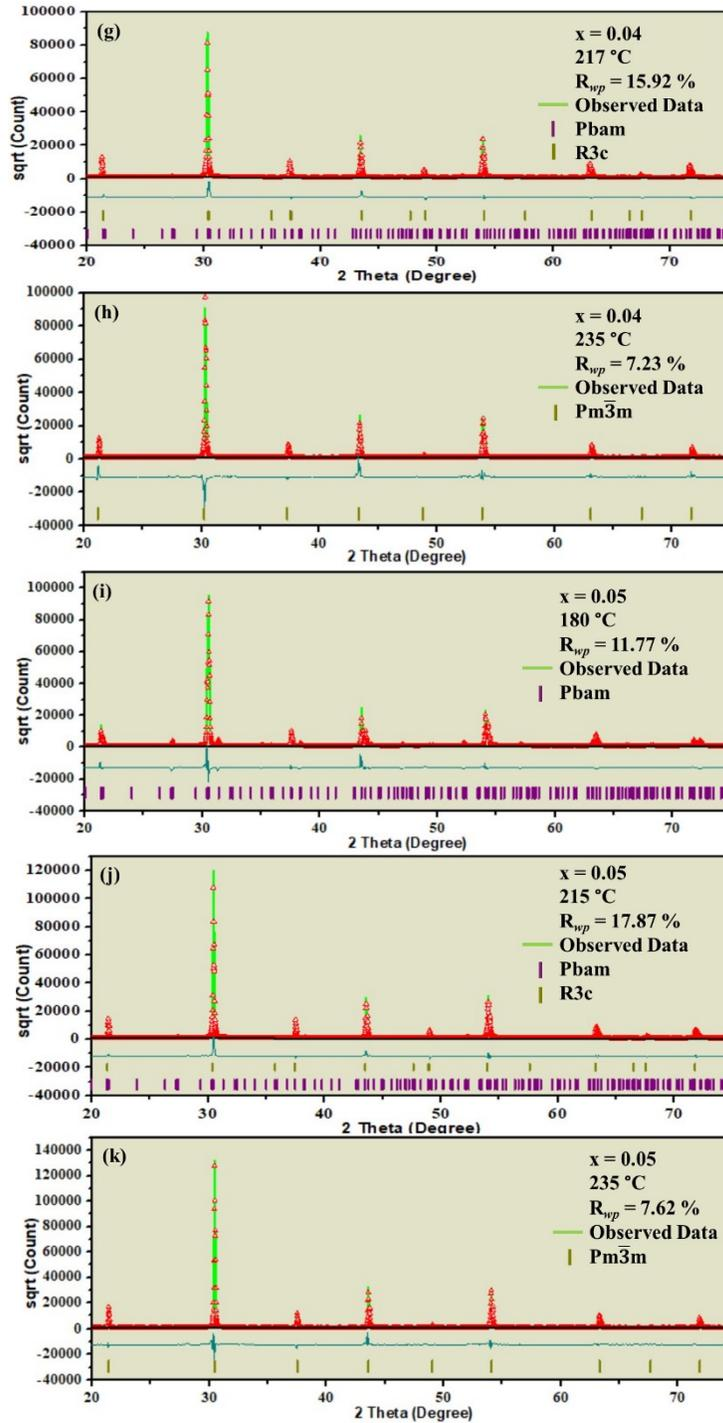
Figure S2. (a-k) Rietveld refinement results of the X-ray powder diffraction patterns of  $x = 0.01$ ,  $0.02$ ,  $0.04$  and  $0.05$  ceramic measured at different temperatures. The Pbam space group is used to refine the data below  $T_{C1}$ . The  $\text{Pm}\bar{3}\text{m}$  symmetry is used to refine the data above  $T_{C2}$ . For the intermediate phase the refinement is performed by using a combination of R3c and Pbam phases.
