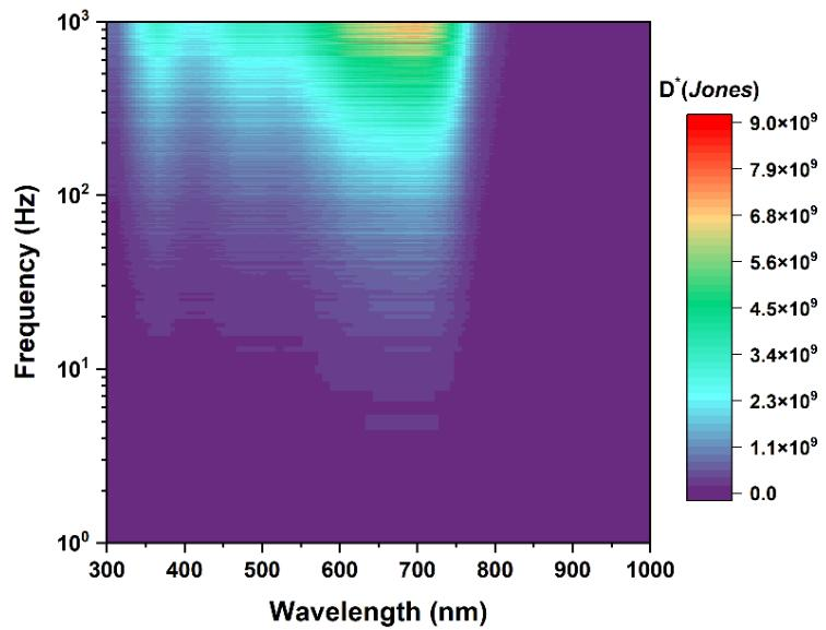
**Fig. S3.**  $D^*$  spectra of binary device from noise.
