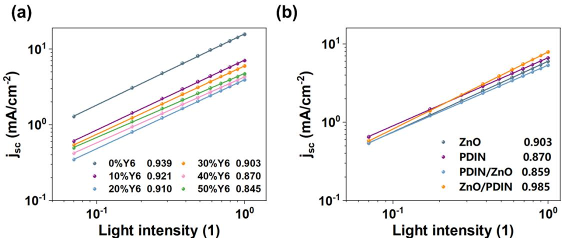
**Fig. S9.** (a-b) Dependence of short-circuit current on light intensity of OPDs with different Y6 weight fractions and ETLs.
