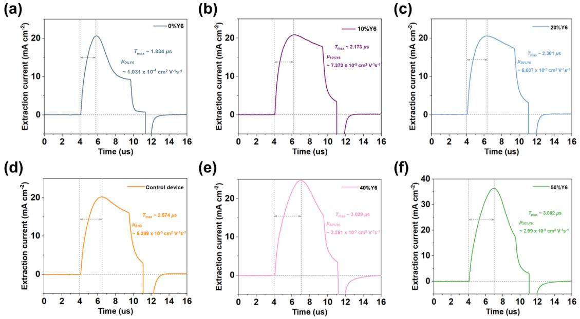
**Fig. S10.** (a-f) Carrier mobility of OPDs with different Y6 weight fractions.
