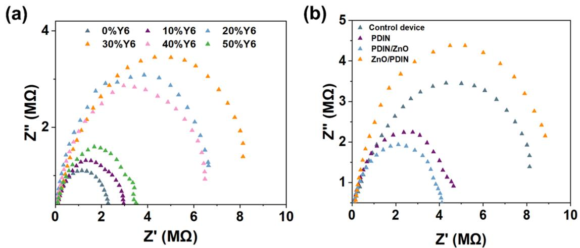
**Fig. S6.** Impedance spectra of OPDs with (a) different Y6 weight fractions and (b) different ETLs.
