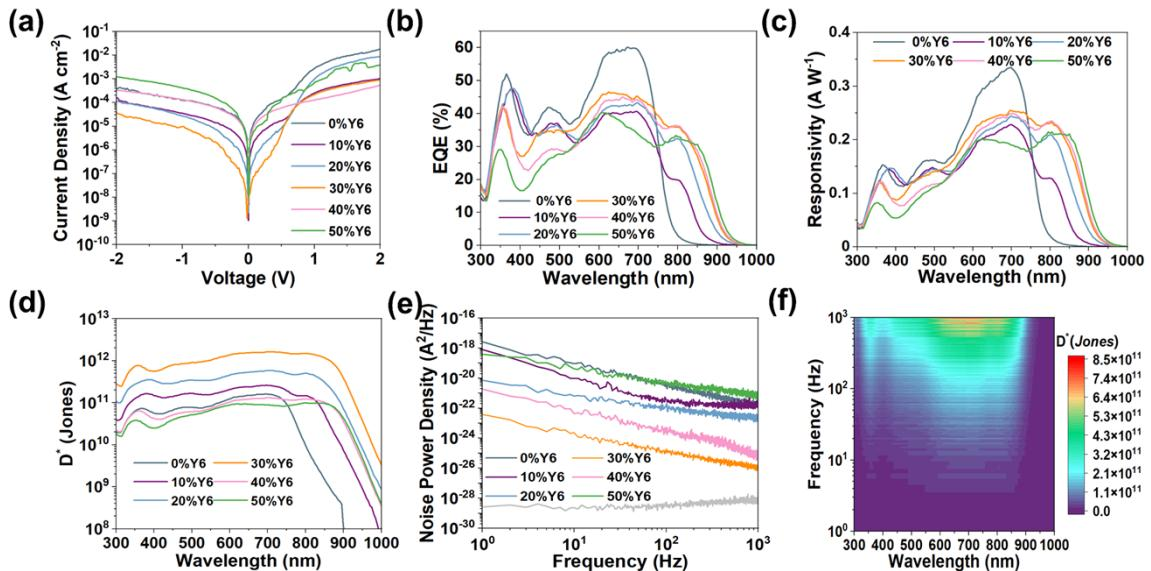
**Fig. S2** (a) The dark J-V curves, (b) EQE curves, (c) Responsivity curves, (d) Specific detectivity curves obtained from  $J_D$ , (e) Noise spectral densities, and (f) NIR-specific detectivity spectra obtained from the noise current for OPDs with different  $\text{Y6}$  weight fractions.
