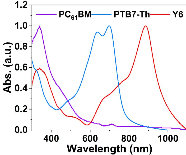
**Fig. S1.** Normalized absorption spectra of three materials,  $\text{PC}_{61}\text{BM}$ ,  $\text{PTB7-Th}$ ,  $\text{Y6}$ .
