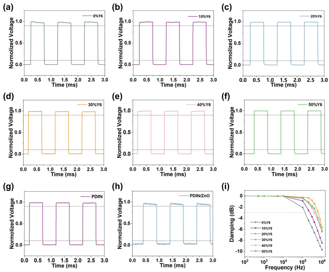
**Fig. S12.** (a-h) The response speed of OPDs with different Y6 weight fractions and ETLs. (i) -3dB cutoff frequency of OPDs with different Y6 weight fractions.
