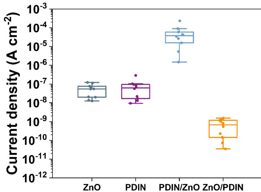
**Fig. S4.** Dark current box plots of 10 devices fabricated separately under different ETLs.
