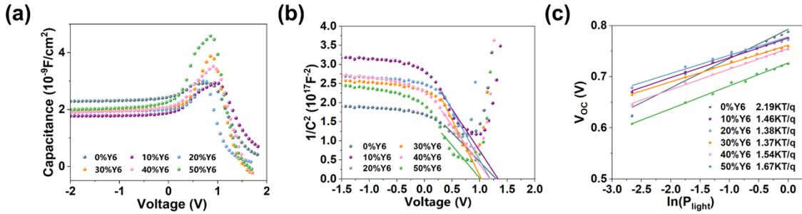
**Fig. S7.** (a) Capacitance-Voltage curves, (b) Mott Schottky curves, and (c) Dependence of the open-circuit voltage on light intensity of OPDs with different Y6 weight fractions.
