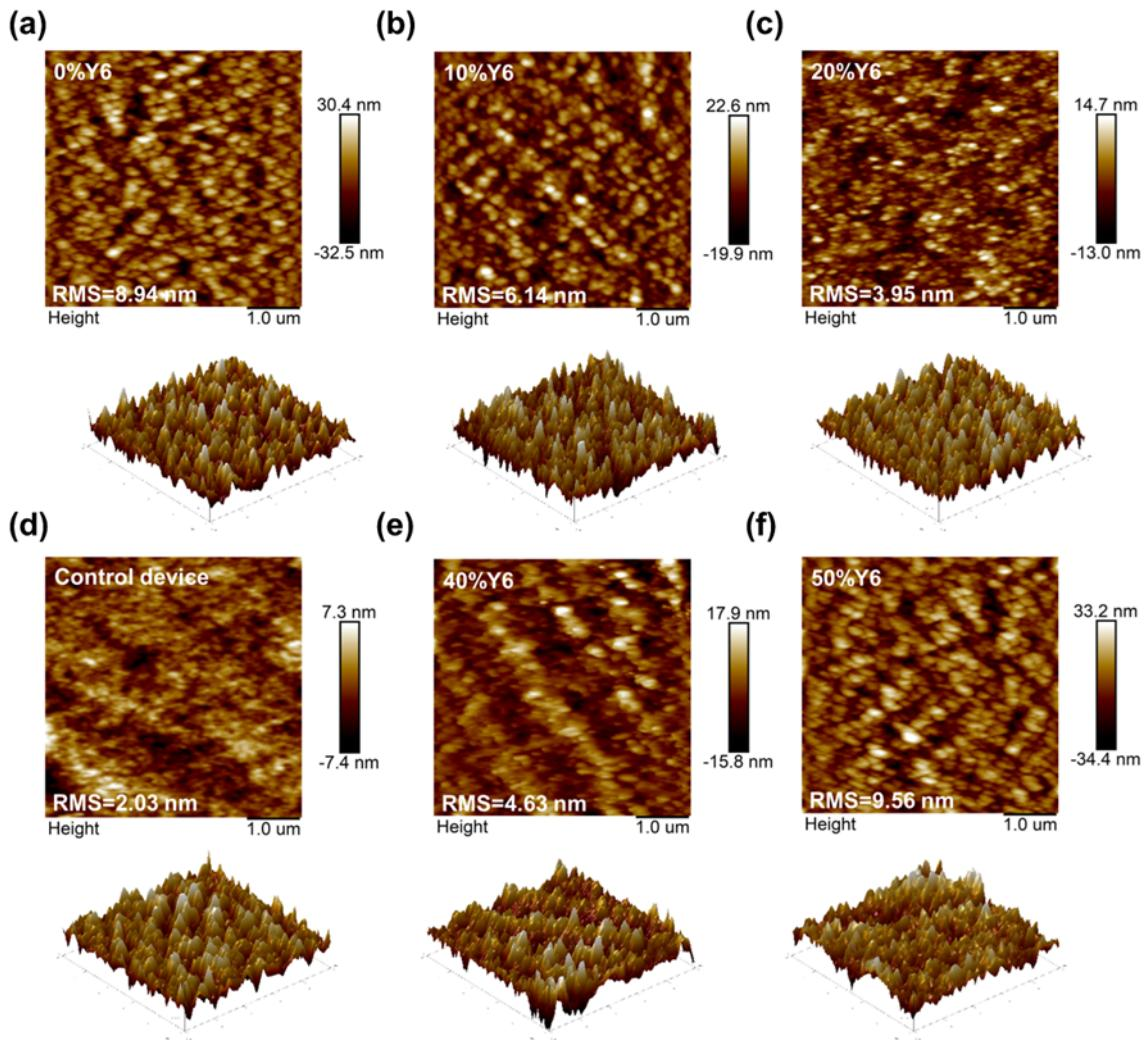
**Fig. S5.** AFM height images ( $5 \times 5 \mu\text{m}$ ) and 3D AFM diagrams of the active layers on (a) 0%Y6, (b) 10%Y6, (c) 20%, (d) 30%Y6, (e) 40%Y6, and (f) 50%Y6.
