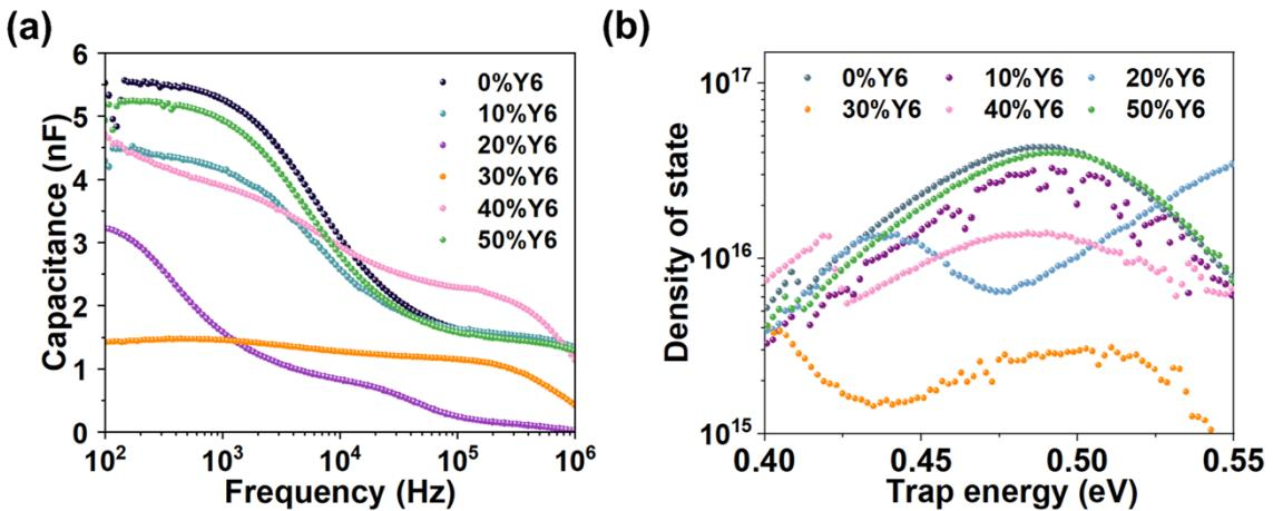
**Fig. S8.** (a-b) Capacitance-Frequency curves and trap density of state curves of OPDs with different Y6 weight fractions.
