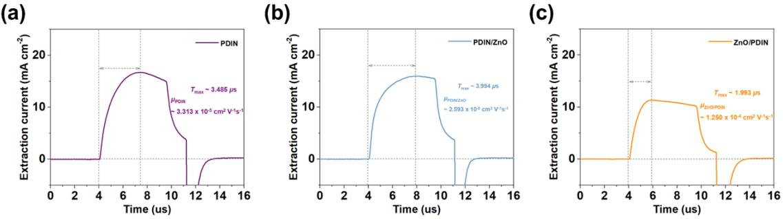
**Fig. S11.** (a-c) The carrier mobility of OPDs with different ETLs.
