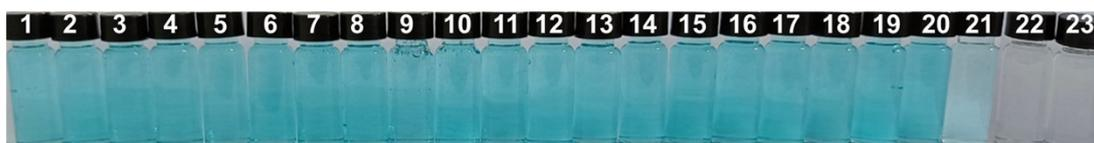
**Figure S4.** Color of **Dma** solution under daylight illumination after the addition of various analytes (1: Blank, 2:  $CO_3^{2-}$ , 3:  $HCO_3^-$ , 4:  $C_2O_4^{2-}$ , 5:  $CH_3COO^-$ , 6: PPI, 7:  $HPO_4^{2-}$ , 8:  $SO_4^{2-}$ , 9:  $S_2O_3^{2-}$ , 10:  $SCN^-$ , 11:  $HS^-$ , 12:  $N_3^-$ , 13:  $NO_2^-$ , 14:  $F^-$ , 15:  $Cl^-$ , 16:  $Br^-$ , 17:  $I^-$ , 18: Cys, 19: Hcy, 20: GSH, 21:  $S^{2-}$ , 22:  $SO_3^{2-}$ , 23:  $HSO_3^-$ ).
