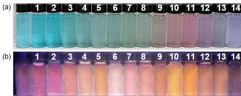
**Figure S7.** Daylight (above) and Fluorescent (below) color changes of **Dma** ( $10\ \mu\text{M}$ ) on the addition of various amines in DMSO/ $\text{H}_2\text{O}$  (4/6, v/v, pH=6.4). (1: Blank, 2: ANI, 3: TMA, 4: TYA, 5: PEA, 6: DEA, 7: TPA, 8: CHA, 9: PPA, 10: TEA, 11: DEA, 12: SPE, 13: PUT, 14: CAD).
