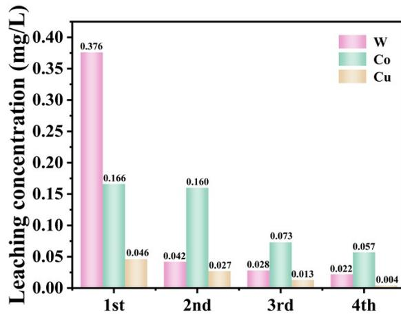
Fig. S6 Leached concentrations of W, Co, and Cu in the CCW/PMS/Vis system.
