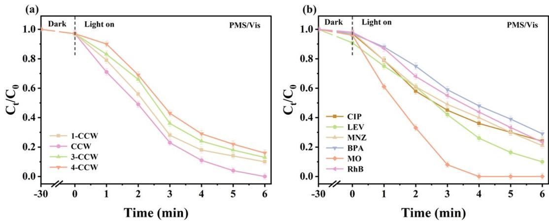
Fig. S4(a) The activity of CW with different copper doping amounts for TC degradation. (b) The performance of the CCW/PMS/Vis system in removing various pollutants.
