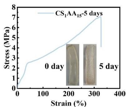
**Fig. S6:** Stress-strain curves of  $CS_1AA_{15}$  hydrogel stored at 25 °C and 54% RH for 5 days.
