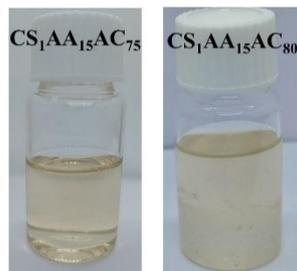
**Fig. S1:** Optical photographs of precursor solutions at CS:H<sub>2</sub>O:AA:AC ratios of 1:5:15:75 and 1:5:15:80, respectively.
