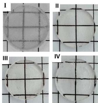
**Fig. S4:** Optical photograph of (I)  $CS_1AA_{15}$  (II)  $CS_1AA_{15}AC_{25}$  (III)  $CS_1AA_{15}AC_{50}$  (IV)  $CS_1AA_{15}AC_{75}$  hydrogel transparency.
