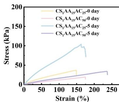
**Fig. S8:** Stress-strain curves of CS<sub>1</sub>AA<sub>15</sub>AC<sub>25</sub>, CS<sub>1</sub>AA<sub>15</sub>AC<sub>50</sub> hydrogels initial and stored at 25 °C and 54% RH for 5 days
