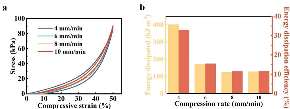
**Fig. S3:** (a) Loading-unloading test of CS<sub>1</sub>AA<sub>15</sub>AC<sub>75</sub> hydrogel at different compression rates (b) Calculation of energy dissipated at different compression rates of CS<sub>1</sub>AA<sub>15</sub>AC<sub>75</sub> hydrogel at 50% strain vs. energy dissipation efficiency.
