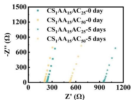
**Fig. S9:** Impedance of CS<sub>1</sub>AA<sub>15</sub>AC<sub>25</sub>, CS<sub>1</sub>AA<sub>15</sub>AC<sub>50</sub> hydrogels initial and stored at 25 °C and 54% RH for 5 days.
