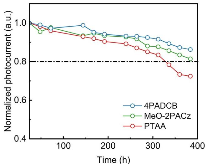
**Figure S9.** The storage stability of unsealed devices with different HTLs under ambient air conditions with a relative humidity of  $25\pm 5\%$ .
