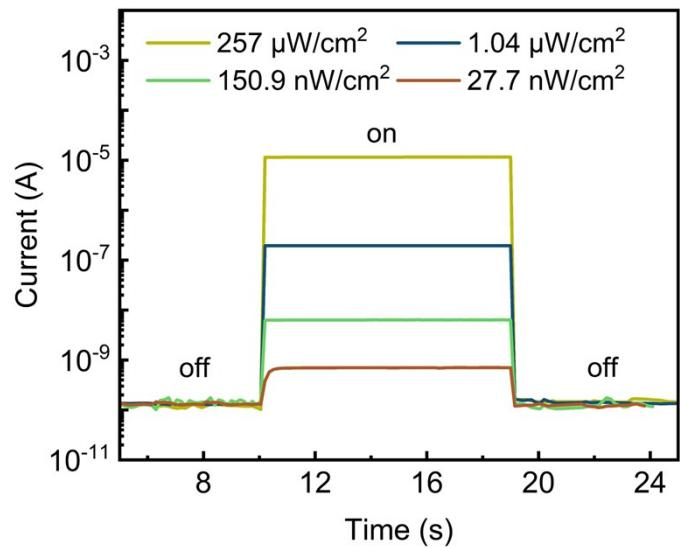
**Figure S7.** The I-T curve under different weak light illuminations at 520 nm.
