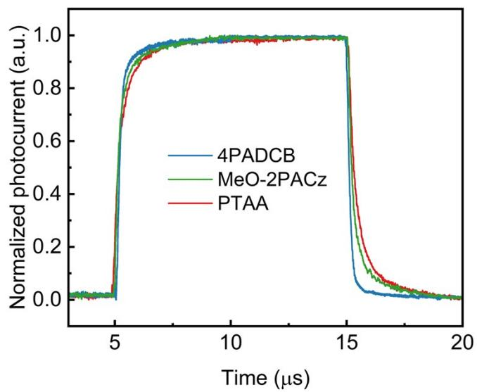
**Figure S5.** The transient response of PPDs based on different HTLs.
