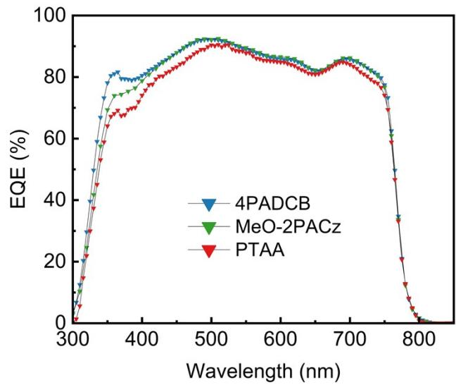
**Figure S4.** The external quantum efficiency (EQE) of PPDs with different HTLs.
