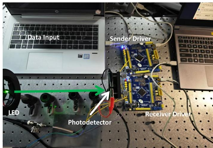
**Figure S10.** Photograph of the visible light communication application based on perovskite photodetectors.
