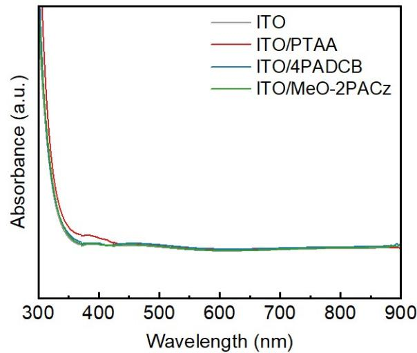
**Figure S1.** UV–vis transmission spectra of bare ITO, PTAA-coated ITO, MeO-2PACz-coated ITO, and 4PADCB-coated ITO substrates.
