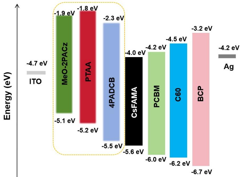
**Figure S2.** Energy-level diagram of the perovskite photodetectors based on different HTLs (4PADCB, MeO-2PACz, and PTAA).
