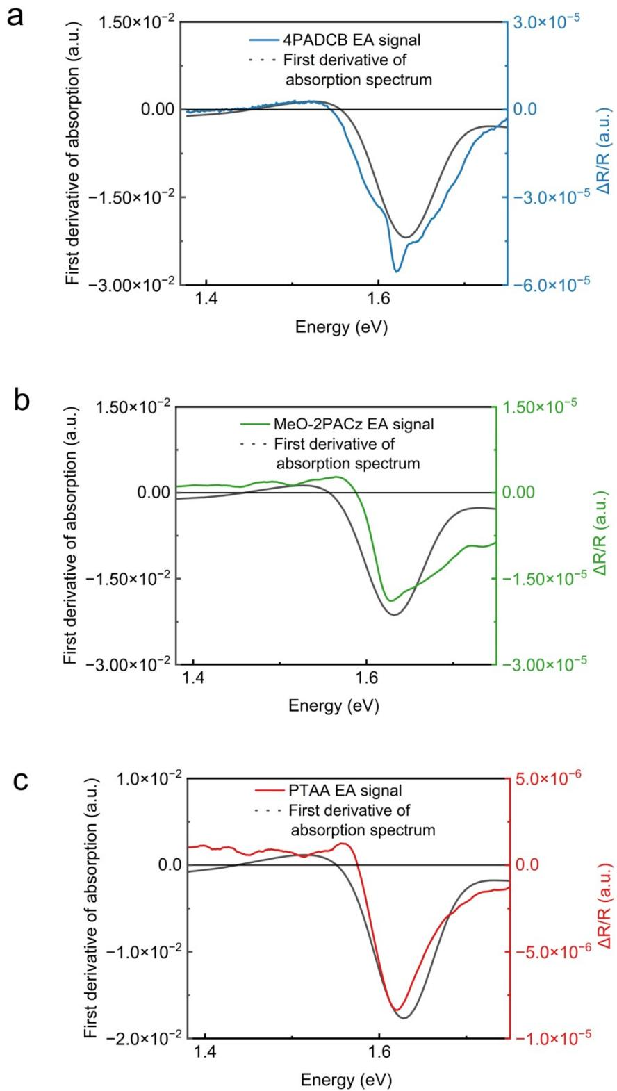
**Figure S6.** EA spectrum and the first derivative of the corresponding light absorption spectrum of the perovskite film deposited on (a)4PADCB, (b)MeO-2PACz and (c) PTAA.
