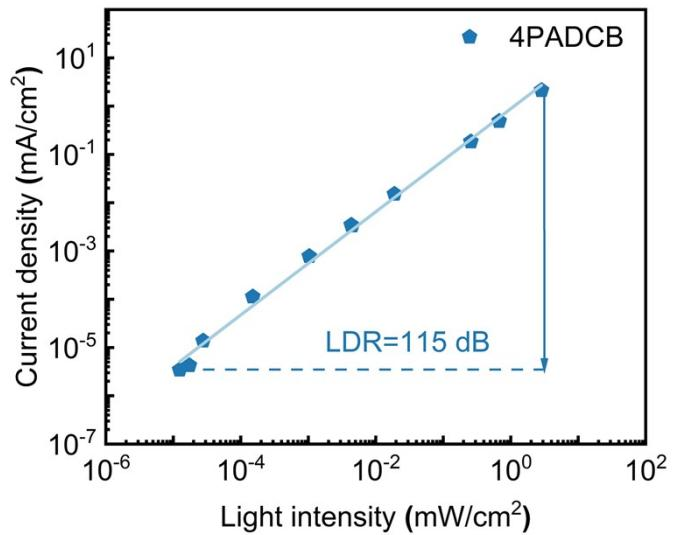
**Figure S8.** Linear dynamic range of 4PADCB-based perovskite photodetectors measured under zero bias voltage and illumination with a 520 nm light source at varying light intensities.
