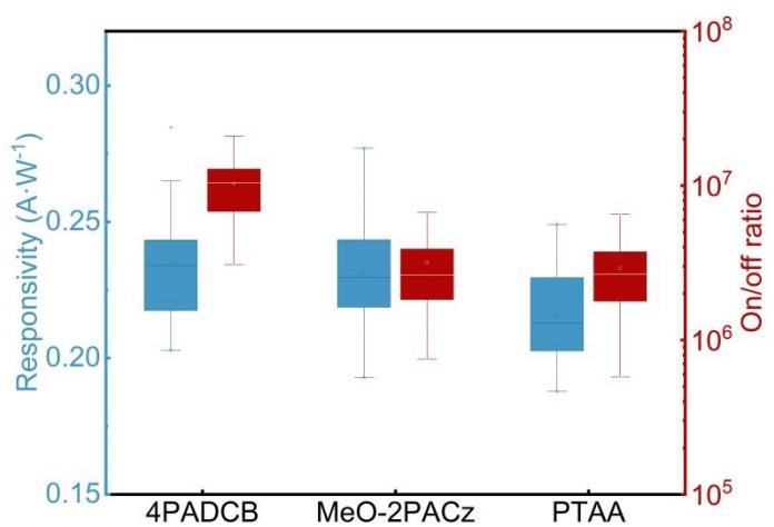
**Figure S3.** The statistical distributions of responsivity, and on/off ratio for perovskite photodetectors (PPDs) with different hole transport layers (HTLs), tested at AM 1.5G solar spectrum condition.
