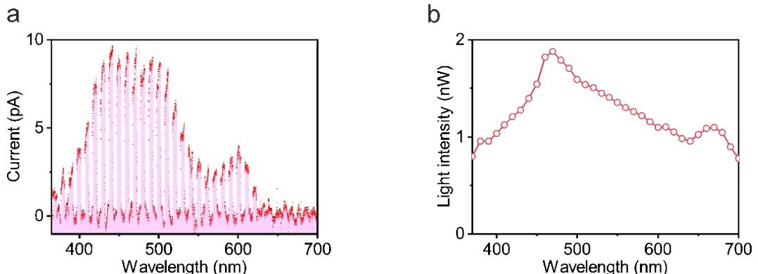
**Figure S12.** (a) Photoresponse curves measured at a 1 V bias under illumination with monochromatric light of progressively increasing wavelengths. (b) Intensity of monochromatric light as a function of wavelength.
