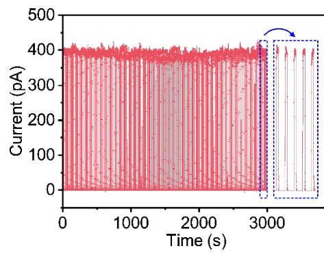
**Figure S15.** Photoresponse curve recorded over 3000 seconds under cyclic illumination at a wavelength of 520 nm.
