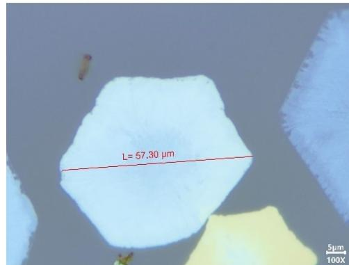
**Figure S3.** Optical image of the SbI<sub>3</sub> thin crystal. The optical image shows that the size of single crystal SbI<sub>3</sub> can reach up to 50 μm.
