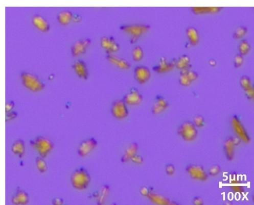
**Figure S2.** Optical images of SbI<sub>3</sub> grown on SiO<sub>2</sub>/Si substrate.
