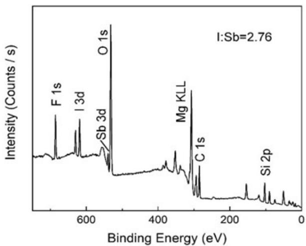
**Figure S6.** X-ray photoelectron spectroscopy (XPS) survey spectra of  $\text{SbI}_3$  on mica.
