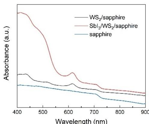
**Figure S13.** The optical absorption spectra of WS<sub>2</sub> and SbI<sub>3</sub>/WS<sub>2</sub> heterostructure on sapphire substrates.
