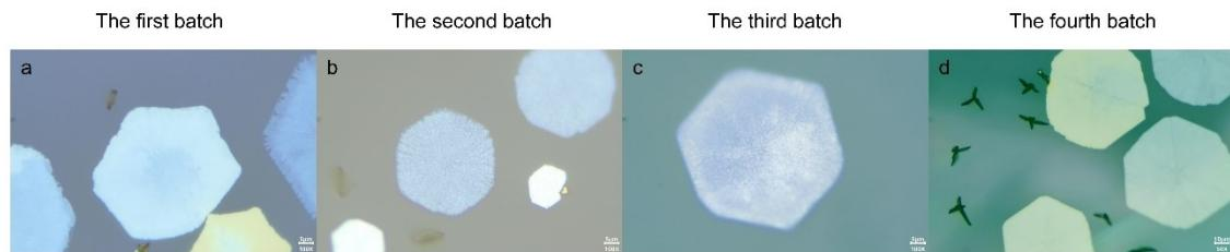
**Figure S4.** Optical images of SbI<sub>3</sub> thin crystals on mica substrates. (a) First batch of the SbI<sub>3</sub> samples. (b) Second batch of the SbI<sub>3</sub> samples. (c) Third batch of the SbI<sub>3</sub> samples. (d) Fourth batch of the SbI<sub>3</sub> samples.
