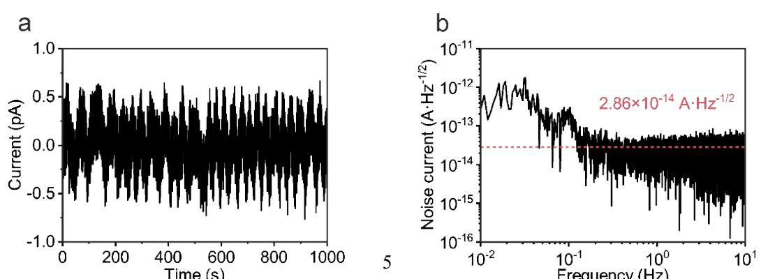
**Figure S14.** (a) Time-resolved dark current of a SbI<sub>3</sub>-modified WS<sub>2</sub> photodetector measured under dark condition at  $V=1$  V and (b) Noise spectral density curve derived from the Fourier transform of the dark current traces, illustrating the frequency-dependent characteristics of the noise signal.
