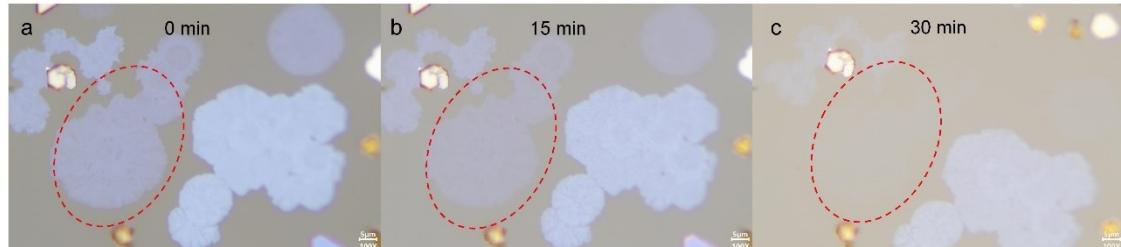
**Figure S5.** Air stability of the sample characterized by optical images. (a) The optical images of the as-prepared sample. (b) The optical images of the sample exposed in air for 15 min. (c) The optical images of the sample exposed in air for 30 min.
