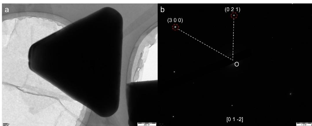
**Figure S7.** (a) Low-magnification TEM image of a  $\text{SbI}_3$  crystal. (b) SAED pattern of  $\text{SbI}_3$ .
