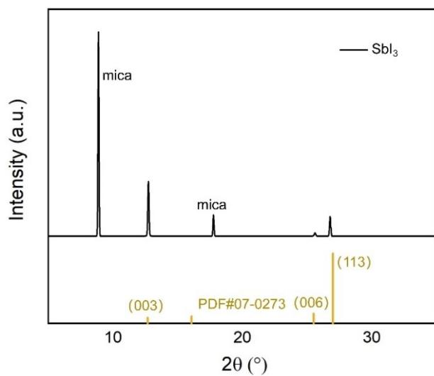
**Figure S8.** X-ray diffraction (XRD) pattern of  $\text{SbI}_3$  on mica.
