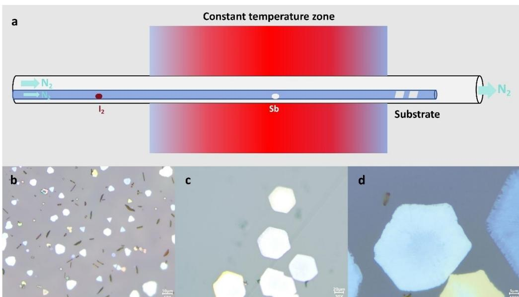
**Figure S1.** Antimony triiodide synthesized on mica substrates. (a) Schematic illustration of an CVD growth setup. (b–d) Optical images of SbI<sub>3</sub> thin crystals grown on mica substrate.
