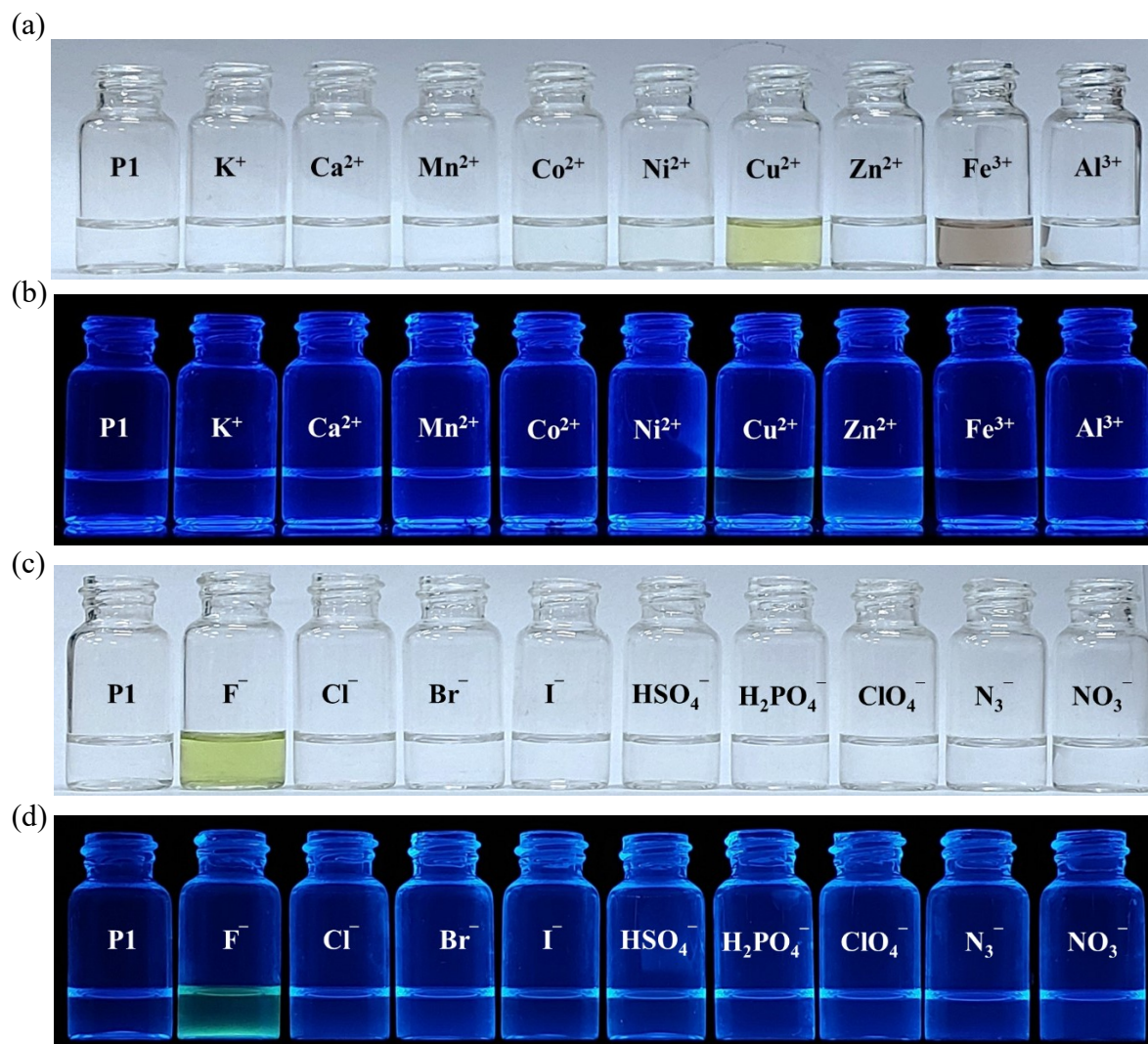
Fig. S7 Visual responses of P1 upon addition of different cations under ambient (a) and UV light (b) conditions, and anions under ambient (c) and UV light (d) conditions, in \text{CH}_3\text{CN}:\text{DMSO} (9:1, v/v; pH 7.1) solution.
