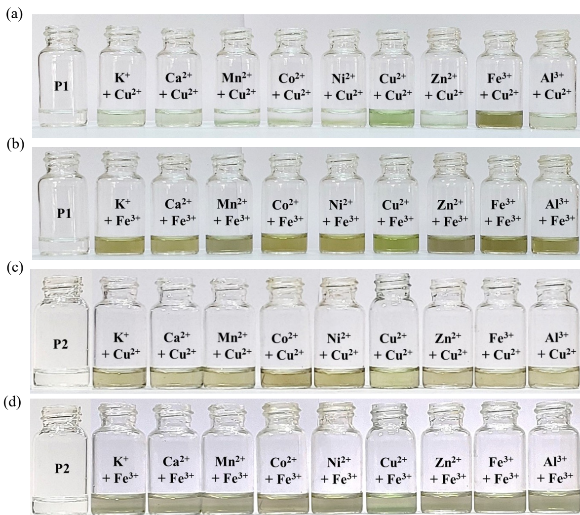
Fig. S8 Visual responses of P1 upon the addition of \text{Cu}^{2+} (a) and \text{Fe}^{3+} (b) cations, and P2 upon the addition of \text{Cu}^{2+} (c) and \text{Fe}^{3+} (d) cations in the presence of various competing metal ions under ambient light condition, in \text{CH}_3\text{CN}:\text{DMSO} (9:1, v/v; pH 7.1) solution.
