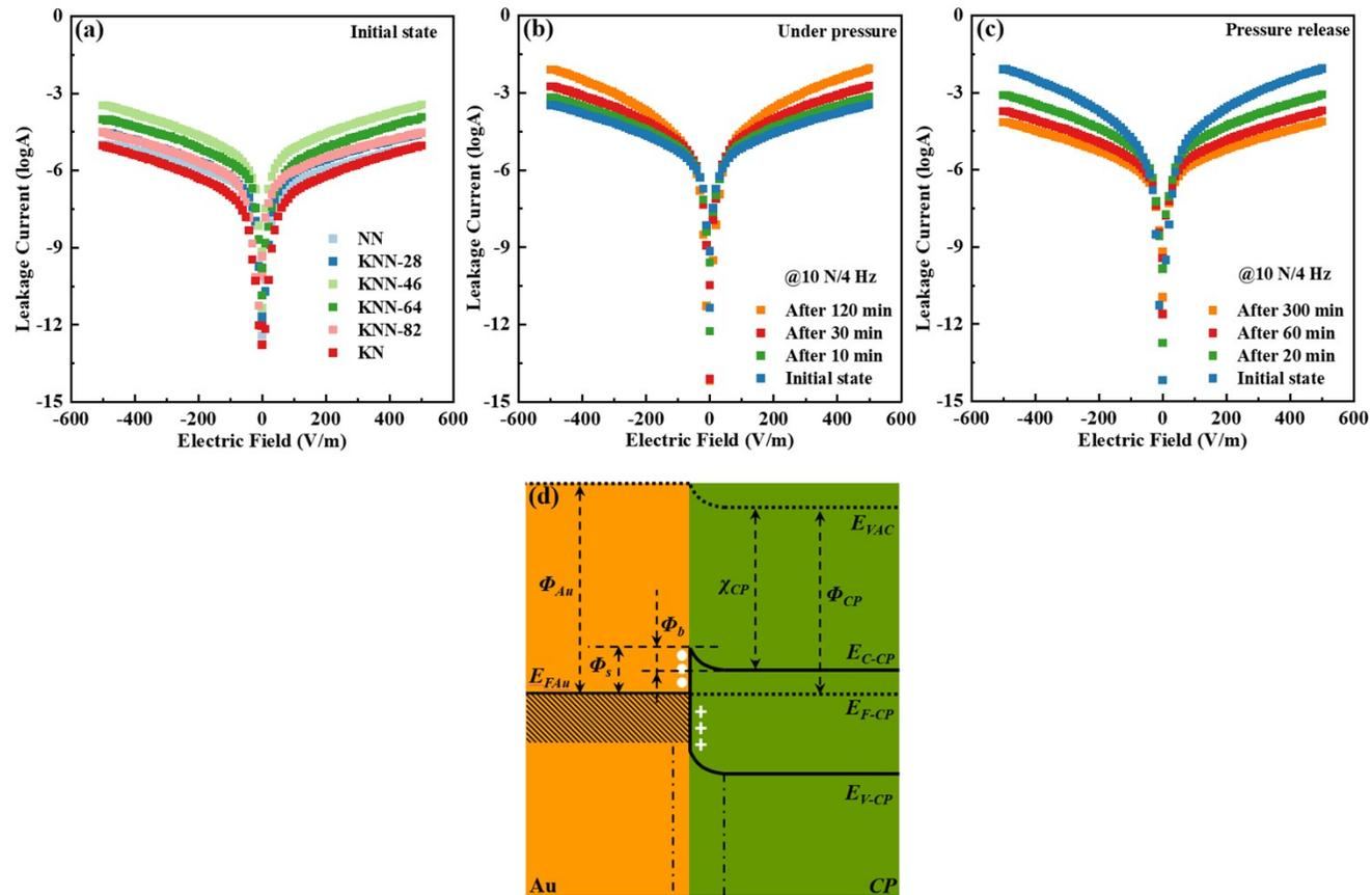
Figure S3 (a) the I-V curves of all the C8P2-KNN films with different KNN components; (b) the I-V curves of the C8P2-KNN46 film under a mechanical load of 10 N at 4 Hz for different durations; (c) the I-V curves of the C8P2-KNN46 film at different durations after pressure release; (d) the band diagram of the interface between the Au electrode and the pristine C8P2 film.
