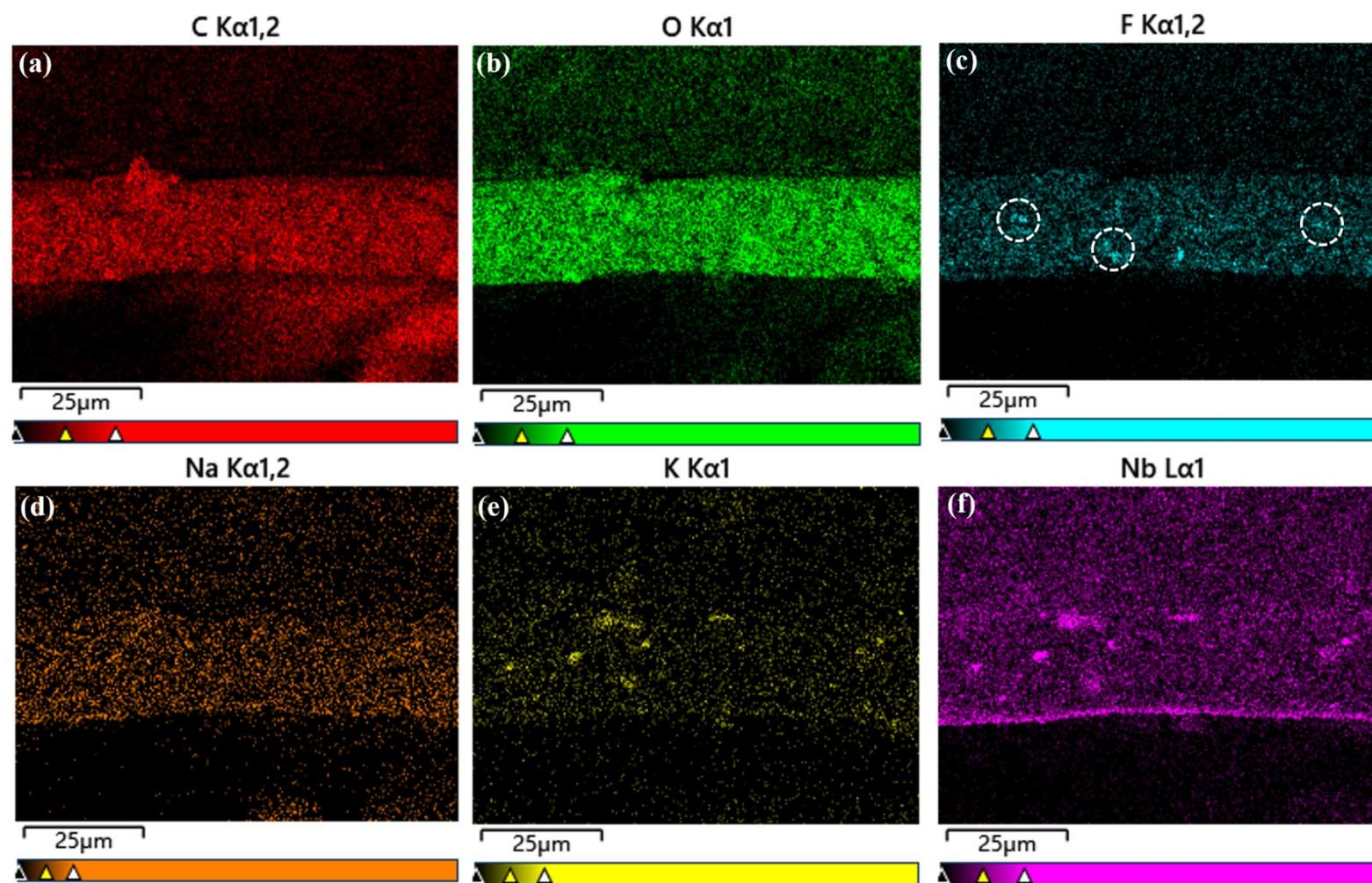
Figure S1 The energy dispersive spectroscopy (EDS) mappings for the C, O, F, Na, K, and Nb elements of Figure 3(a).
