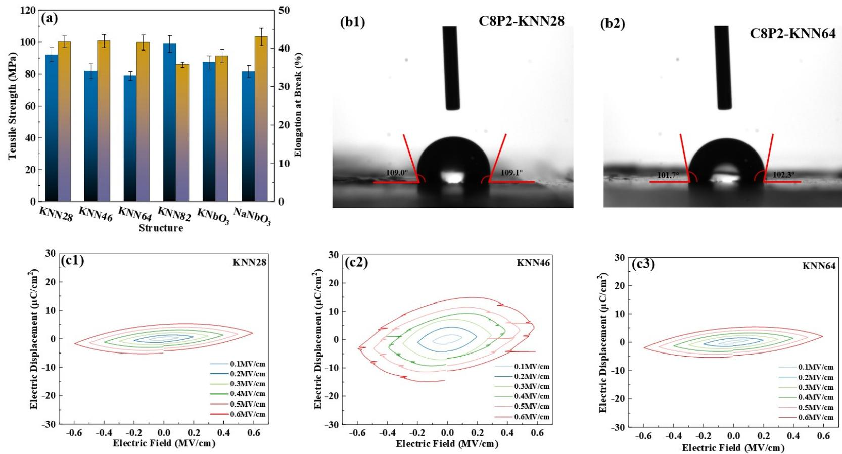
Figure S4(a) the tensile strength and elongation at break of all C8P2-KNN films; The image of the water contact angle of the (b1) C8P2-KNN28; (b2) C8P2-KNN64; the polarization-electric field relationships for the (c1) KNN28, (c2) KNN46, (c3) KNN64 films under different fields.
