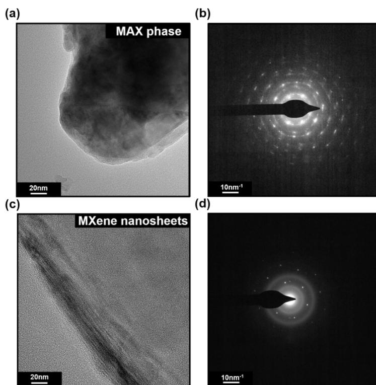
**Figure S3.** (a) TEM image and (b) corresponding SAED pattern of the MAX phase, (c) TEM image and (d) SAED pattern of MXene nanosheets.
