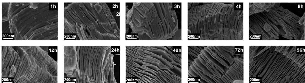
**Figure S1.** SEM images of  $\text{Ti}_3\text{AlC}_2$  samples etched for different durations (1 h to 96 h), illustrating the progressive delamination and morphological evolution from the MAX phase to MXene nanosheets.
