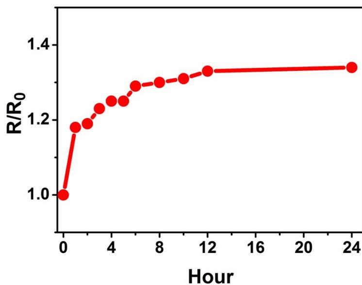
**Figure S4.** Normalized resistance ( $R/R_0$ ) of the MXene/PVDF electrode (7:1 weight ratio) during thermal aging at 80 °C over a 24-hour period.
