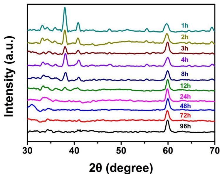
**Figure S2.** XRD patterns of  $\text{Ti}_3\text{AlC}_2$  samples etched for varying durations, showing the gradual disappearance of MAX phase peaks and the corresponding formation of MXene, highlighting the effect of etching time on phase conversion.
