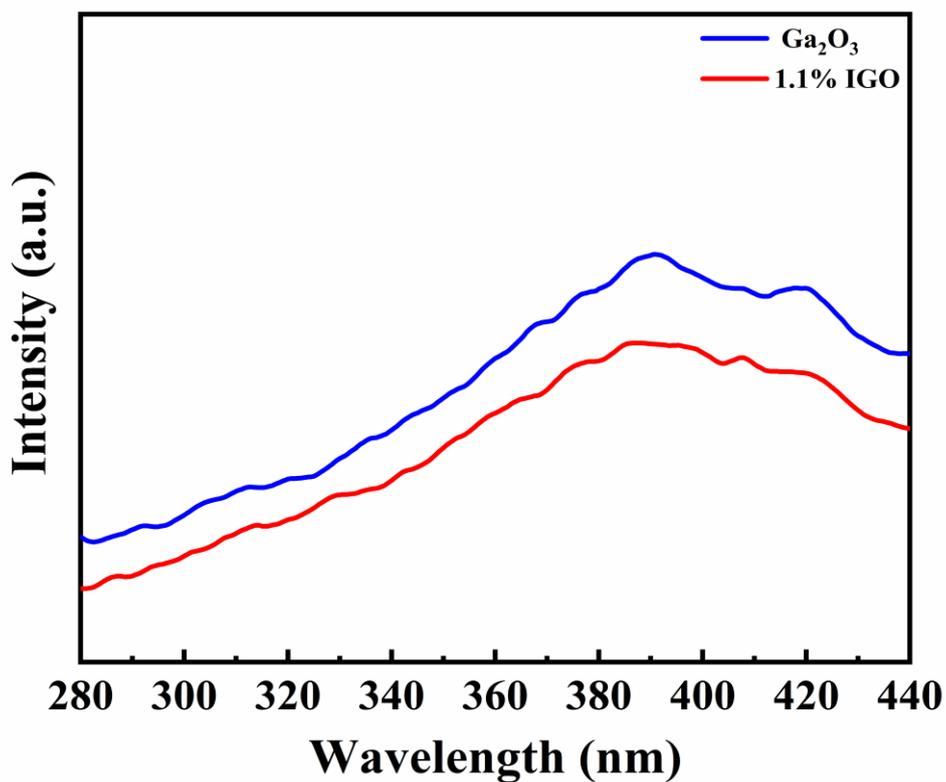
**Fig. S5.** Steady-state PL spectra of the undoped sample and that with the optimal concentration doping.
