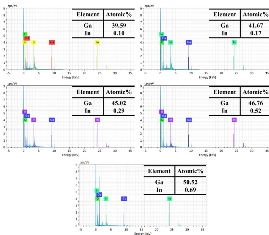
**Fig. S3.** The element content analysis of top-down SEM images with different concentration gradients of In-doping.
