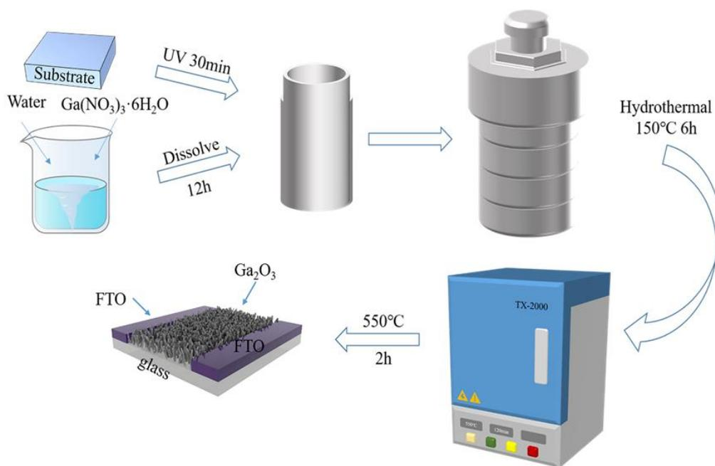
**Fig. S1.** Schematic diagram of IGO nanorods made by hydrothermal method.
