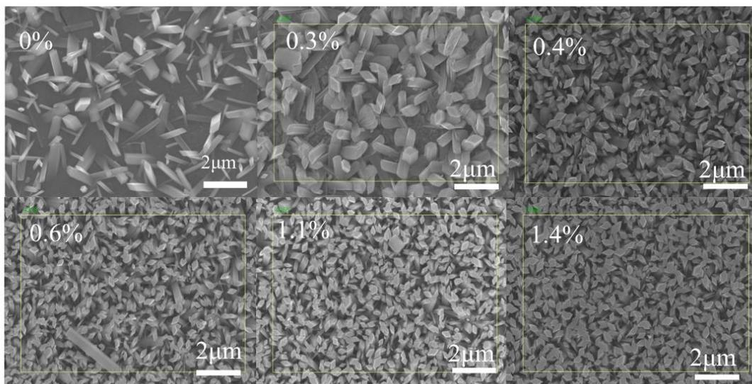
**Fig. S2.** Top-down SEM images with different concentration gradients of In-doping.
