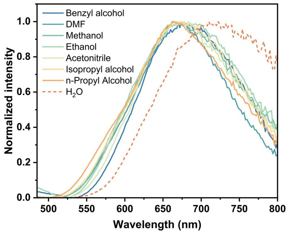
**Figure S10.** PL spectra of **CuI-MOF-H** after 3 days of water, methanol, ethanol, n-propyl alcohol, isopropyl alcohol, DMF, benzyl alcohol and acetonitrile immersion.
