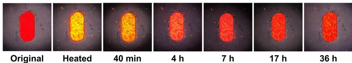
**Figure S7.** Photos of CuI-MOF-H under 365nm UV light at different times (room temperature, 54%RH).
