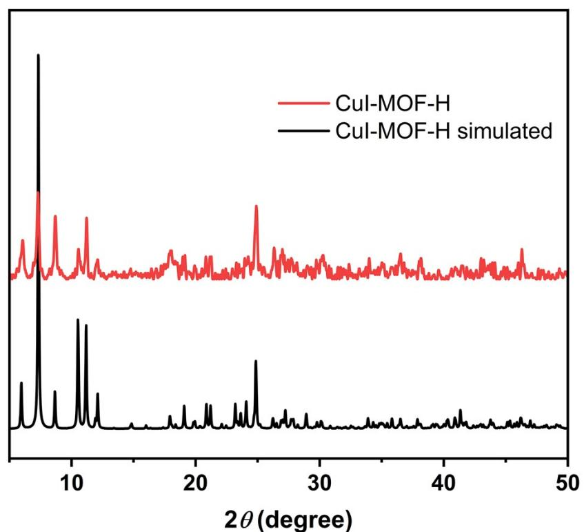
**Figure S6.** The experimental and simulated PXRD patterns of **CuI-MOF-H**.
