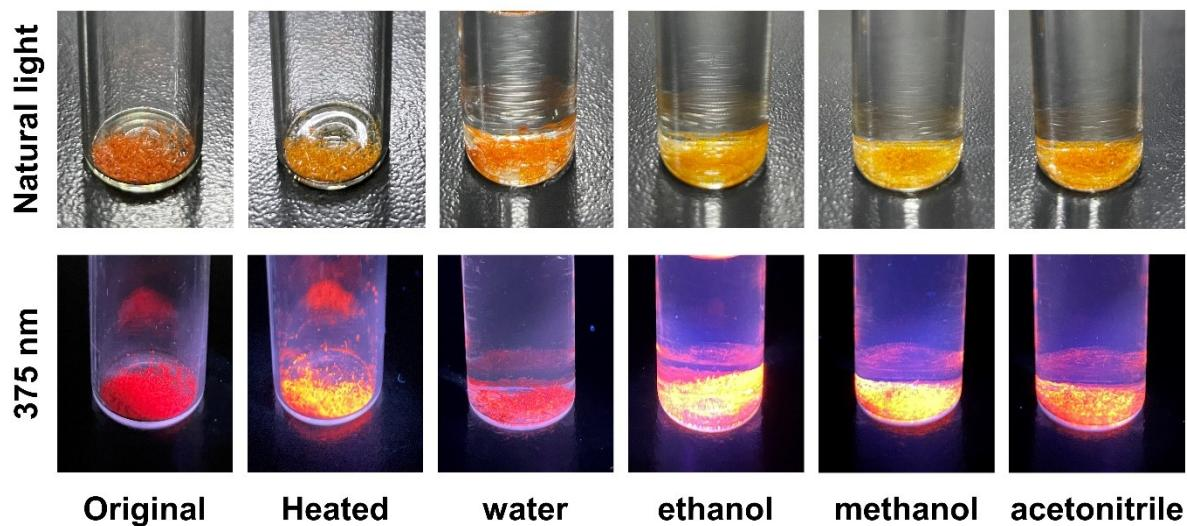
**Figure S9.** Photos of **CuI-MOF-H** after 3 days of water, anhydrous ethanol, methanol, and acetonitrile immersion.
