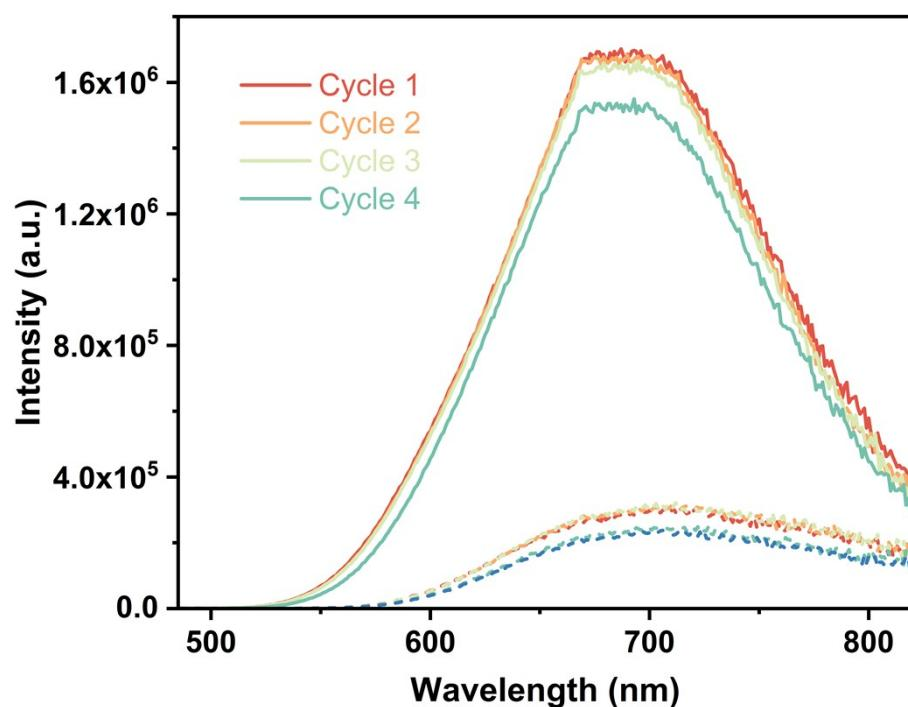
**Figure S8.** Recycle tests of CuI-MOF and CuI-MOF-H for four runs.
