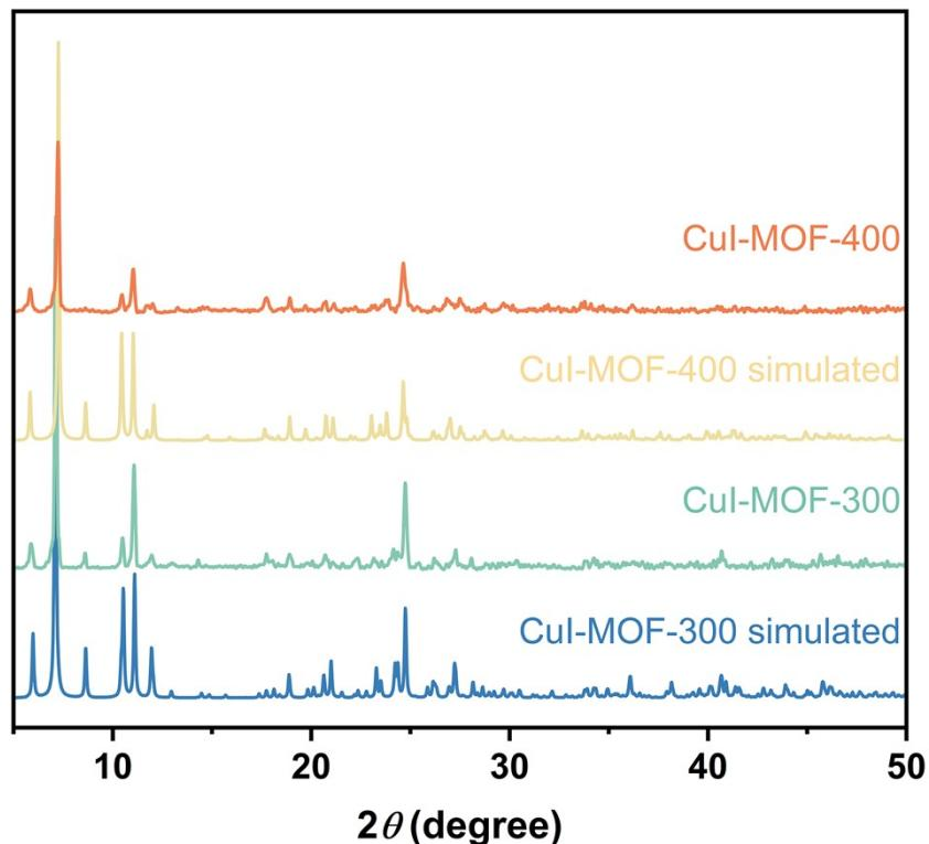
**Figure S2.** The experimental and simulated PXRD patterns of CuI-MOF-300 and CuI-MOF-400.
