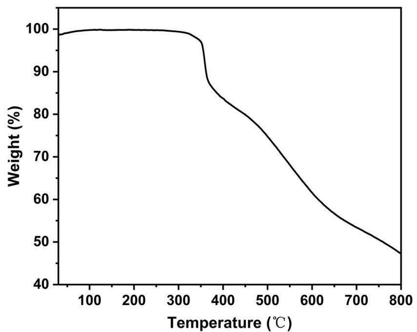
**Figure S5.** The TGA curve of **CuI-MOF-H**.
