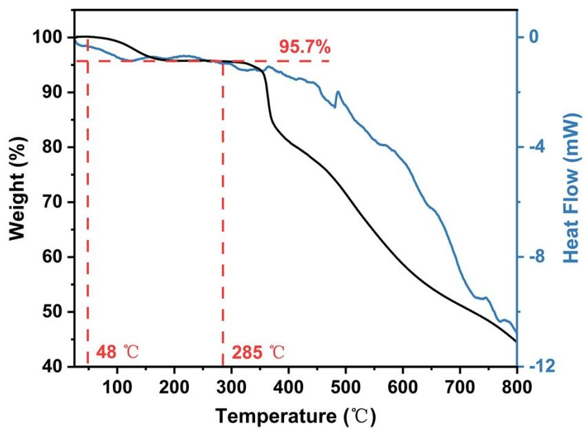
**Figure S3.** The TGA and DSC curves of **CuI-MOF**.
