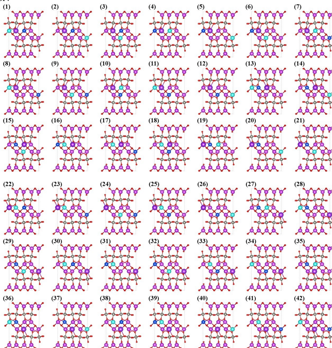
Fig. S2 Structures of \text{K}^+ , \text{Ho}^{3+} , and \text{Yb}^{3+} -codoped \text{Bi}_2\text{WO}_6 with \text{Bi}^{3+} substitution
