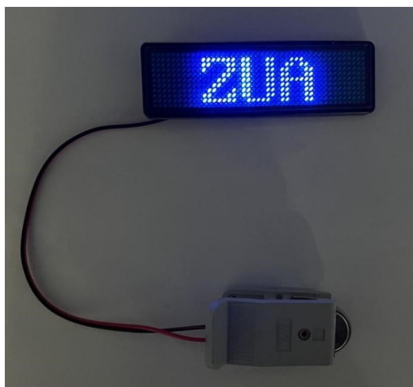
Fig. S18 Two NMO@NCS//AC ASC devices connected in series light up the "ZUA" blue LED display.
