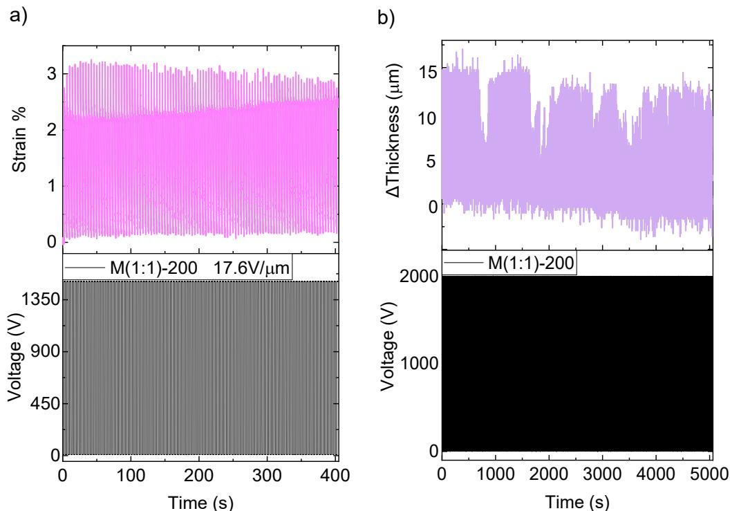
**Fig. S22** Cyclic actuation test of a single layer **M(1:1)-200** for 100 cycles at  $17.6 \text{ V } \mu\text{m}^{-1}$  (1500 V) at 0.25 Hz (a), and stack actuator with five active layers with a thickness of  $\sim 145 \mu\text{m}$  at an electric field of  $13.8 \text{ V } \mu\text{m}^{-1}$  (2000 V) for more than 1000 cycles.
