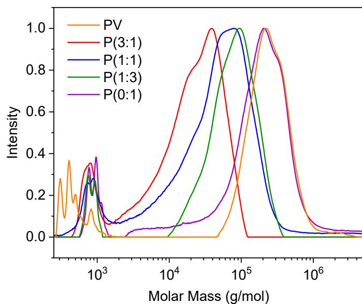
**Fig. S2** GPC elugrams of the polymers PV, P(3:1), P(1:1), P(1:3), P(0:1). The polymer (PV) was synthesized through anionic ring-opening polymerization of 1,3,5,7-tetravinyl-1,3,5,7-tetramethylcyclotetrasiloxane using TMAH as the initiator. The PV contains a small amount of cycles which are difficult to remove by precipitation or distillation. GPC elugram of the P(1:0) could not be recorded as it is insoluble in THF.
