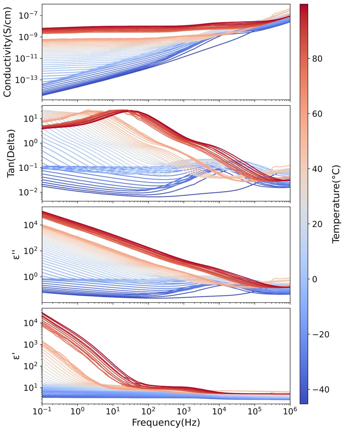
**Fig. S8** The conductivity ( $\sigma'$ ), loss tangent ( $\tan(\delta)$ ), dielectric loss ( $\epsilon''$ ), and dielectric permittivity ( $\epsilon'$ ) analysis at altering temperature as a function of frequency ranging from  $10^{-1}$  and  $10^6$  Hz for M(3:1).
