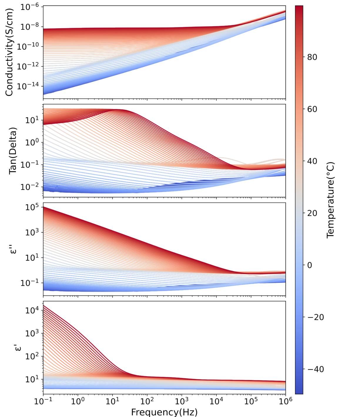
**Fig. S7** The conductivity ( $\sigma'$ ), loss tangent ( $\tan(\delta)$ ), dielectric loss ( $\epsilon''$ ), and dielectric permittivity ( $\epsilon'$ ) analysis at altering temperature as a function of frequency ranging from  $10^{-1}$  and  $10^6$  Hz for M(1:0).
