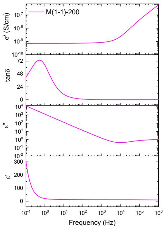
**Fig. S21** Impedance spectroscopy at room temperature and different frequencies of **M(1:1)-200**.
