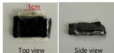
**Fig. 23** Photo of the stack actuator constructed by layering an interdigitated structure composed of alternating 5 dielectric films ( $145 \mu\text{m}$  thick and a size of  $1 \times 1.5 \text{ cm}$ ) and 6 electrode layers ( $205 \mu\text{m}$  thick and a size of  $1 \times 1.5 \text{ cm}$ ).
