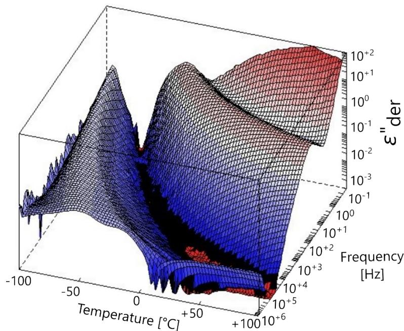
**Fig. S12** 3D plot of conduction-free  $\epsilon''_{\text{der}}$  curves of a **M(0:1)** as a function of frequency from  $10^{-1}$  to  $10^6$  Hz and temperatures from -100 to +100  $^{\circ}\text{C}$ .
