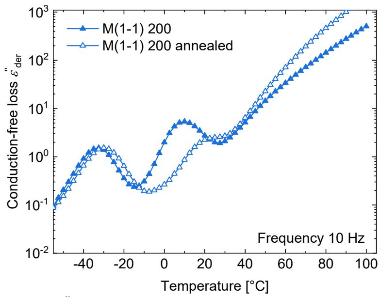
**Fig. S17**  $\varepsilon_{der}''$  curves of a **M(1-1)-200** as a function of temperature at a frequency of 10 Hz before and after annealing
