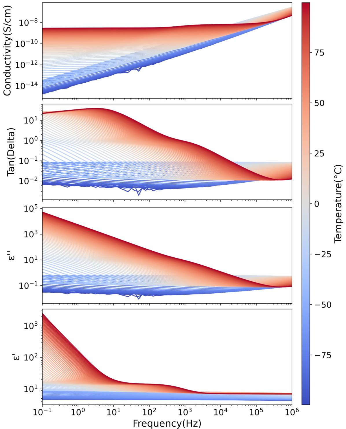
**Fig. S10** The conductivity ( $\sigma'$ ), loss tangent ( $\tan(\delta)$ ), dielectric loss ( $\epsilon''$ ), and dielectric permittivity ( $\epsilon'$ ) analysis at altering temperature as a function of frequency ranging from  $10^{-1}$  and  $10^6$  Hz for M(1:3).
