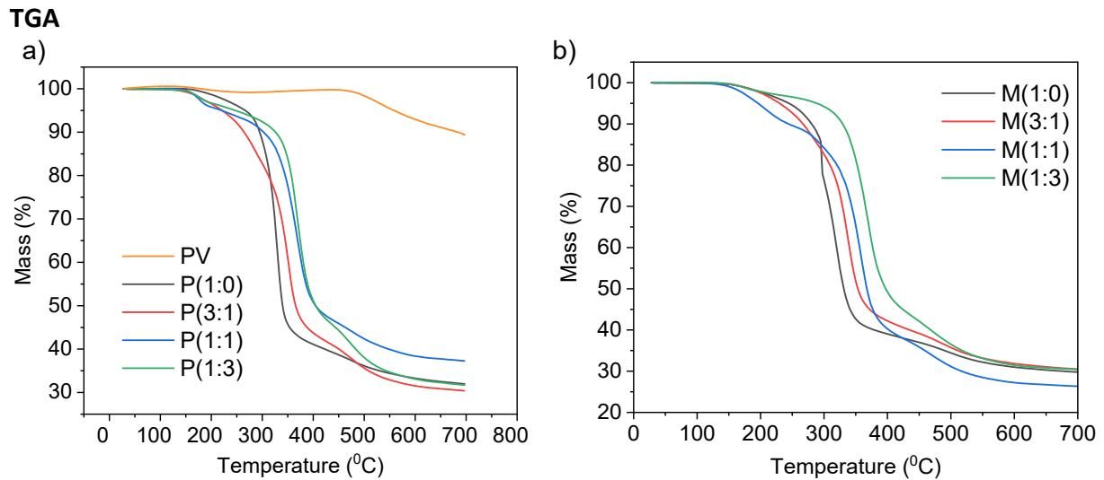
**Fig. S5** TGA of the polymers **P(x:y)** (a), and materials **M(x:y)** (b)
