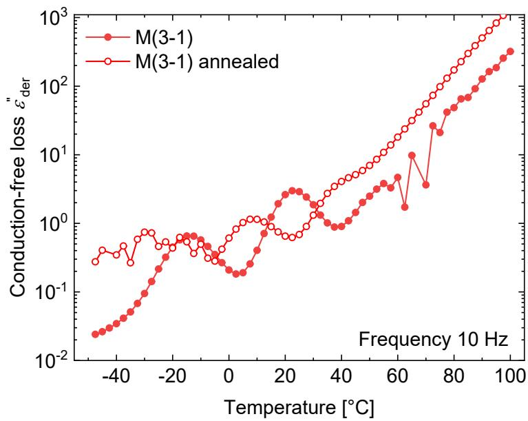
**Fig. S16**  $\varepsilon_{der}''$  curves of a **M(3-1)** as a function of temperature at a frequency of 10 Hz before and after annealing.
