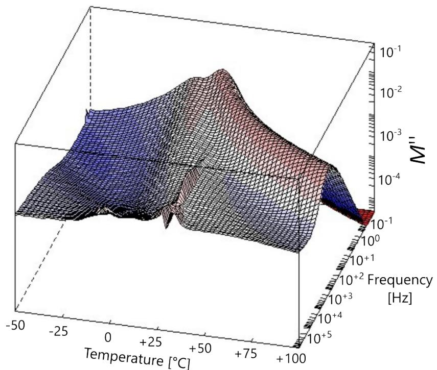
**Fig. S11** 3D plot of electric loss modulus  $M''$  of **M(1-0)**.
