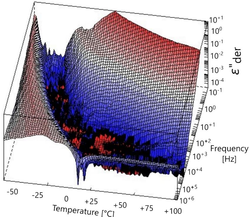
**Fig. S14** 3D plot of conduction-free  $\epsilon''_{\text{der}}$  curves of a butane thiol functionalized V<sub>4</sub> (tetravinyltetramethylcyclotetrasiloxane) sample as a function of frequency from  $10^{-1}$  to  $10^6$  Hz and temperatures from -100 to +100 °C.
