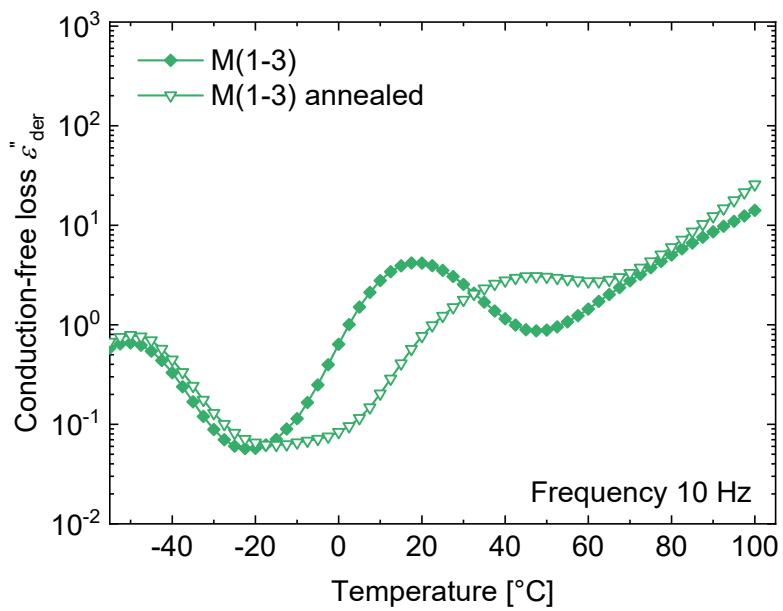
**Fig. S18**  $\varepsilon_{der}''$  curves of a **M(1-3)** as a function of temperature at a frequency of 10 Hz before and after annealing.
