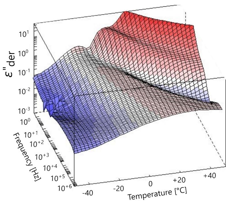
**Fig. S13** 3D plot of conduction-free  $\epsilon''_{\text{der}}$  curves of a 3-mercaptosulfolane functionalized V<sub>4</sub> (tetravinyltetramethylcyclotetrasiloxane) sample as a function of frequency from  $10^{-1}$  to  $10^6$  Hz and temperatures from -100 to +100 °C.
