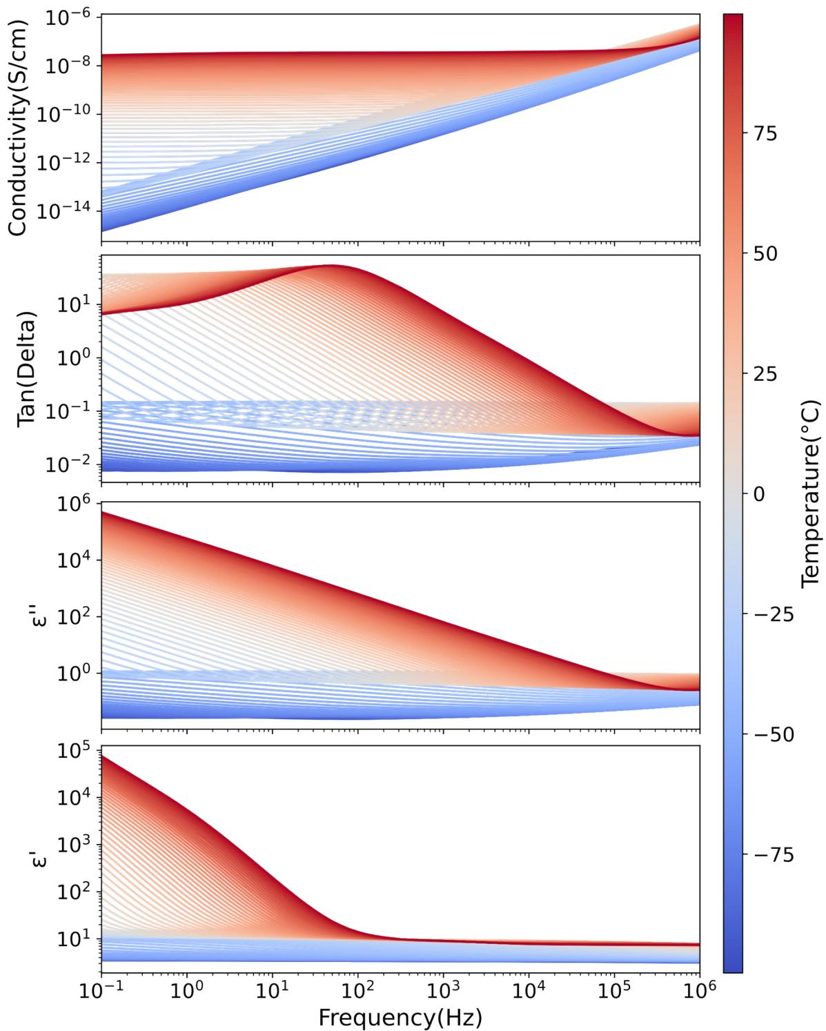
**Fig.S9** The conductivity ( $\sigma'$ ), loss tangent ( $\tan(\delta)$ ), dielectric loss ( $\epsilon''$ ), and dielectric permittivity ( $\epsilon'$ ) analysis at altering temperature as a function of frequency ranging from  $10^{-1}$  and  $10^6$  Hz for M(1:1).
