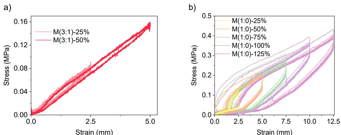
**Fig. S6** Uniaxial cyclic test of **M(3:1)** at 25 %, 50 % strain for 10 cycles (a) and of **M(1:0)** at 25 %, 50 %, 75 %, 100 %, 125 % strain for 10 cycles (b).
