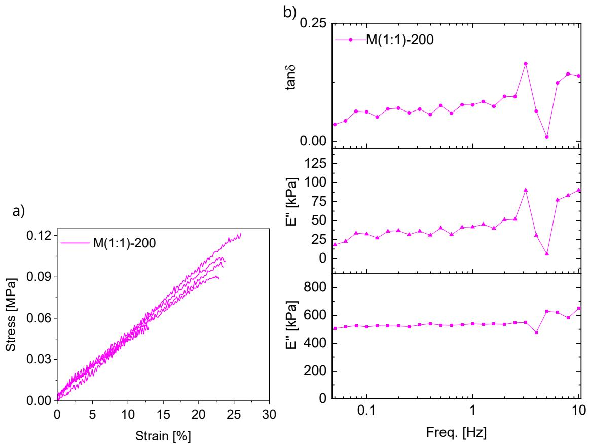
**Fig.S20** Tensile test (a) and DMA (b) of **M(1:1)-200**.
