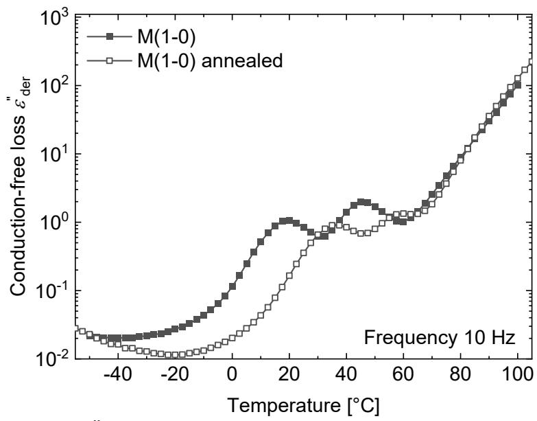
**Fig. S15**  $\varepsilon_{der}''$  curves of a **M(1-0)** as a function of temperature at a frequency of 10 Hz before and after annealing.
