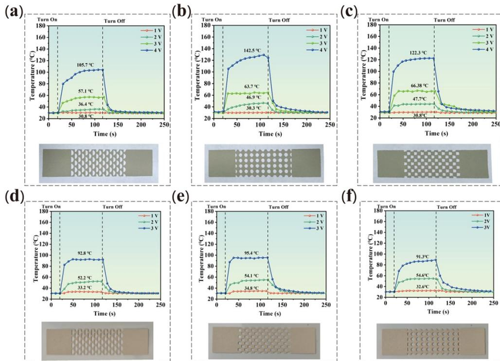
**Figure S3** Heating performances of Paper-based (a-c) and PET-based PFHs (d-f) prepared when the printed patterns are semicircular, circular, and square shape.
