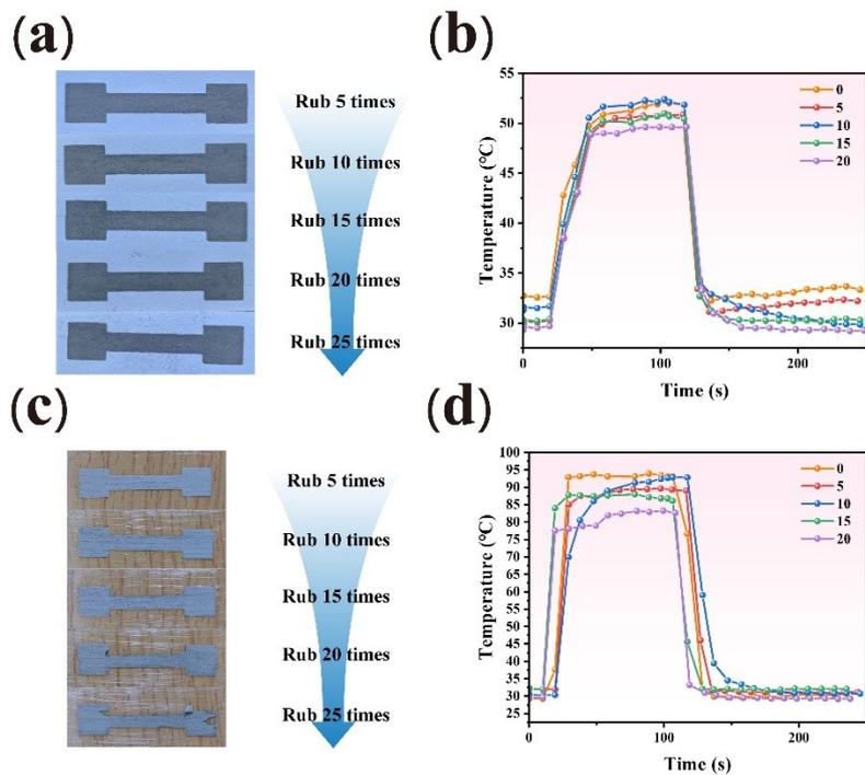
**Figure S5** Photos (a) and temperature response curves (b) of the sample printed on the paper substrate being sanded for different times (5, 10, 15, 20 and 25 times) using sandpaper; and photos (c) and temperature response curves (d) of the sample printed on the PET substrate being sanded for different times (5, 10, 15, 20 and 25 times) using sandpaper.
