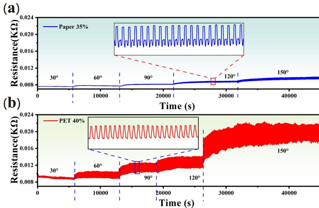
**Figure S4** (a) Electrical properties of paper-based FPHs (a) and PET-based FPHs (b) during 500 consecutive bending tests at different angles of 30°, 60°, 90°, 120° and 150°.
