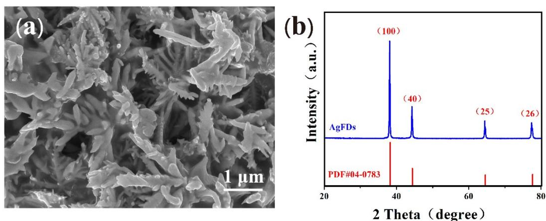
**Figure S1** The SEM image (a) and XRD pattern (b) of printed layer of Ag FDs-based conductive ink.
