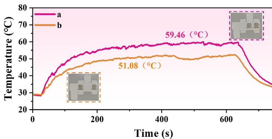
**Figure S7** Temperature response curve of heating units that printed on adjacent (a) and non-adjacent sides (b).
