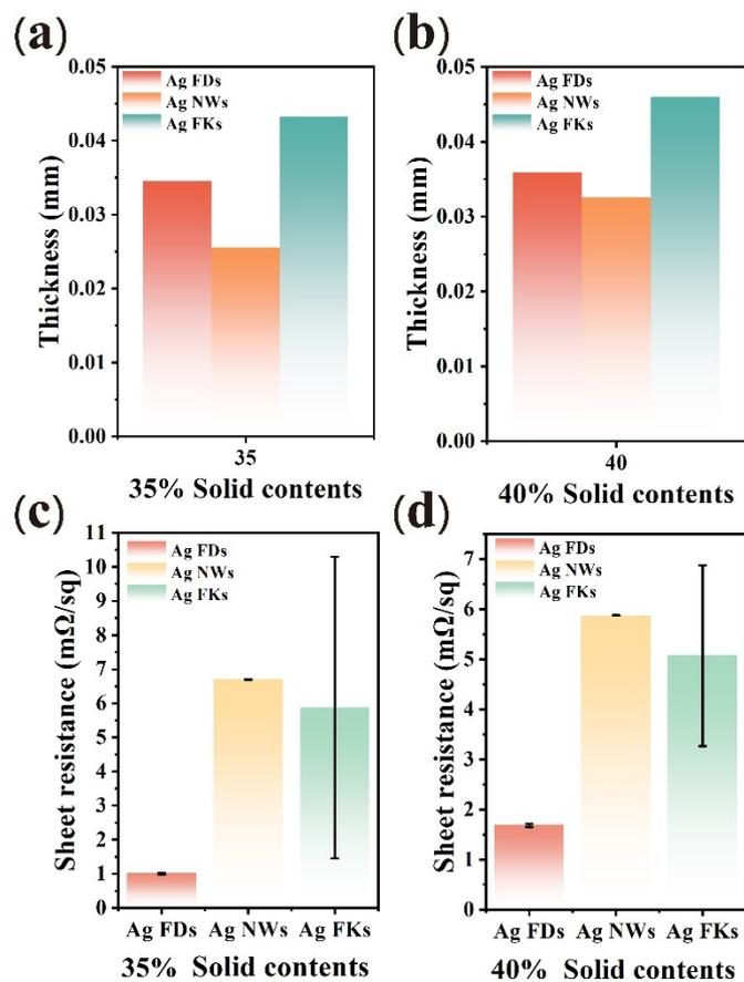
**Figure S2** Ink thickness of different Ag nanomaterials (Ag FDs, Ag NWs and Ag FKs)-based inks on paper substrate (a) and PET substrate (b) after printing 3 times. Sheet resistance of Ag nanomaterials (Ag FDs, Ag NWs and Ag FKs)-based inks on paper substrate (c) and PET substrate (d).
