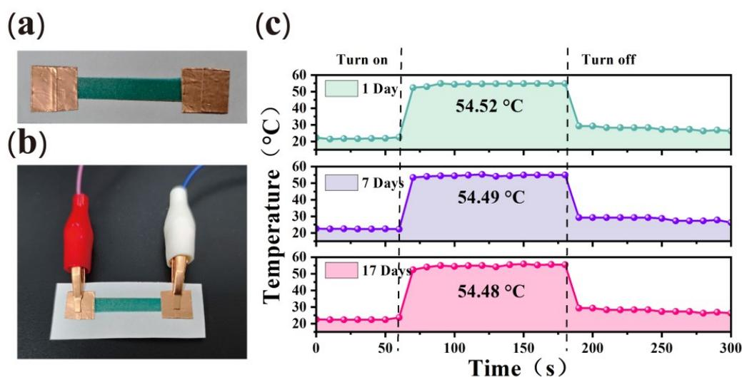
**Fig. S6** The long-term heating stability and heating performance of the paper-based
