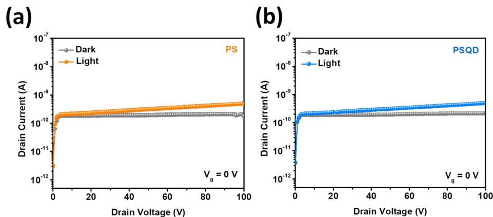
**Figure S10.** Output characteristics of phototransistors based on (a) PS and (b) PSQD. The  $V_d$  was swept from 0 to 100 V in the absence of a gate bias ( $V_g = 0$  V) under 405-nm illumination ( $16.96 \text{ mW cm}^{-2}$ ).
