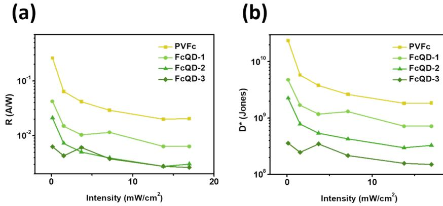
**Figure S7.** (a) Photoresponsivity and (b) specific detectivity of PVFc and CD@QD-PVFc photodetectors measured under various light intensities. The device parameters were determined from the temporal current characteristics at  $V_d = 100$  V and  $V_g = 0$  V.
