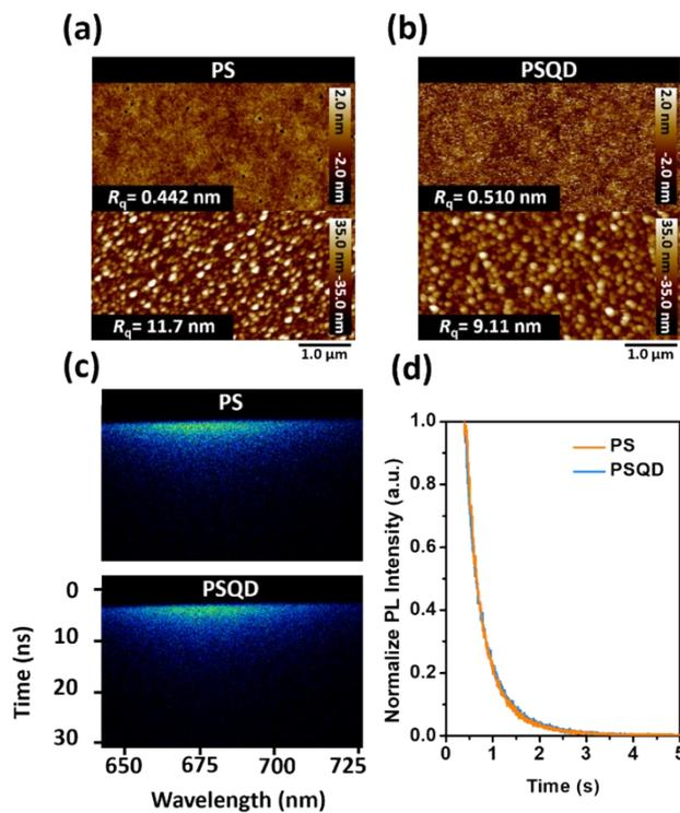
**Figure S9.** (a,b) AFM height images of PS and PSQD films. The lower part of each image shows the topography after thermal evaporation of BPE-PDI. (c) TR-PL 2D contour plots and (d) the corresponding 1D decay profiles of the bilayered films (polymer/BPE-PDI) under 375-nm laser excitation.
