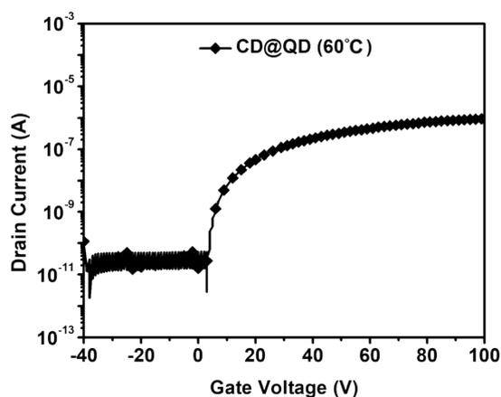
**Figure S5.** Transfer characteristics of the CD@QD phototransistor after thermal treatment at  $60 \text{ }^\circ\text{C}$ . The drain current was measured under dark conditions at  $V_d = 100$  V.
