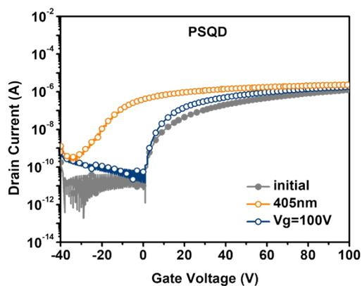
**Figure S11.** Transfer characteristics of the phototransistor device based on the PSQD hybrid film. The drain current was measured at  $V_d = 100$  V. The photowriting was performed under 405 nm illumination ( $16.96 \text{ mW cm}^{-2}$ ), and the electrical erasure was achieved by applying  $V_g = 100$  V for 1 s at  $V_d = 0$  V.
