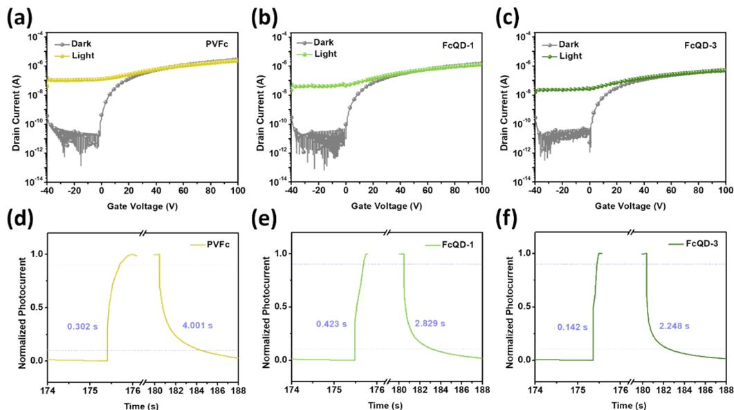
**Figure S4.** (a–c) Transfer curves and (d–f) transient response of the phototransistor detectors comprising (a,d) PVFc, (b,e) FcQD-1, and (c,f) FcQD-3. The transfer curves characteristics were measured in the dark and under light illumination. The measurements were conducted at a fixed  $V_d = 100$  V with a 405 nm light ( $16.96 \text{ mW cm}^{-2}$ ).
