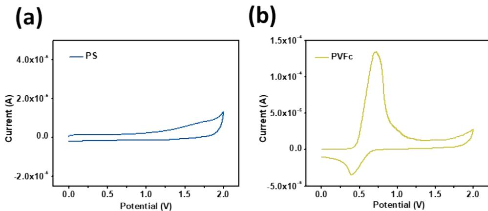
**Figure S2.** Cyclic voltammetry profiles of PS and PVFc polymers measured using an Ag/AgCl reference electrode, a Pt auxiliary electrode, and an ITO glass working electrode coated with the studied materials.
