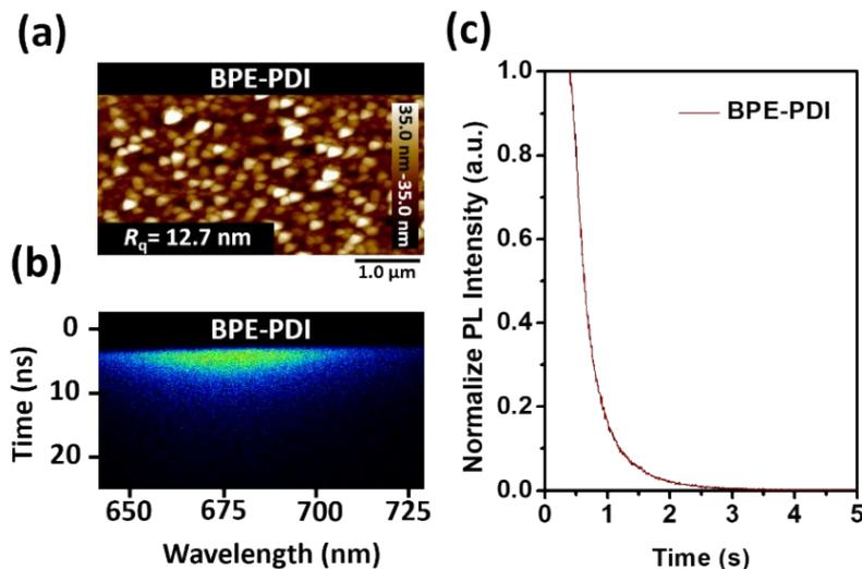
**Figure S3.** (a) AFM height images of BPE-PDI. (b) TR-PL 2D contour plots and (c) the corresponding 1D decay profiles of the BPE-PDI film under 375-nm laser excitation.
