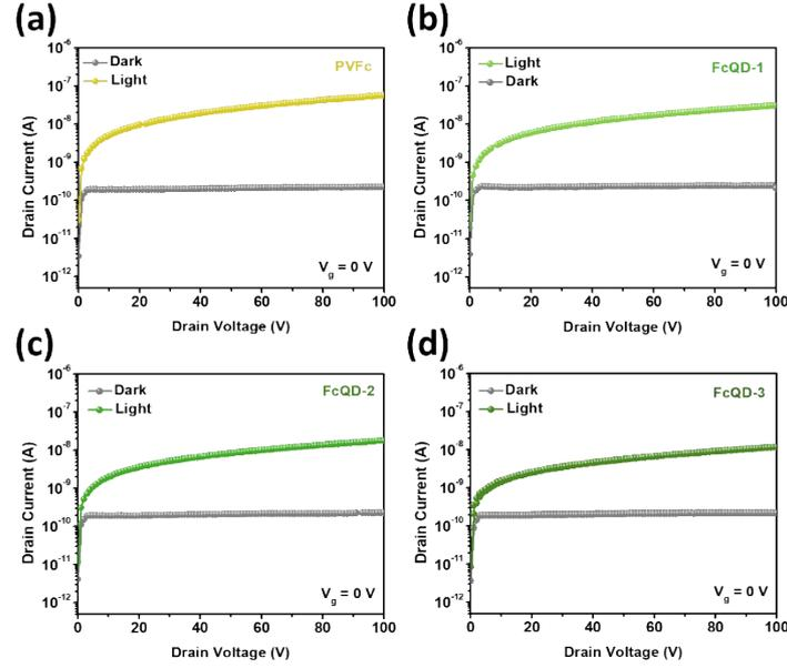
**Figure S6.** Output characteristics of the phototransistors based on (a) PVFc, (b) FcQD-1, (c) FcQD-2, and (d) FcQD-3. The  $V_d$  was swept from 0 to 100 V in the absence of a gate bias ( $V_g = 0$  V) under 405-nm illumination ( $16.96 \text{ mW cm}^{-2}$ ).
