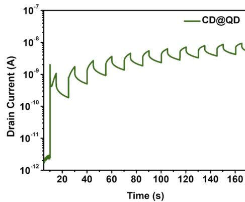
**Figure S8.** The endurance test of the CD@QD phototransistor, consisting of 10 cycles with 5 s of irradiation followed by 10 s of dark conditions. Note that the operating parameters in this test are  $V_d = 100$  V and 405-nm light ( $16.96 \text{ mW cm}^{-2}$ ).
