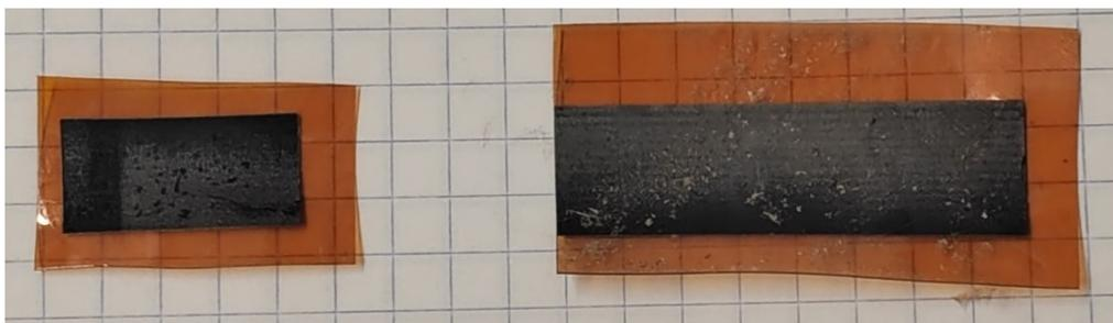
**Fig. S1** Aging changes of LIG films at room temperature. The left picture is LIG film. The right picture shows the LIG film being retained at room temperature for 240 days.
