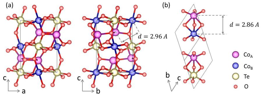
FIG. S2: The optimized unit cells of  $\text{Co}_3\text{TeO}_6$  in (a)  $P2_1/n$  and (b)  $R3$  (with cell volumes  $V = 202$  and  $101 \text{ \AA}^3$ , respectively), with the minimum distance between  $\text{Co}_A$  and  $\text{Co}_B$  indicated.
