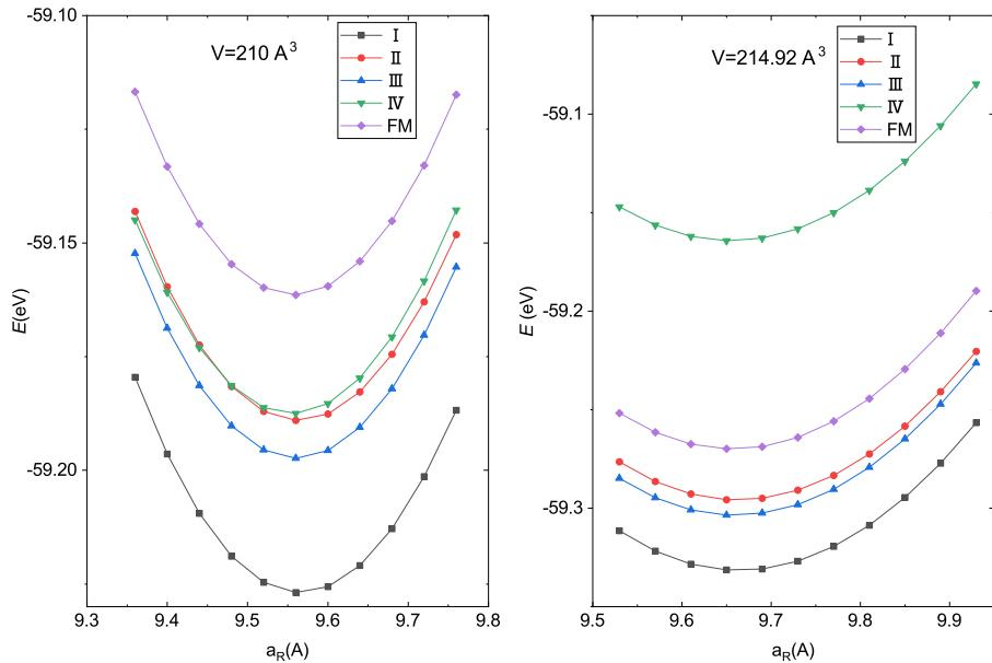
FIG. S4: The variation of total energies of  $\text{Co}_3\text{TeO}_6$  in *R*3 phase with lattice constant  $a_R$  in different magnetic structures. The volume of the unit cell is fixed at (a)  $V = 210 \text{ \AA}^3$  and (b)  $V = 214.92 \text{ \AA}^3$ , respectively.
