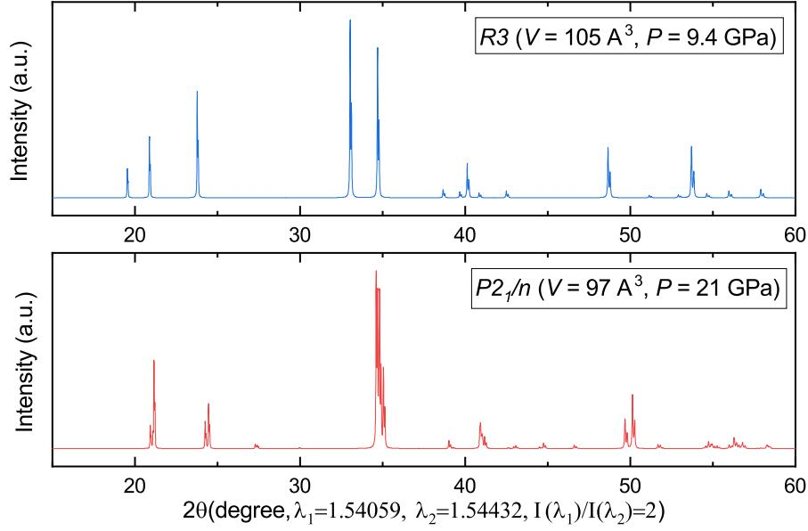
FIG. S3: The simulated X-ray powder diffraction patterns of  $\text{Co}_3\text{TeO}_6$  in *R*3 and  $P2_1/n$ , respectively, by VESTA<sup>8</sup>.
