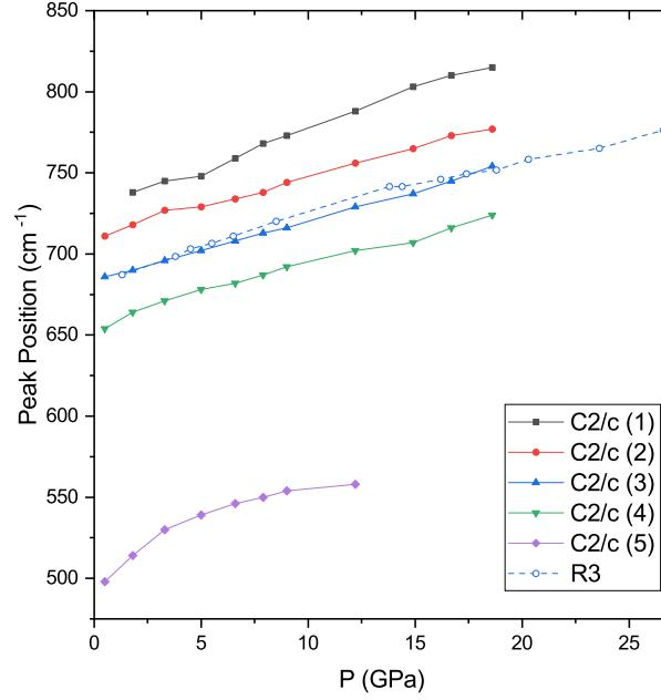
FIG. S5: The pressure dependence of the phonon frequencies of Raman spectrum of  $\text{Co}_3\text{TeO}_6$  in  $C2/c$  and  $R3$  phases, obtained from Fig.6 in main text. The frequencies of five highest peaks of  $C2/c$  are shown.
