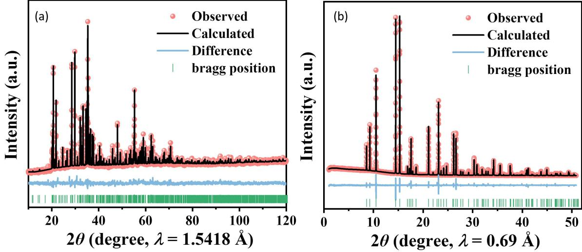
FIG. S1: Refinement of the (a) PXD data of  $\text{Co}_3\text{TeO}_6$  in  $C2/c$  and (b) SPXD data of  $\text{Co}_3\text{TeO}_6$  in  $R3$  (obtained at 5 GPa 1073 K), respectively. The experimental, calculated, difference curves, and Bragg-reflection positions are shown in red, black, blue and green, respectively.
