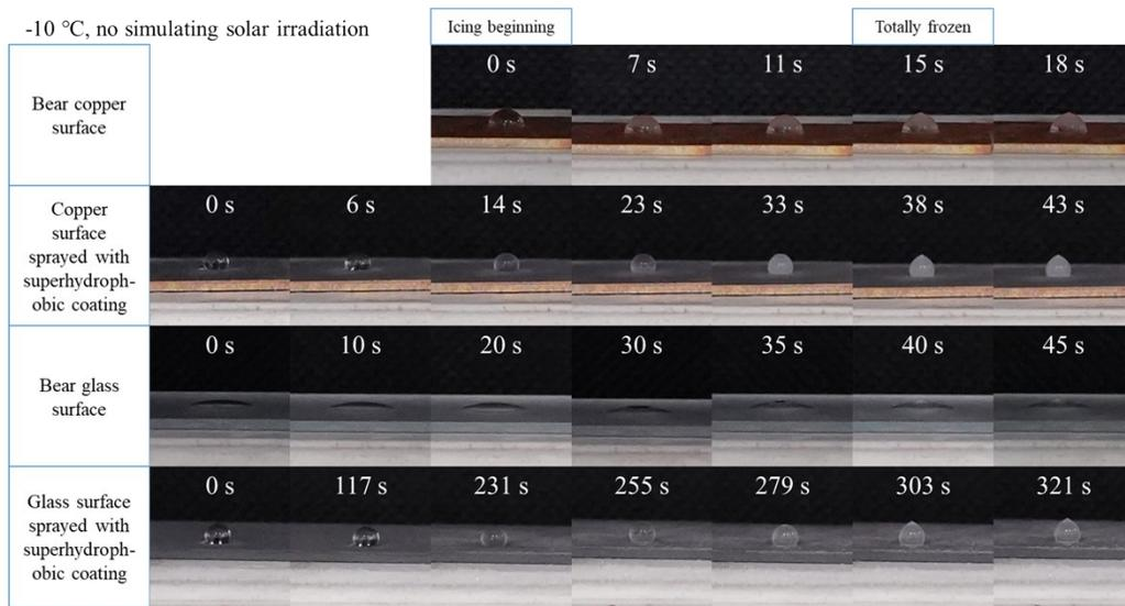
**Fig.S3** The freezing time of four surfaces under the temperature of -10 °C, relative humidity of 40%, without illumination.
