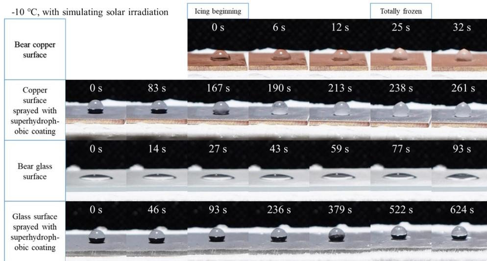
**Fig.S5** The freezing time of four surfaces under the temperature of -10 °C, relative humidity of 40%, with illumination.
