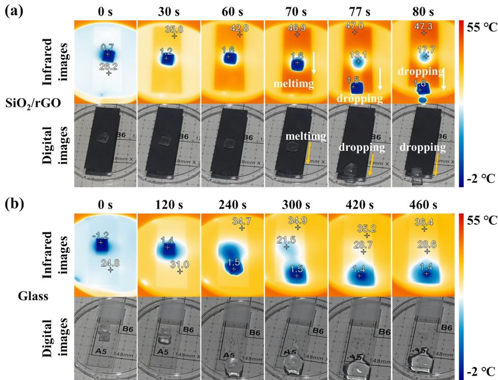
**Fig. S7** Deicing performance of the (a) SiO<sub>2</sub>/rGO composite coating and (b) glass surface under simulated sunlight (900 W/m<sup>2</sup>), with ice cube dimensions of 0.8 × 0.8 × 0.8 cm<sup>3</sup> (0.512 mL).
