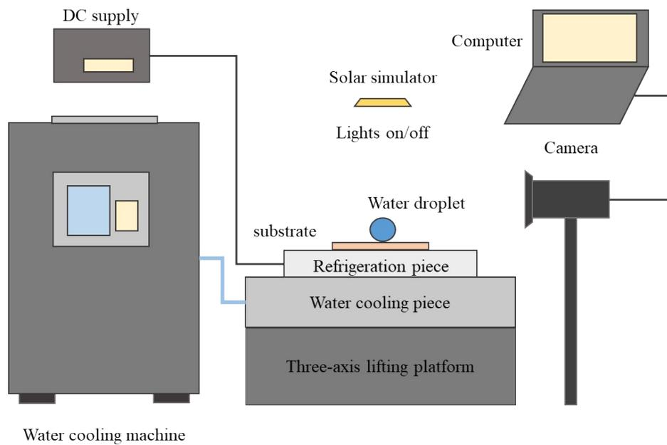
**Fig.S1** Schematic diagram of the icing-delay test system.
