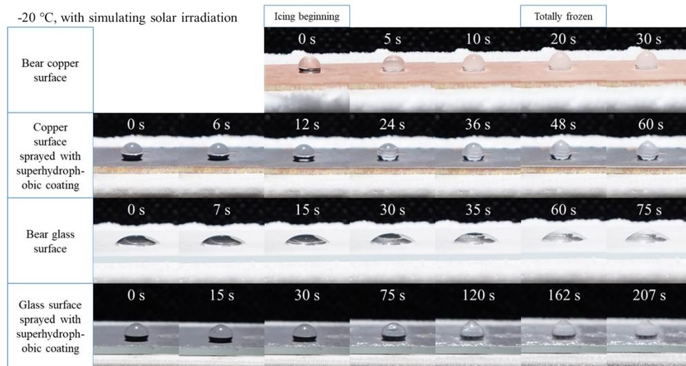
**Fig.S6** The freezing time of four surfaces under the temperature of -20 °C, relative humidity of 40%, with illumination.
