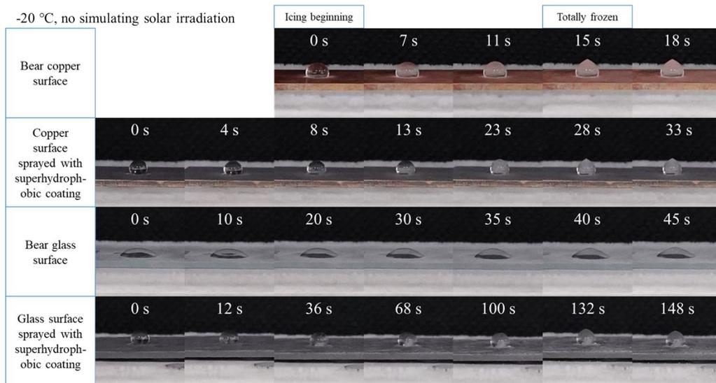
**Fig.S4** The freezing time of four surfaces under the temperature of -20 °C, relative humidity of 40%, without illumination.
