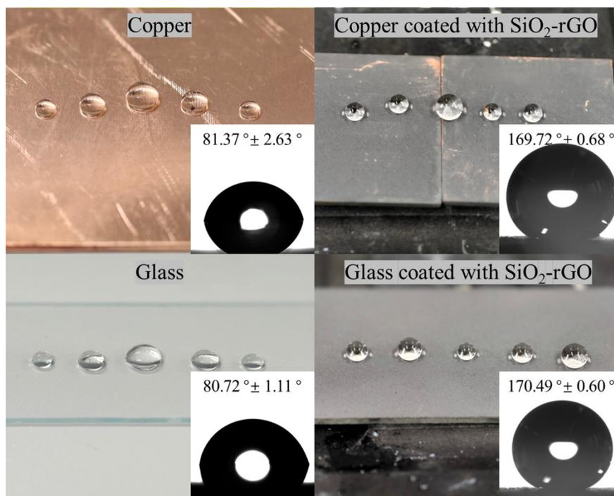
**Fig.S2** Water contact angles (WCAs) of copper, copper coated with  $\text{SiO}_2/\text{rGO}$ , glass and glass coated with  $\text{SiO}_2/\text{rGO}$ .
