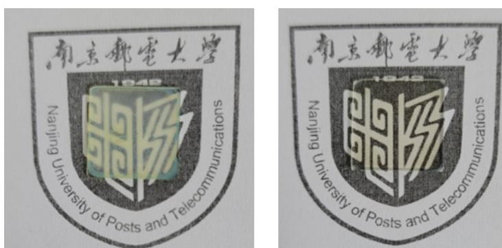
Figure S44. Light transmittance photographs of PChDPF in drop-casting (left) and solvent-casting (right) states.
