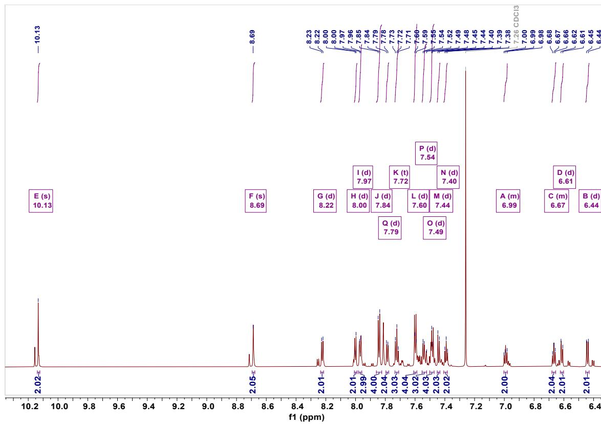
**Figure S8.**  $^1\text{H}$  NMR spectrum of intermediate SAFCz-CHO (solvent: Chloroform-*d*).
