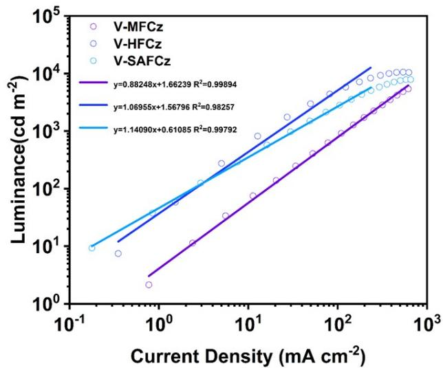
**Figure S34.** Luminance versus current density and the fitted curve plots.
