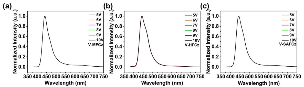
**Figure S35.** (a) EL spectra of V-MFCz, (b) V-HFCz, and (c) V-SAFCz at different voltages.
