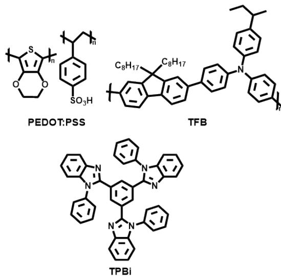
**Figure S33.** Chemical structures of the materials used for the non-doped deep-blue OLED devices.
