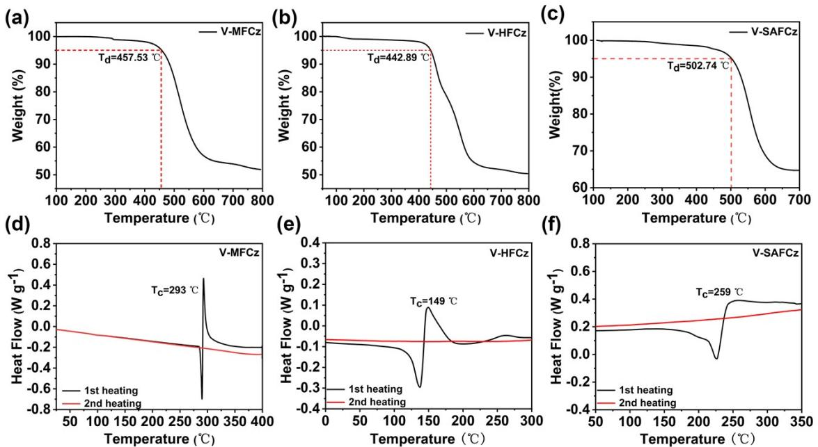
**Figure S29.** (a) TGA curves of V-MFCz (b) V-HFCz (c) V-SAFCz; (d) DSC curves of V-MFCz (e) V-HFCz and (f) V-SAFCz.
