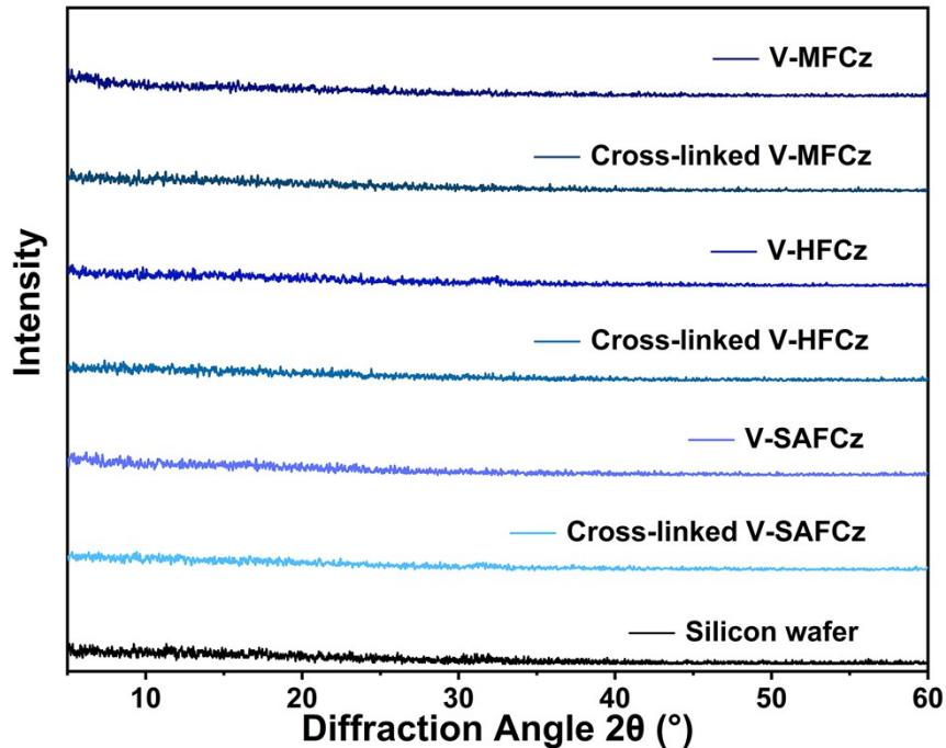
**Figure S31.** XRD patterns of V-MFCz, V-HFCz, and V-SAFCz films before and after cross-linking.
