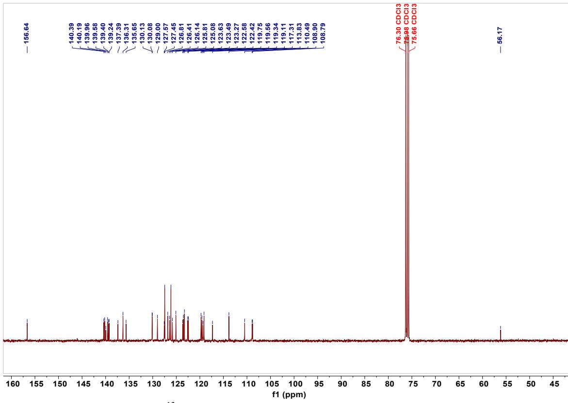
**Figure S17.**  $^{13}\text{C}$  NMR spectrum of V-SAFCz (solvent: Chloroform-*d*).
