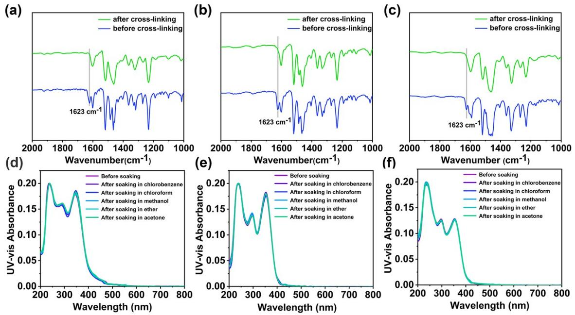
**Figure S30** (a) FTIR spectra of V-MFCz (b) V-HFCz (c) V-SAFCz before and after cross-linking; (d) The solvent resistance of V-MFCz (e) V-HFCz (f) V-SAFCz cross-linked films in different solvents.
