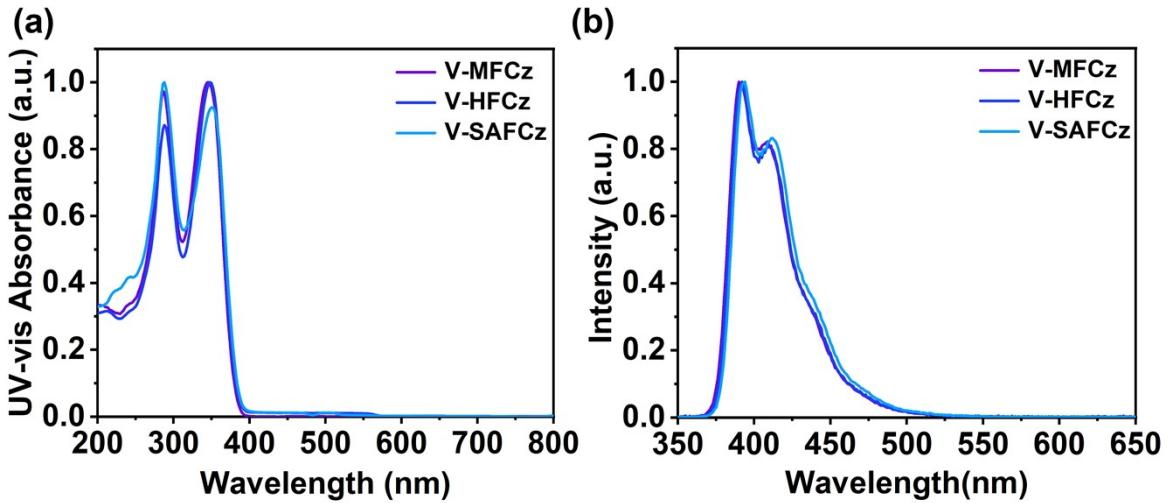
**Figure S27.** The UV-vis absorption and fluorescence spectra of V-MFCz, V-HFCz, and V-SAFCz in toluene solution.
