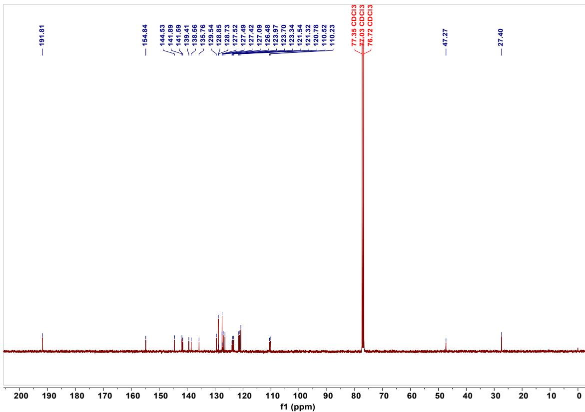
**Figure S11.**  $^{13}\text{C}$  NMR spectrum of intermediate MFCz-CHO (solvent: Chloroform-*d*).
