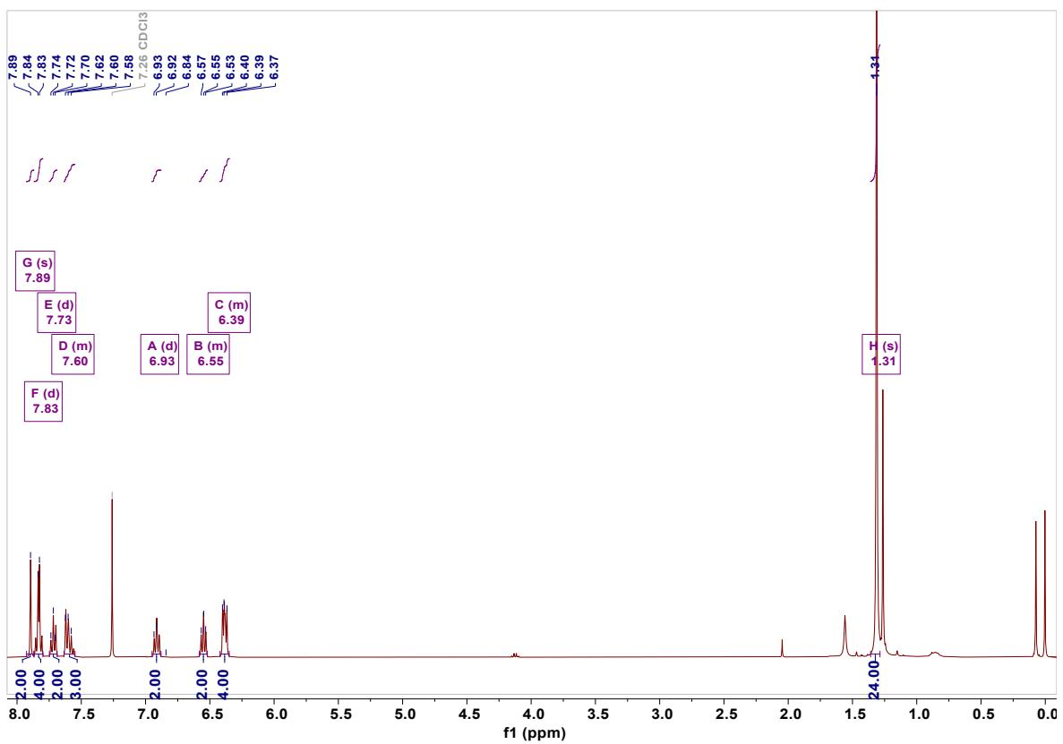
**Figure S7.**  $^1\text{H}$  NMR spectrum of intermediate SAF-Bpin (solvent: Chloroform-*d*).
