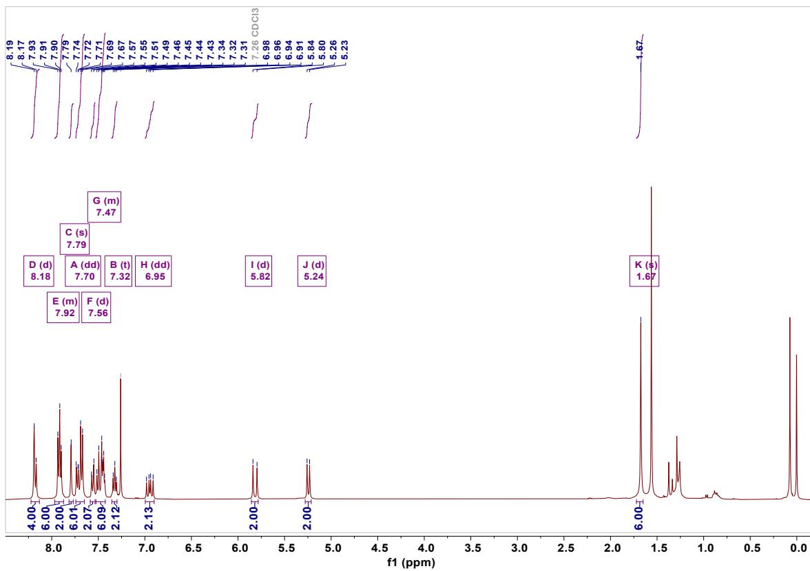
**Figure S3.**  $^1\text{H}$  NMR spectrum of V-MFCz (solvent: Chloroform- $d$ ).
