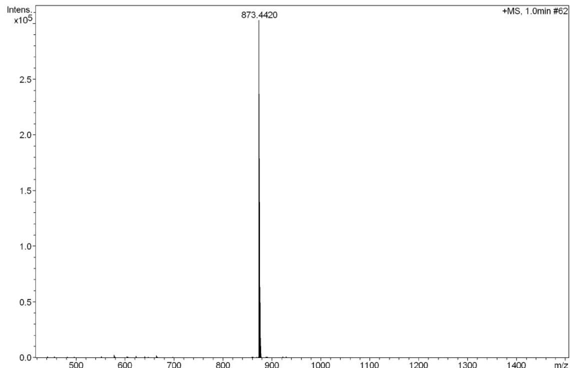
**Figure S21.** The HRMS spectrum of the intermediate HFCz-CHO.
