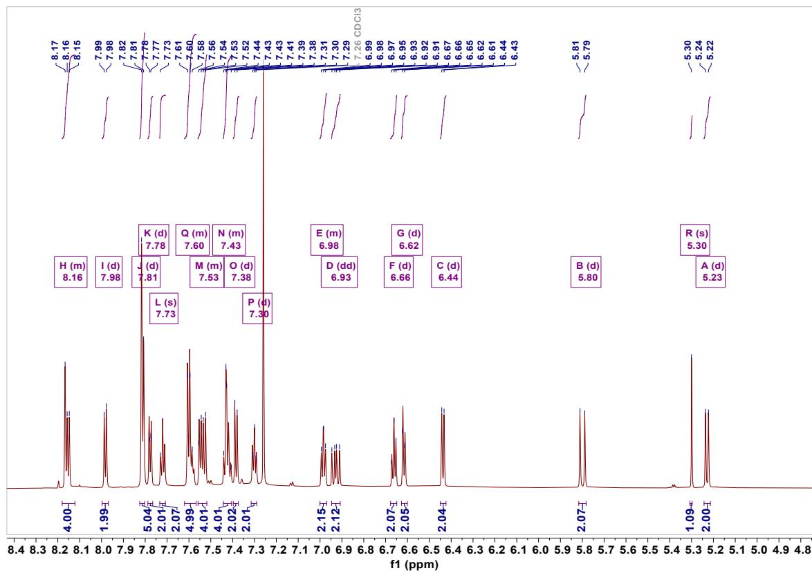
**Figure S9.**  $^1\text{H}$  NMR spectrum of V-SAFCz (solvent: Chloroform-*d*).
