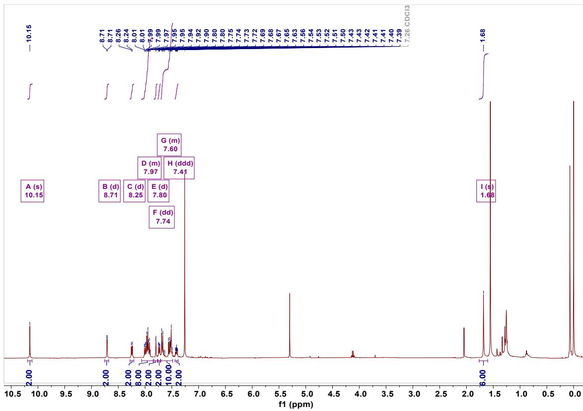
**Figure S2.**  $^1\text{H}$  NMR spectrum of intermediate MFCz-CHO (solvent: Chloroform- $d$ ).
