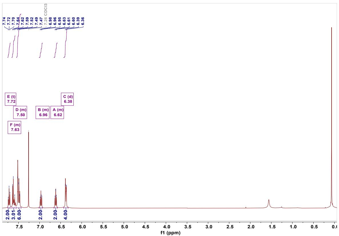
**Figure S6.**  $^1\text{H}$  NMR spectrum of intermediate SAF-Br (solvent: Chloroform-*d*).
