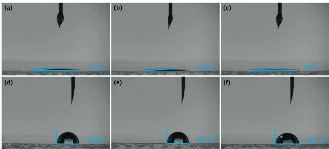
**Figure S32.** (a) Contact angles of V-MFCz, (b) V-HFCz, (c) V-SAFCz cross-linked films with toluene; (d) The contact angle between V-MFCz, (e) V-HFCz, (f) V-SAFCz cross-linked films and water.
