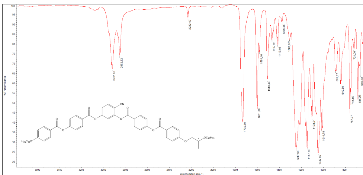
Figure S39. FT-IR spectrum of 4-{4-[4-( n -Dodecyloxy)benzoyloxy]benzoyloxy}-2-{4-[4-(( S )-2- n -dodecyloxypropoxy)benzoyloxy]benzoyloxy} benzonitrile ( IIc ).
