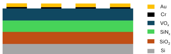
Figure S1: The architecture of VO x films deposited on Si/SiO 2 /SiN x substrate.
