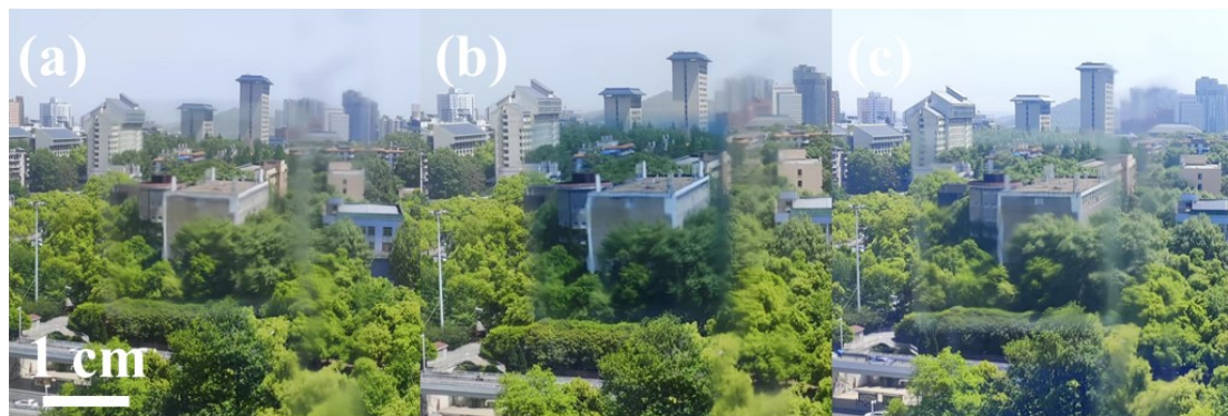
Figure S9. The photographs of MoO 3 /PVP composite film at initial (a), tinted (b) and bleached state (c).
