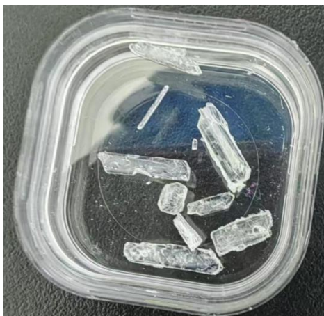
Figure S3. Transparent millimeter-sized \text{TEA}_2\text{Cu}_2\text{Br}_4 single crystals obtained by slow solvent evaporation under ambient conditions (22–25 °C, 45–55% RH) over approximately 48–60 h.
