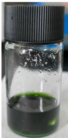
Figure S1. Preparation of the \text{TEA}_2\text{Cu}_2\text{Br}_4 precursor solution by dissolving 2 mmol TEABr and 2 mmol CuBr in 10 mL acetone. The solution was filtered through a 0.45 \mu\text{m} PVDF membrane before crystallization.
