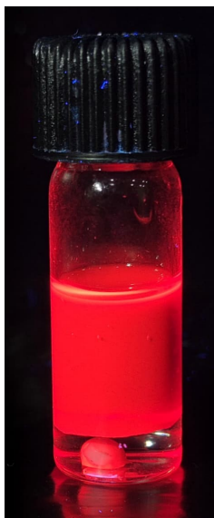
Figure S3. Typical photograph under UV light showing the formation of a biphasic system upon dispersing CuInS 2 quantum dots in toluene and introducing methanol and trioctylphosphine (TOP) as a polar phase along with the metal salt.
