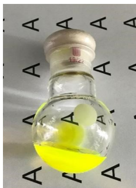
Figure S22. Photograph of the flask after blue light (445 nm)-driven polymerization.
