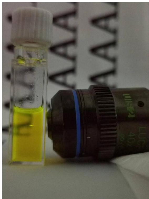
Figure S29. TTA-UC photographed in Ar-saturated ethylene glycol dimethacrylate/trimethylolpropane ethoxylate triacrylate (1/1, v/v). c(\text{PtTNP}) = 5 \mu\text{M} , c(\text{An-3}) = 0.5 \text{ mM} , \lambda_{\text{ex}} = 721 \text{ nm} .
