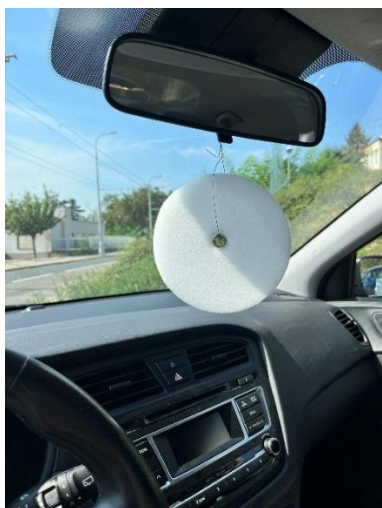
Figure S2 Polyurethane (PUF) disk used as passive sampler
