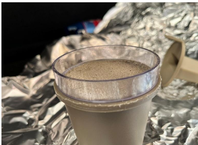
Figure S3 Dust sampling head and quartz microfiber filter containing vehicle dust sample
