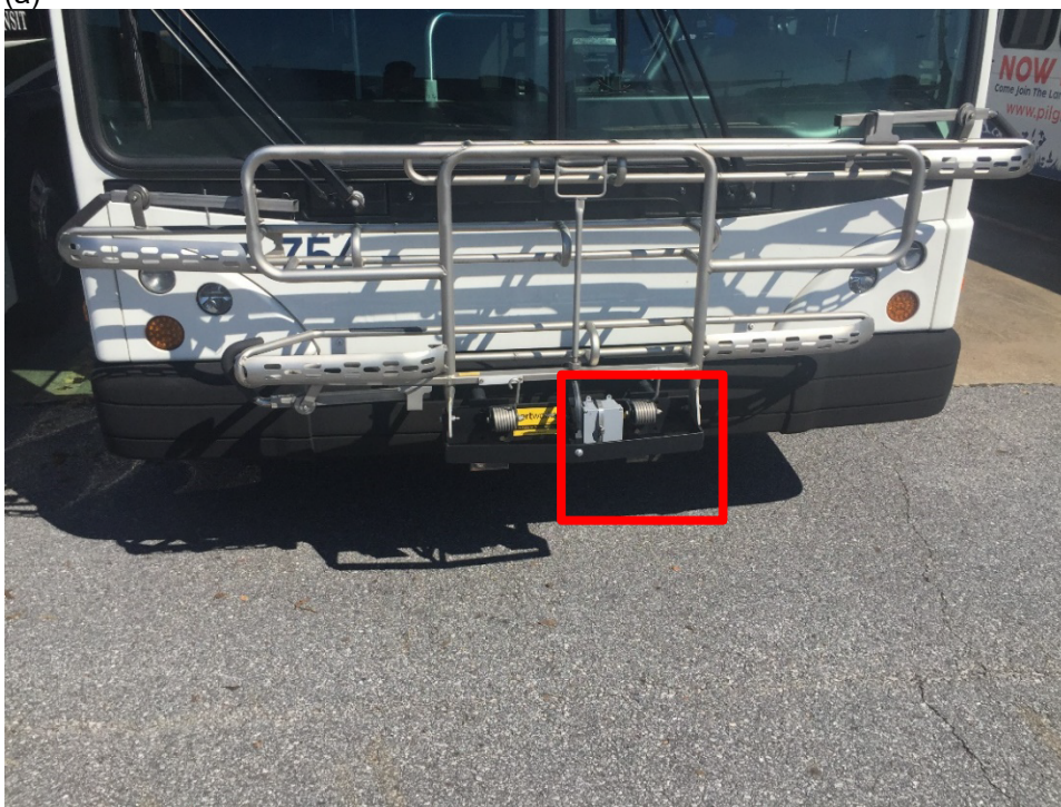
Fig. S1 Data collection related images, (1a) Map of all bus routes from Athens and UGA Transit (Colors represent different bus routes), (1b) Sensor on bus bike rack
