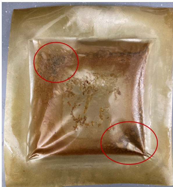
Figure S2-11. Photo of bipolar membrane after use during BPED experiment. Two example areas showing blistering and delamination are circled in red.
