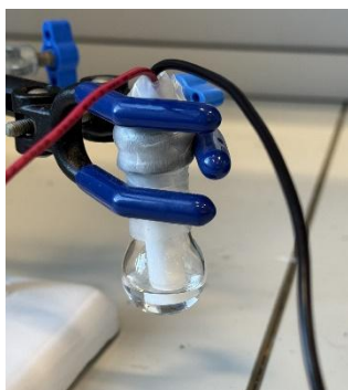
Figure S2 Two-electrode platinum cell designed to perform ionic conductivity measurements.
