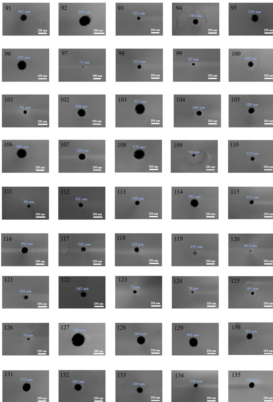
Figure S1 SEM morphology images (cross-section) of the 135 Nanopipettes samples used for training the ANN model. The numbers in each figure correspond to the serial numbers in Table S1.
