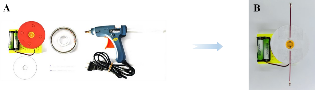
Figure S3. Photograph of centrifuge assembly components. (A) Photographs of all centrifugation device components: DIY centrifuge, medical tape, two 1.5V alkaline batteries in series, double-sided tape, a hot glue gun, two capillary tubes, and a circular sheet of plain paper. (B) A top view of the constructed centrifugal device.
