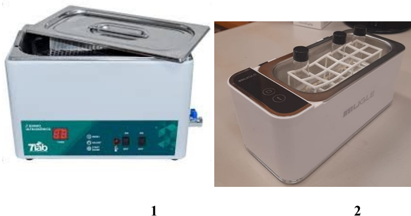
28 Figure S1. Photographs of the ultrasonic baths used in the sample preparation experiments: 29 (1) ultrasonic bath 1 (USC-1400, UNIQUE); (2) ultrasonic bath 2 (YT-80 ultrasonic cleaner).
