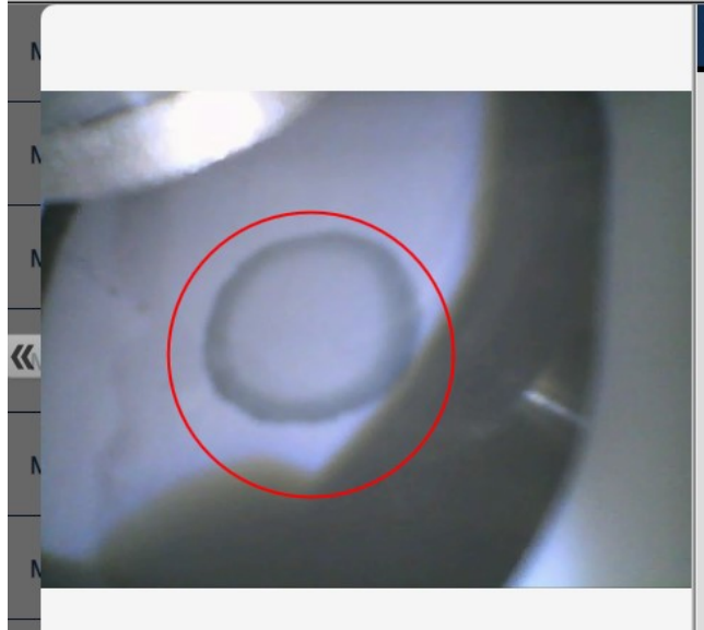
Figure S-2 Internal camera view from the software used to operate the portable XRF analyzer. The XRF beam diameter is approximately 8 mm. The filter is spiked with 3 µL solution containing 45 µg of Cr. The mass density is assumed to be 89.46 µg cm 2 , based on the X-ray beam illumination area (0.503 cm 2 ).
