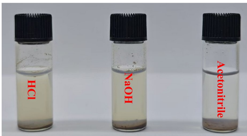
Fig. S1. The stability of \text{NH}_2\text{-UiO-66} after treatment with water, 0.1 M HCl, and 0.1 M NaOH for 24 h.
