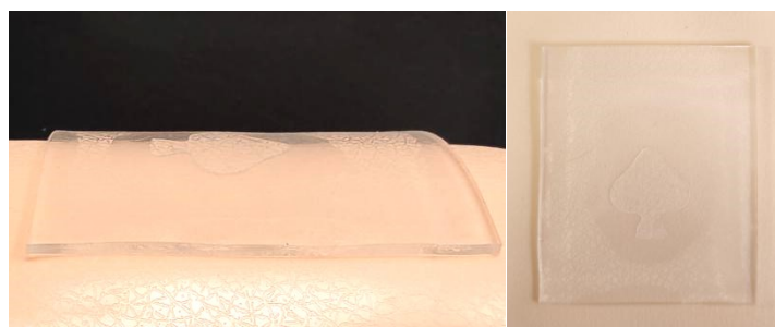
Figure S1: Photographs of the flexible PDMS waveguide.
