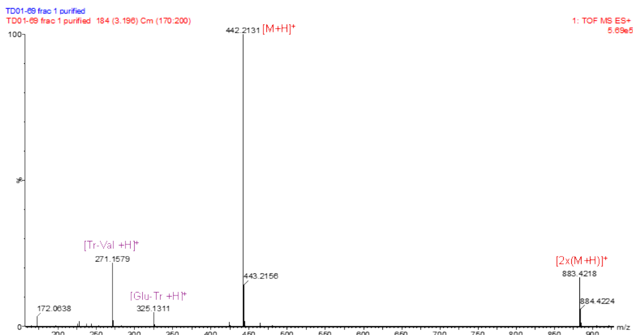
Figure S20. HR-ESI mass spectrum of peptide Ac-ETrv-OH. Observed fragmentation products also identified.
